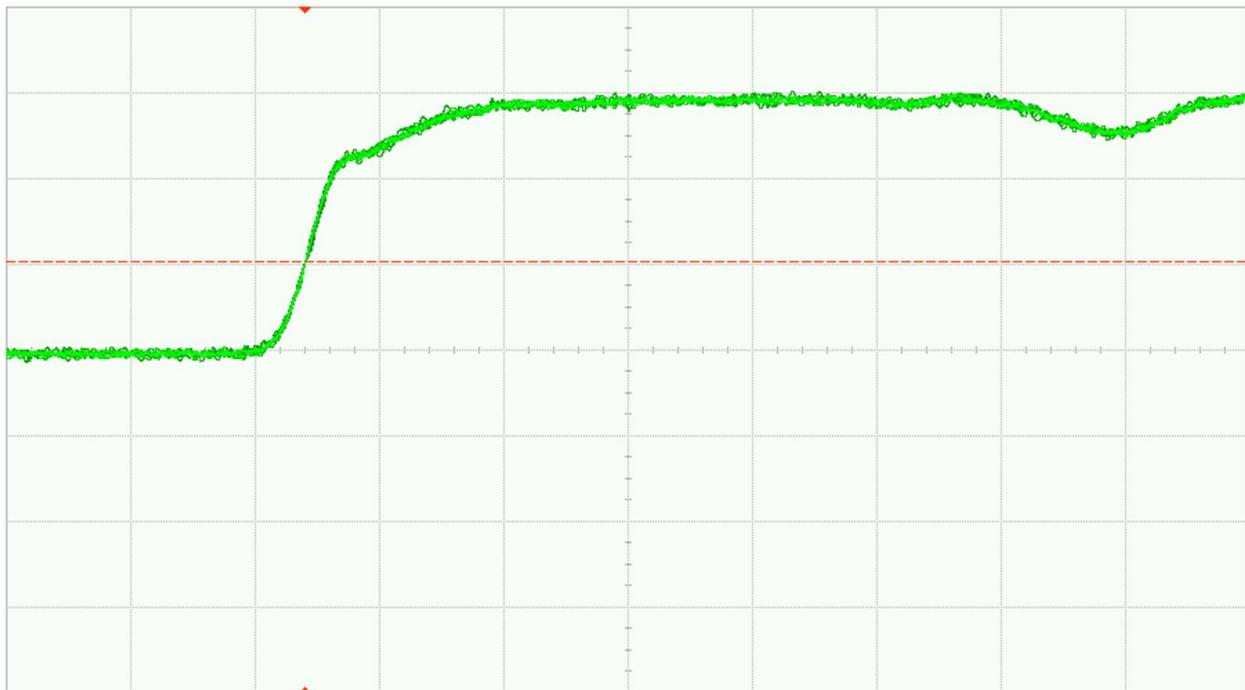
Fig. 27 (a). DUT 15737 pre-irradiation rising edge, abscissa scale is 1V/div and ordinate scale is 2ns/div
