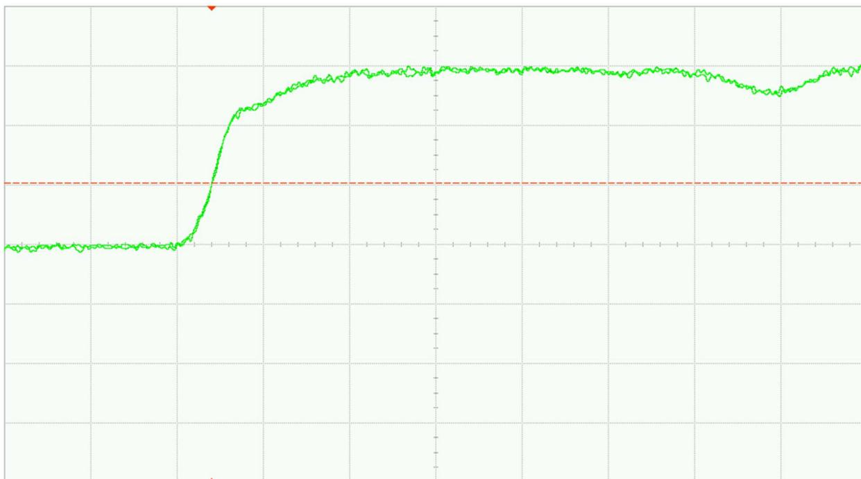
Fig. 28 (a). DUT 15745 pre-irradiation rising edge, abscissa scale is 1V/div and ordinate scale is 2ns/div
