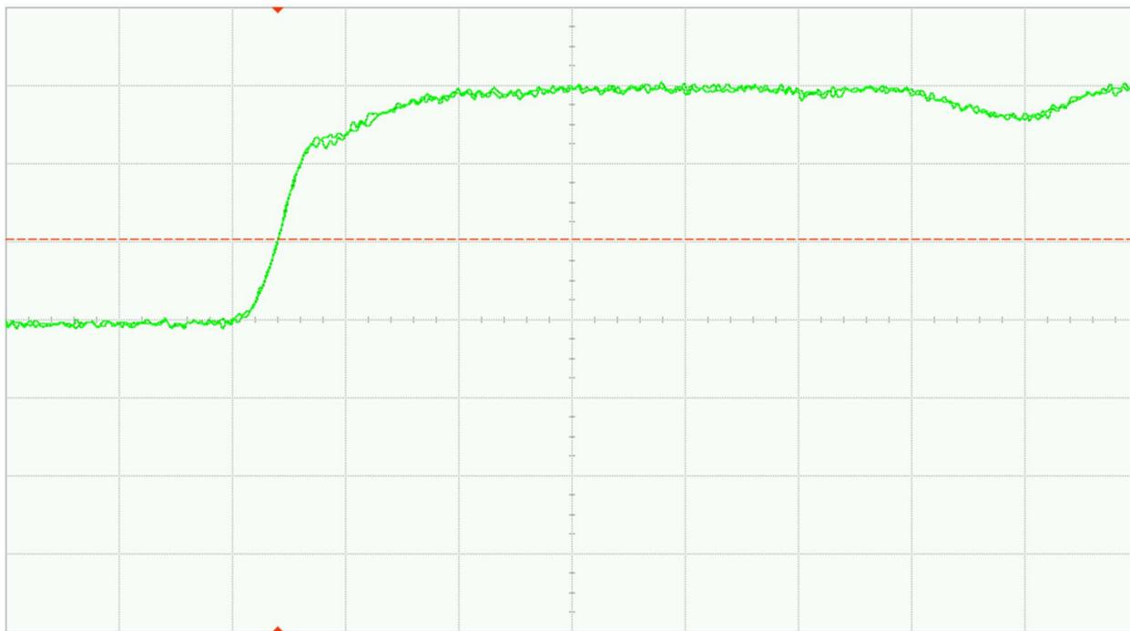
Fig. 30 (b). DUT 15750 post-annealing rising edge, abscissa scale is 1V/div and ordinate scale is 2ns/div
