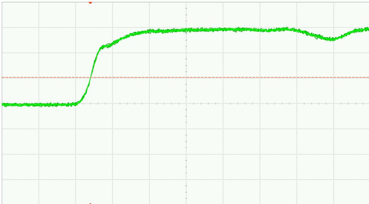
Fig. 30 (a). DUT 15750 pre-irradiation rising edge, abscissa scale is 1V/div and ordinate scale is 2ns/div
