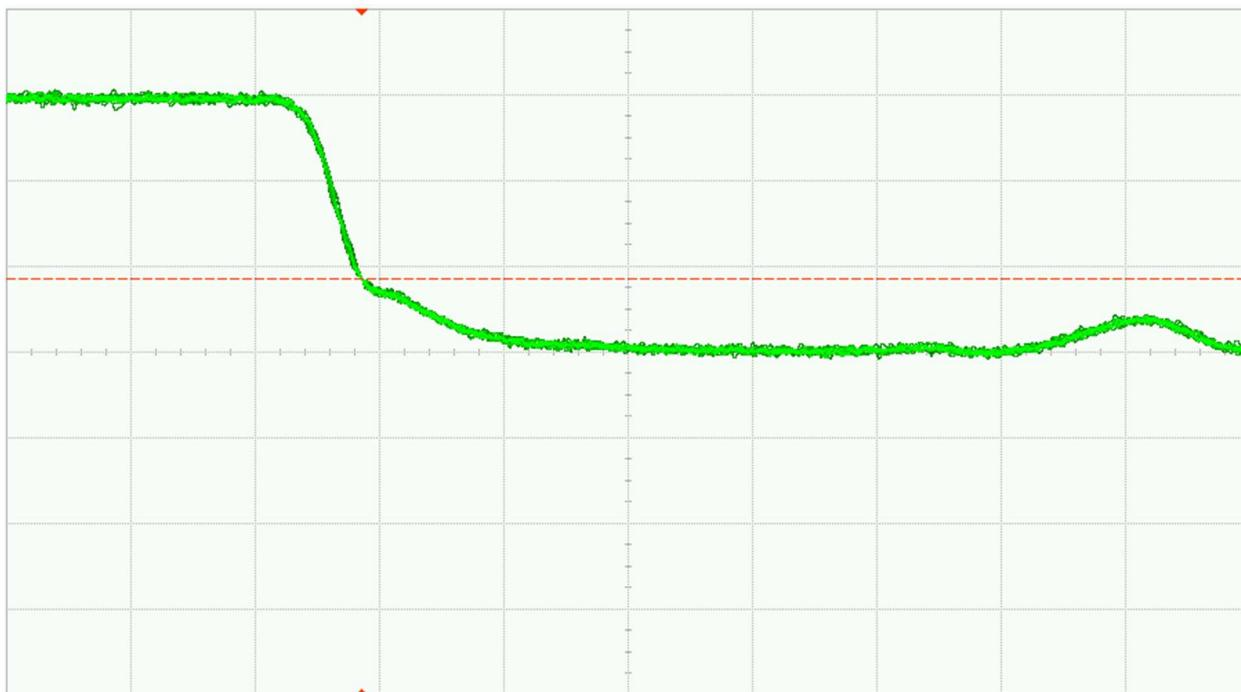
Fig. 35 (a). DUT 15749 pre-irradiation falling edge, abscissa scale is 1V/div and ordinate scale is 2ns/div
