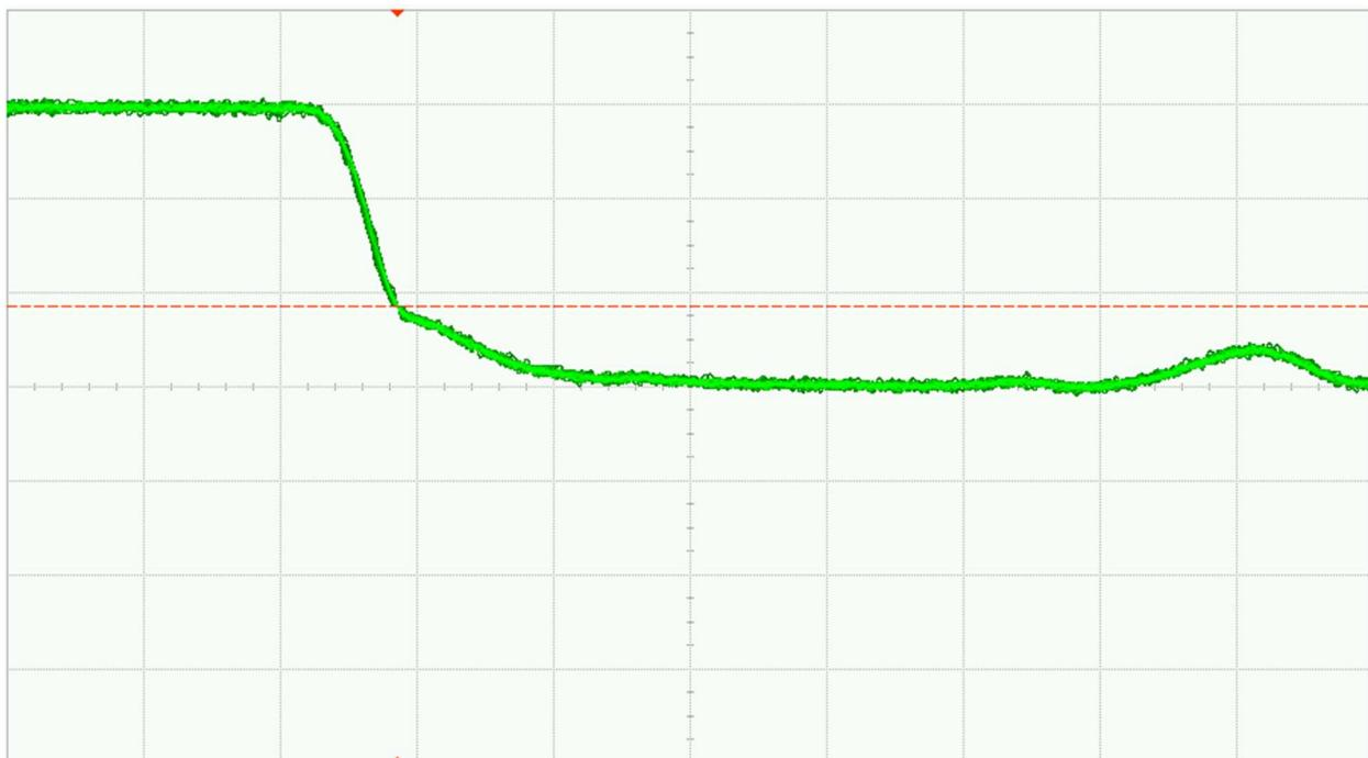
Fig. 36 (a). DUT 15750 pre-irradiation falling edge, abscissa scale is 1V/div and ordinate scale is 2ns/div
