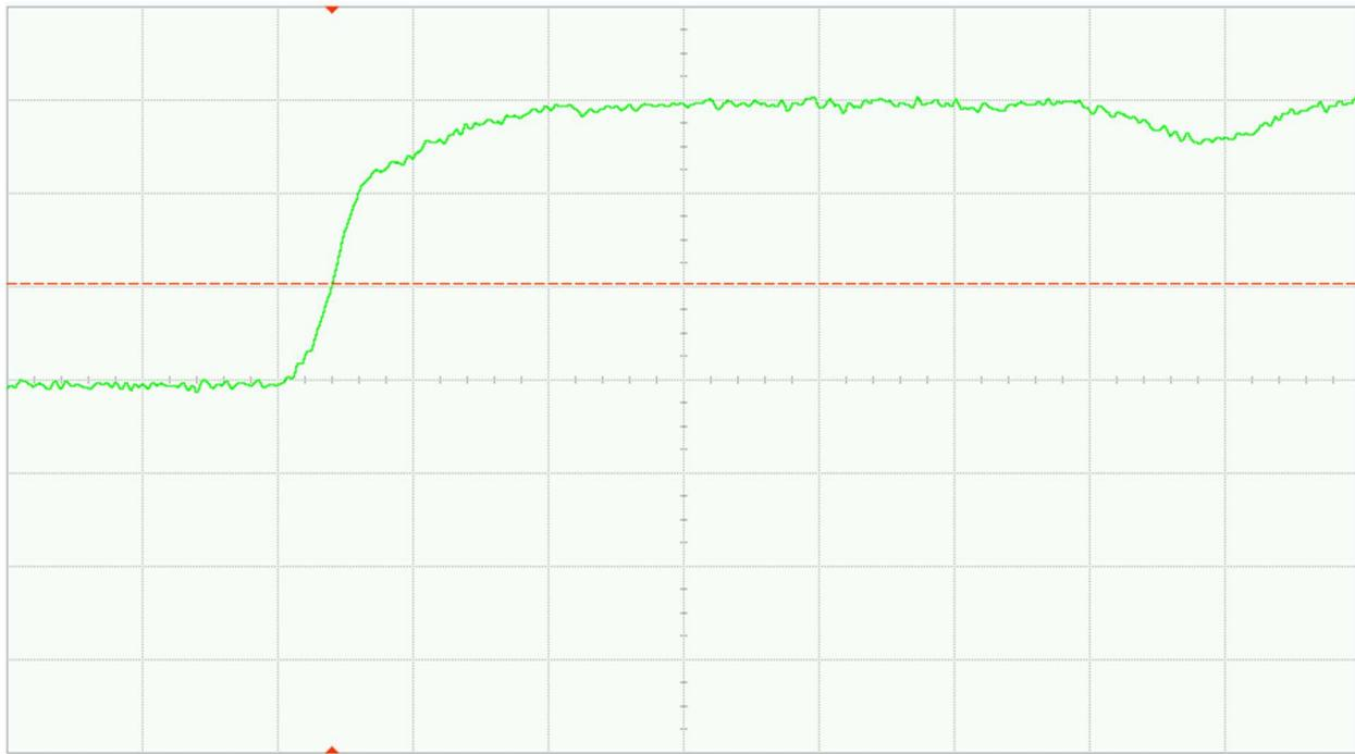
Fig. 29 (b). DUT 15749 post-annealing rising edge, abscissa scale is 1V/div and ordinate scale is 2ns/div
