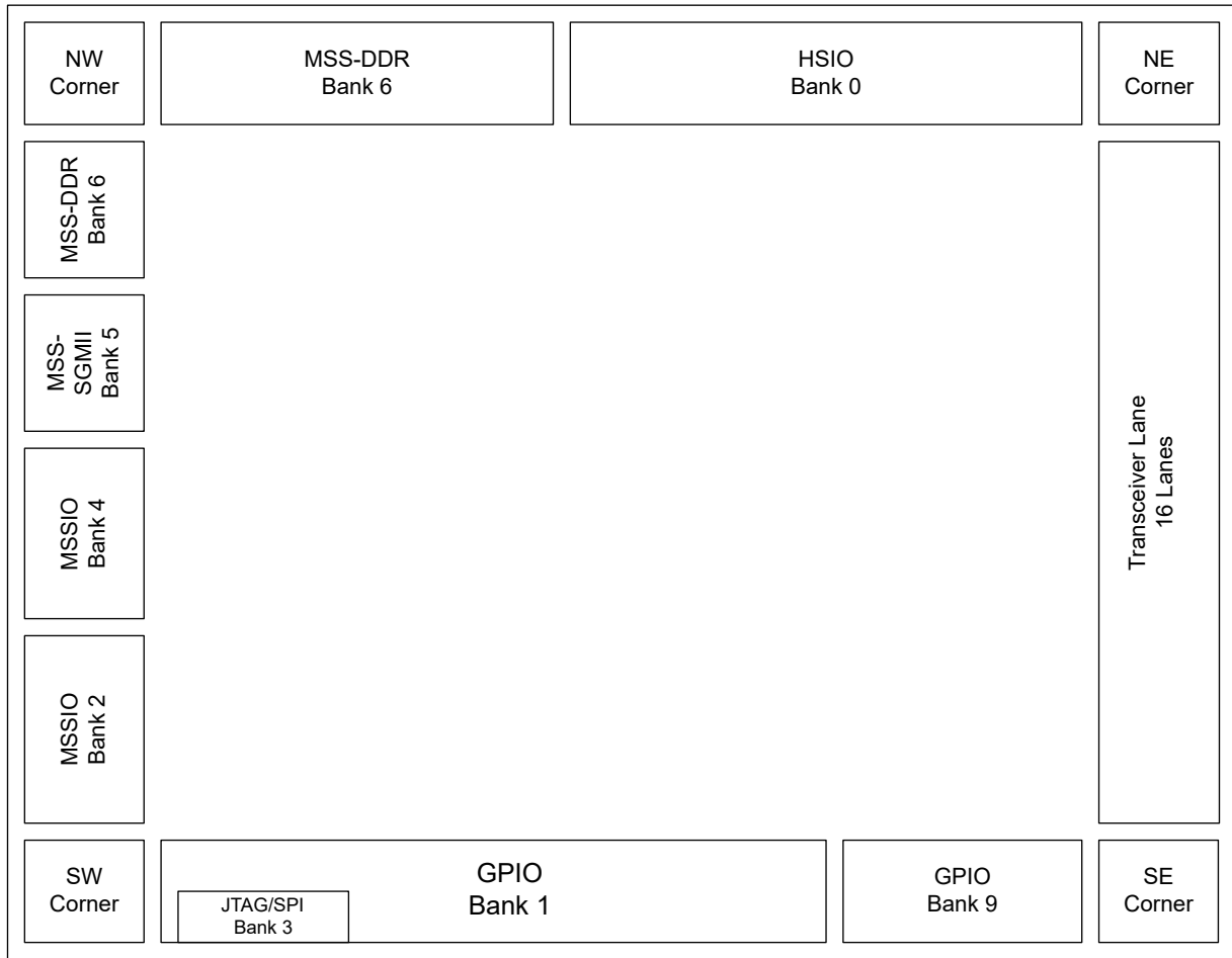
Figure 3-4. PolarFire SoC FPGA MPFS250–FCG1152 I/O Banks
