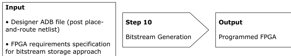
Figure 15 • V-Model Development Step 10—Bitstream Generation
