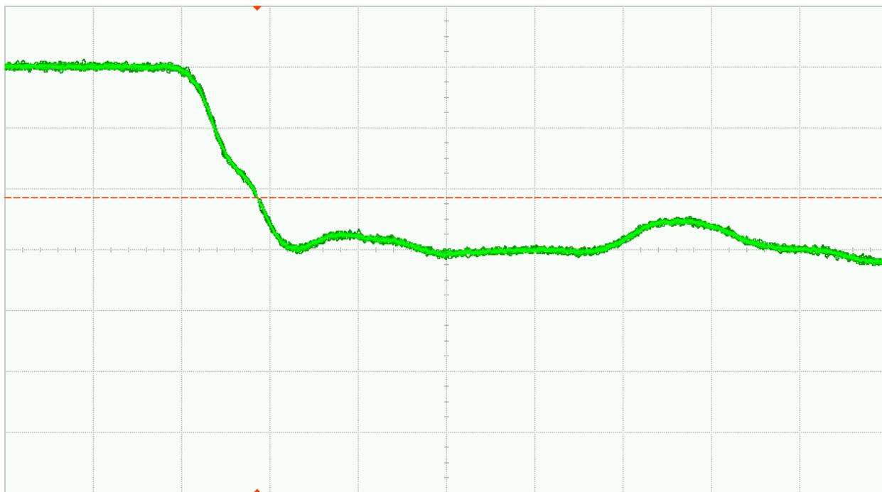
Fig. 36 (a). DUT 05216 pre-irradiation falling edge, abscissa scale is 1V/div and ordinate scale is 2ns/div
