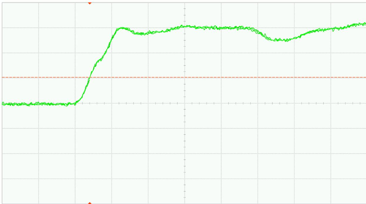
Fig. 31 (b). DUT 05220 post-annealing rising edge, abscissa scale is 1V/div and ordinate scale is 2ns/div
