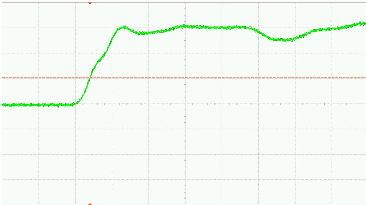
Fig. 29 (b). DUT 05178 post-annealing rising edge, abscissa scale is 1V/div and ordinate scale is 2ns/div
