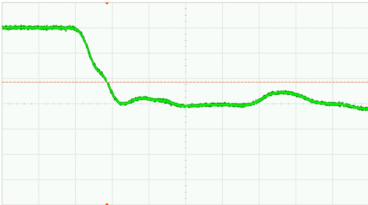
Fig. 34 (a). DUT 05169 pre-irradiation falling edge, abscissa scale is 1V/div and ordinate scale is 2ns/div
