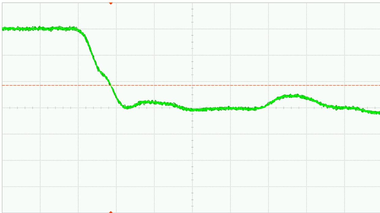
Fig. 33 (a). DUT 05165 pre-irradiation falling edge, abscissa scale is 1V/div and ordinate scale is 2ns/div
