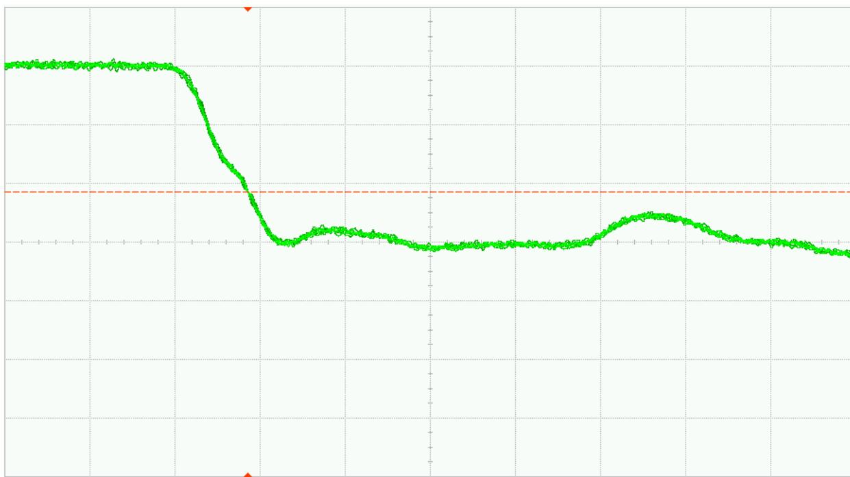
Fig. 35 (a). DUT 05178 pre-irradiation falling edge, abscissa scale is 1V/div and ordinate scale is 2ns/div
