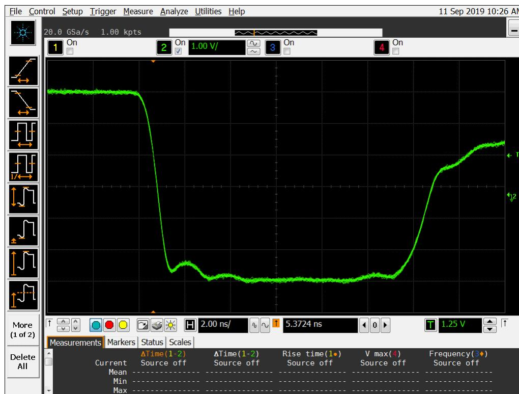
**Figure 15a DUT 6217 Pre-Radiation Falling Edge**
