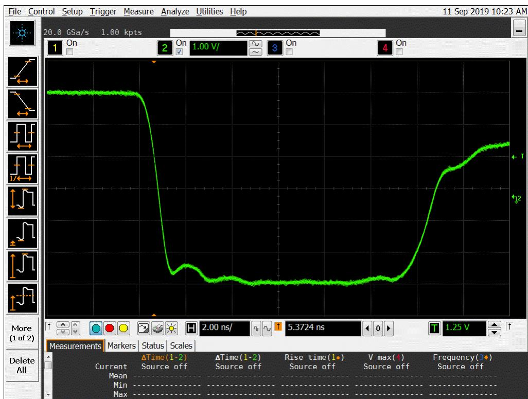
**Figure 18a DUT 6201 Pre-Irradiation Falling Edge**
