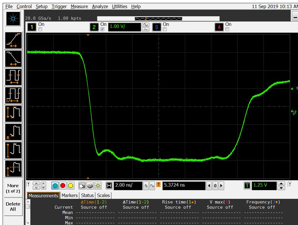
**Figure 19a DUT 6176 Pre-Irradiation Falling Edge**
