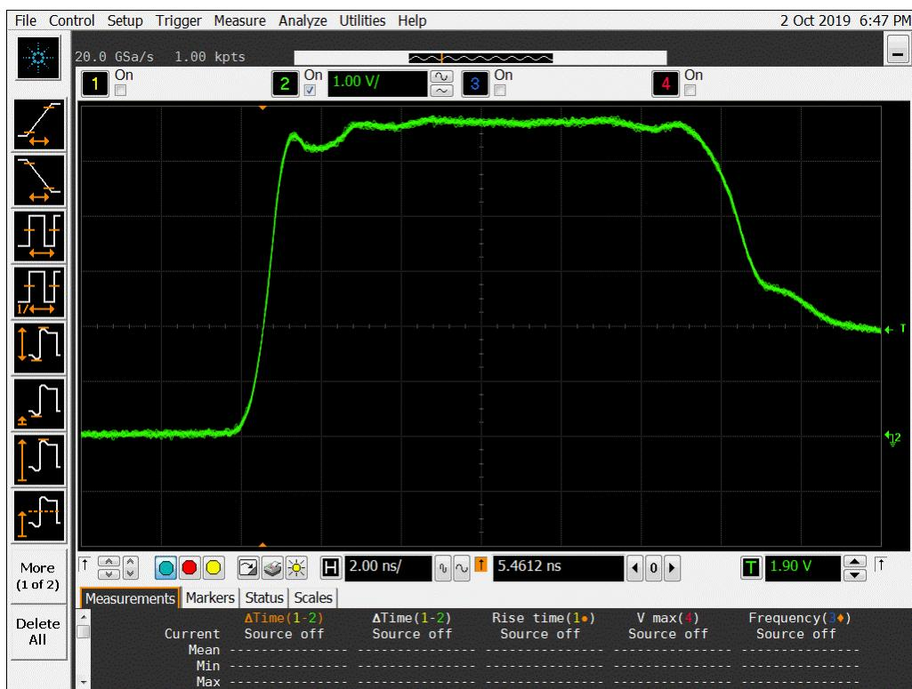
**Figure 10b DUT 6220 Post-Annealing Rising Edge**
