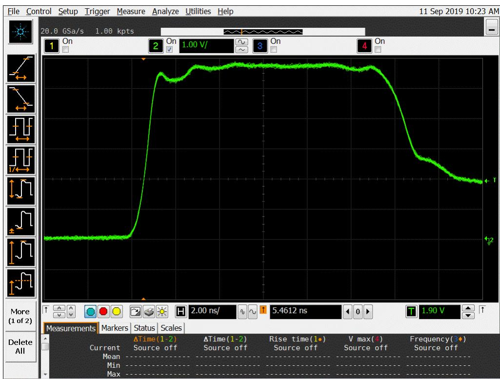
Figure 12a DUT 6201 Pre-Irradiation Rising Edge
