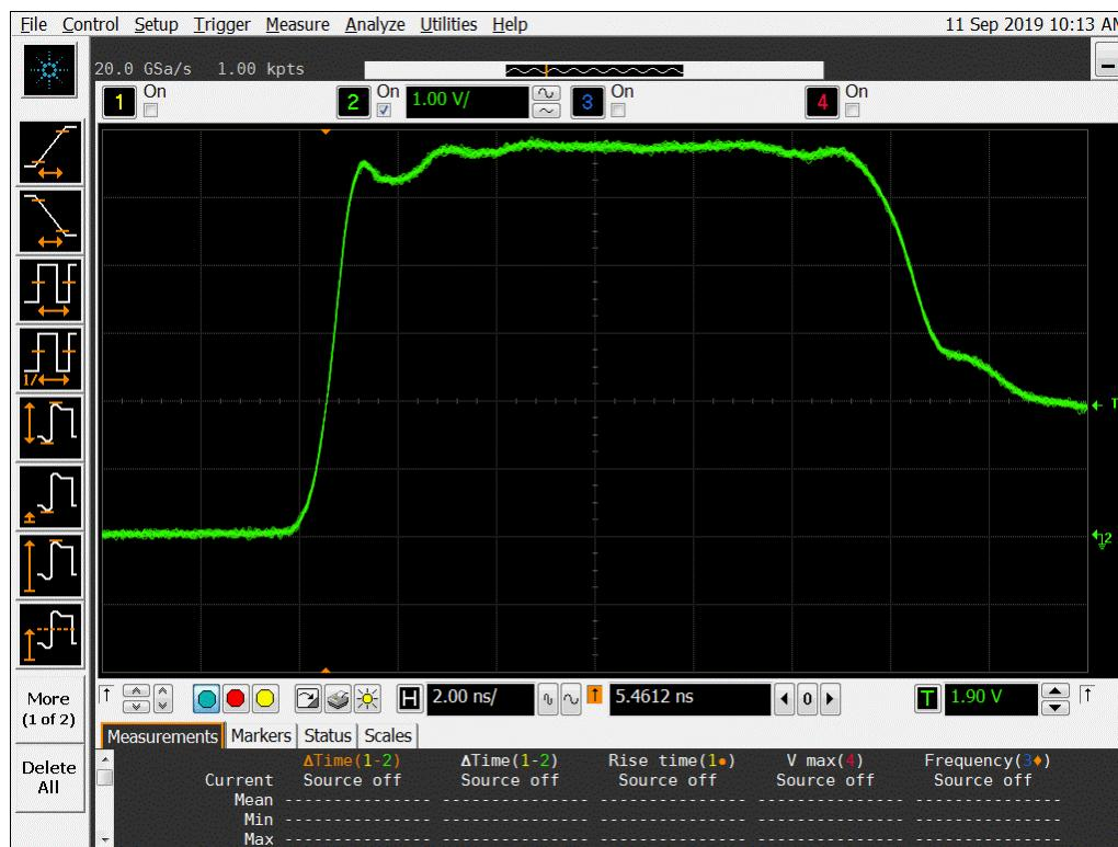
**Figure 13a DUT 6176 Pre-Irradiation Rising Edge**
