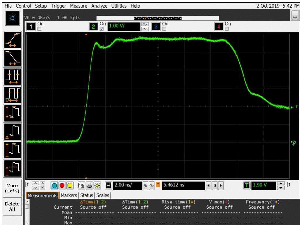
Figure 12b DUT 6201 Post-Annealing Rising Edge
