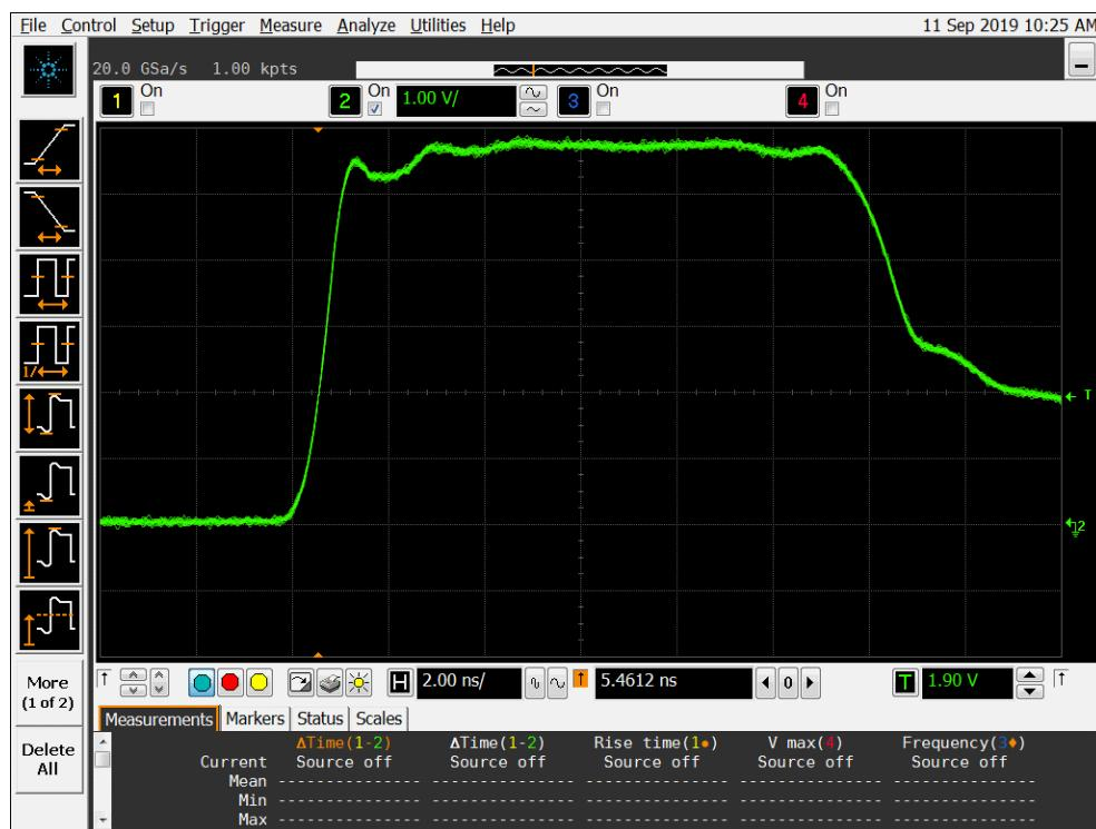
Figure 9a DUT 6217 Pre-Irradiation Rising Edge
