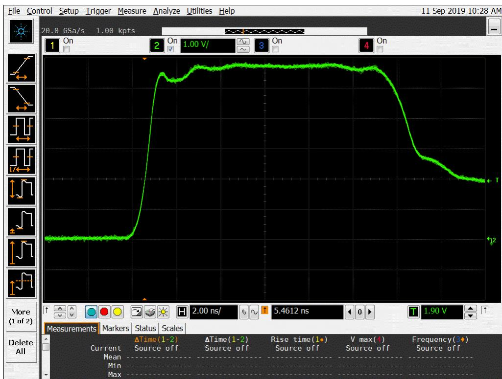
**Figure 10a DUT 6220 Pre-Irradiation Rising Edge**
