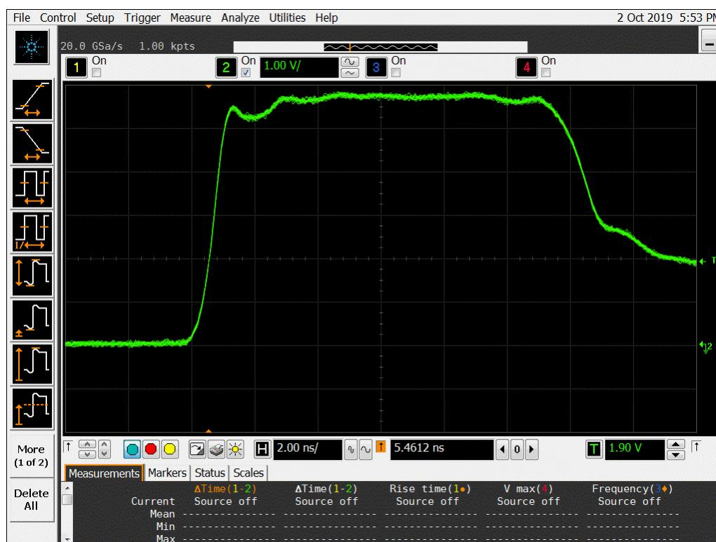
**Figure 13b DUT 6176 Post-Annealing Rising Edge**
