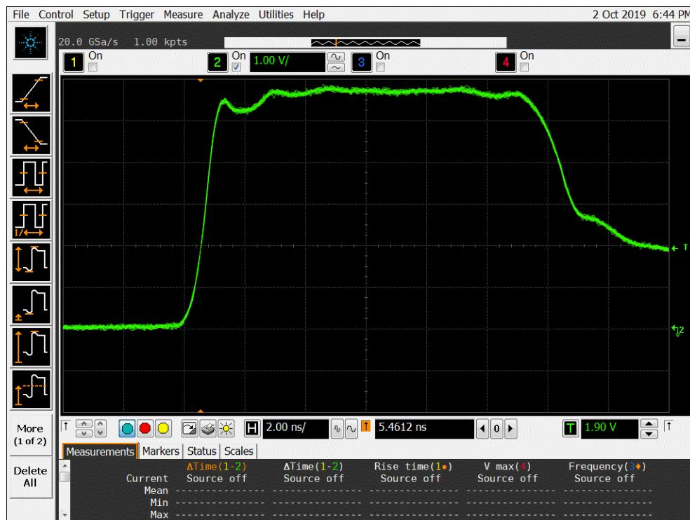
Figure 9b DUT 6217 Post-Annealing Rising Edge
