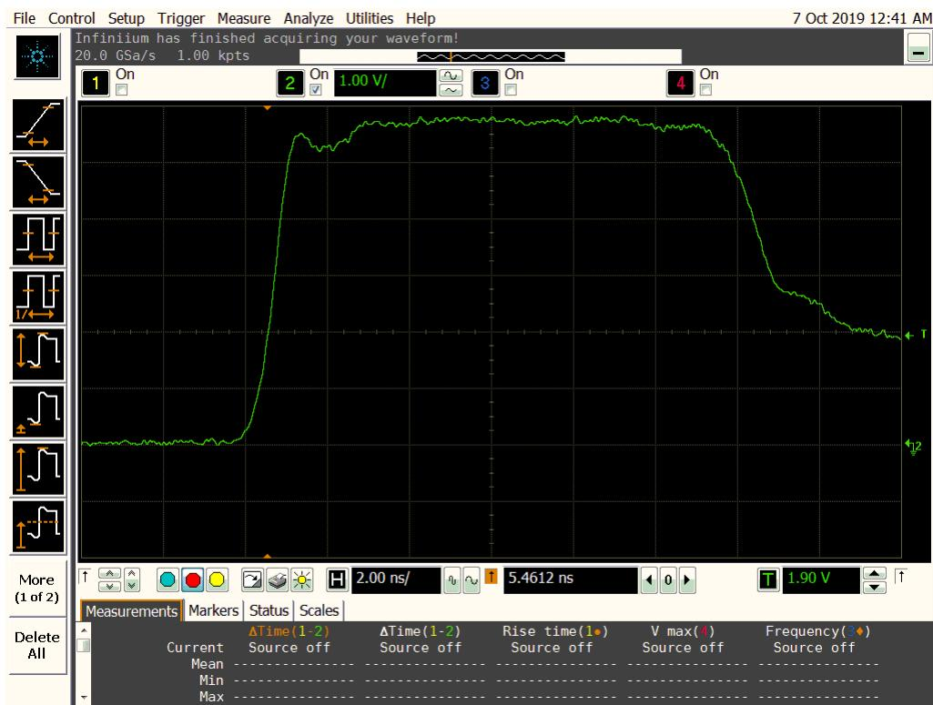
Figure 14b DUT 6180 Post-Annealing Rising Edge
