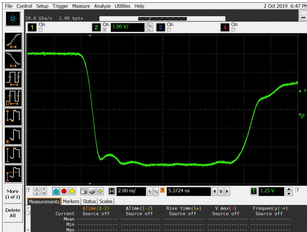
**Figure 16b DUT 6220 Post-Annealing Falling Edge**
