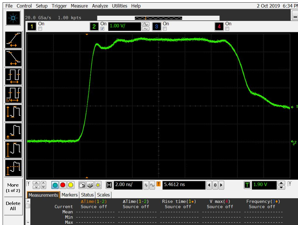
**Figure 11b DUT 6199 Post-Annealing Rising edge**
