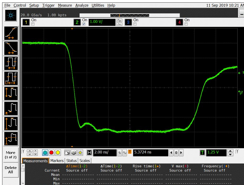
**Figure 17a DUT 6199 Pre-Irradiation Falling Edge**
