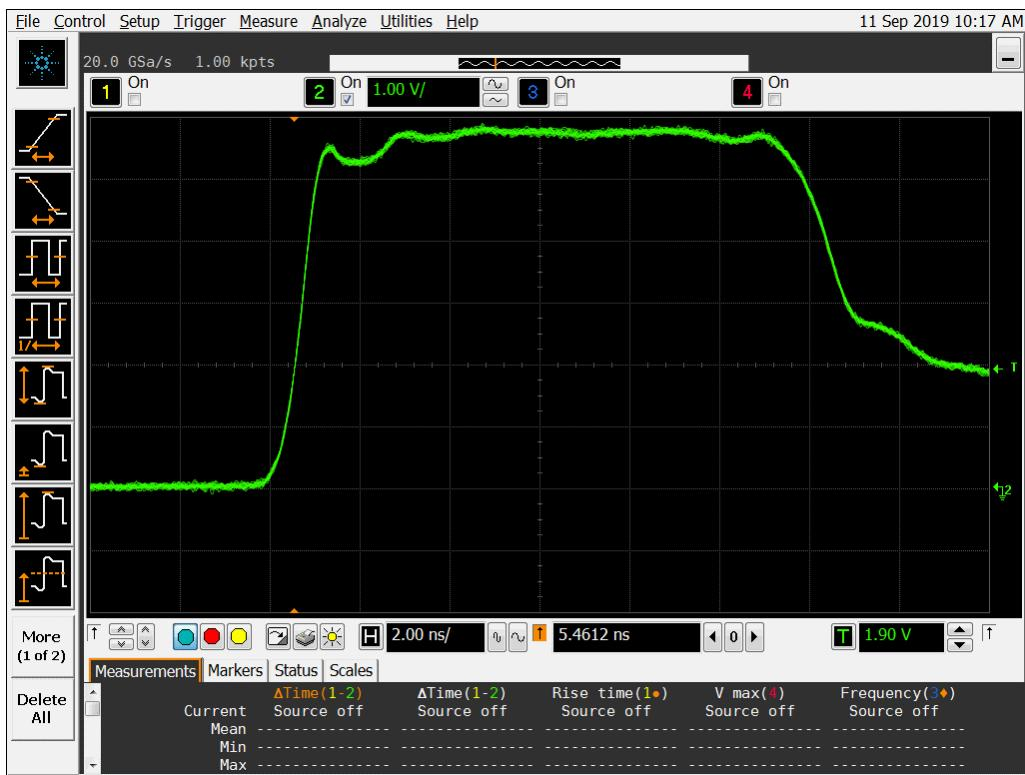
Figure 14a DUT 6180 Pre-Irradiation Rising Edge
