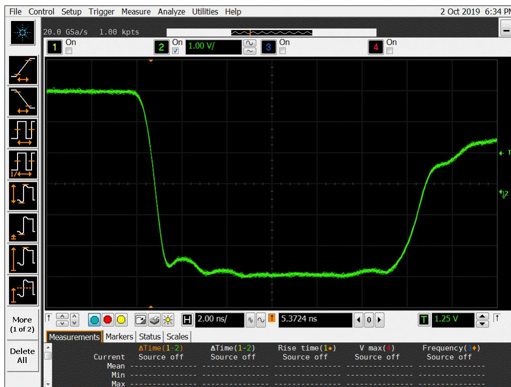
**Figure 17b DUT 6199 Post-Annealing Falling Edge**
