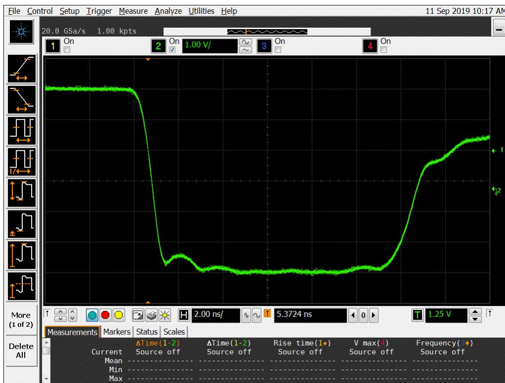
**Figure 20a DUT 6180 Pre-Irradiation Falling Edge**
