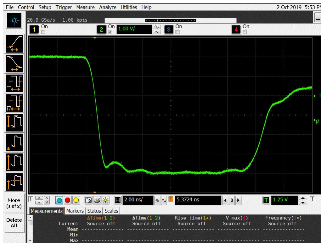
**Figure 19b DUT 6176 Post-Annealing Falling Edge**
