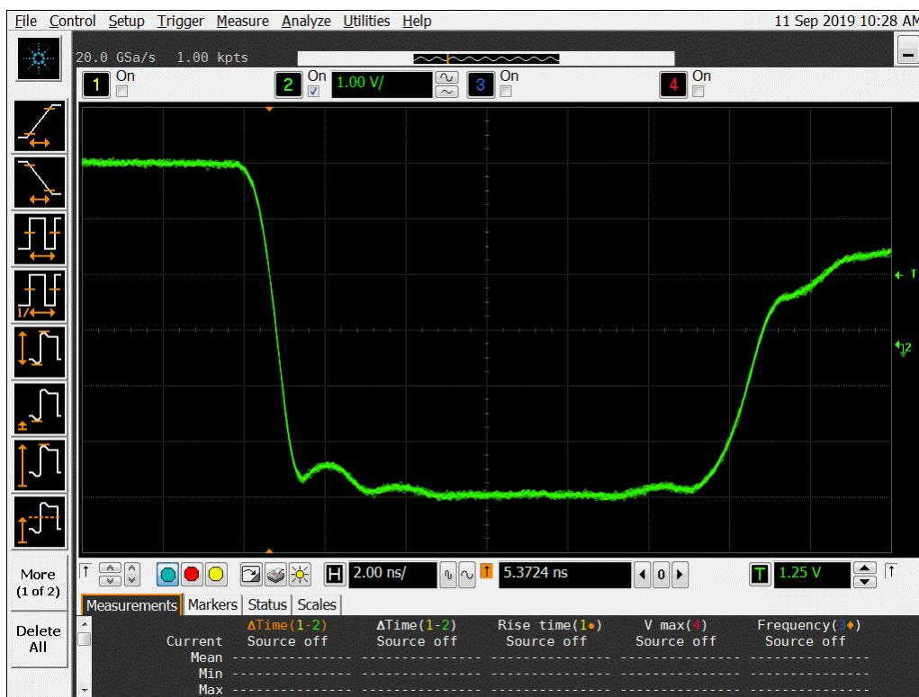
**Figure 16a DUT 6220 Pre-Irradiation Falling Edge**
