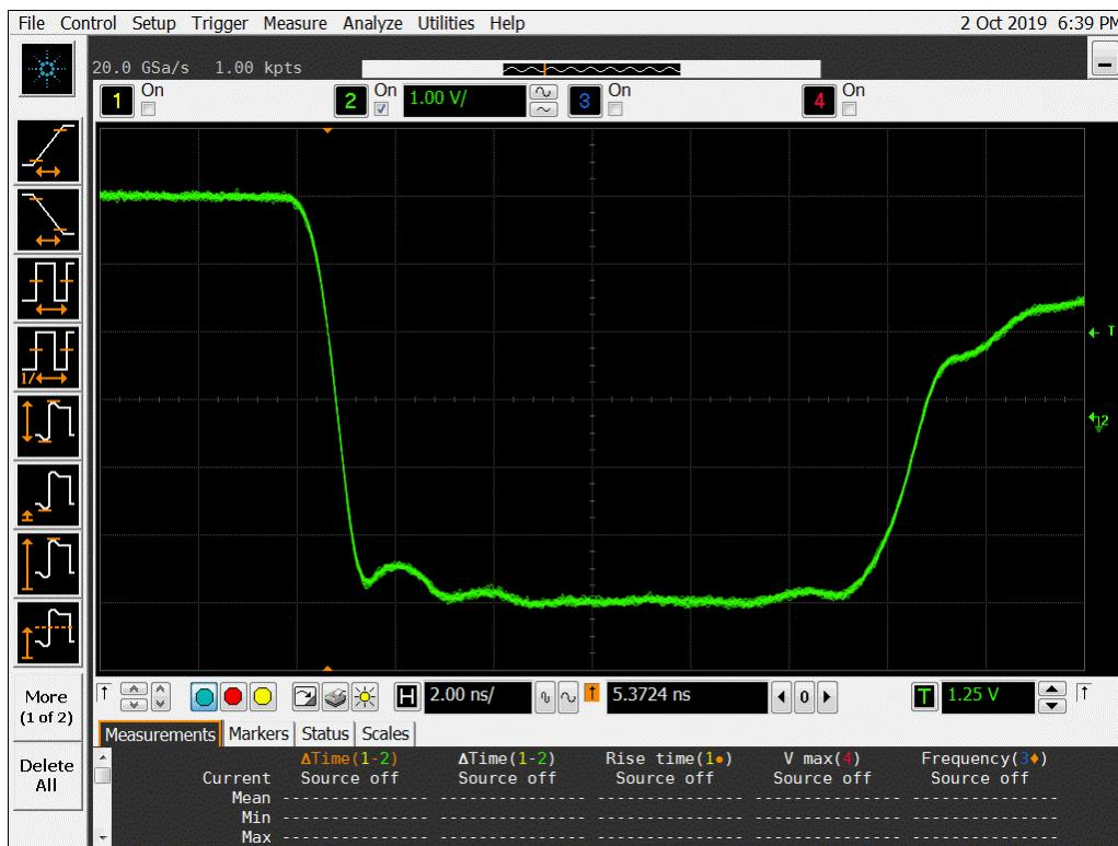
**Figure 20b DUT 6180 Post-Annealing Falling Edge**
