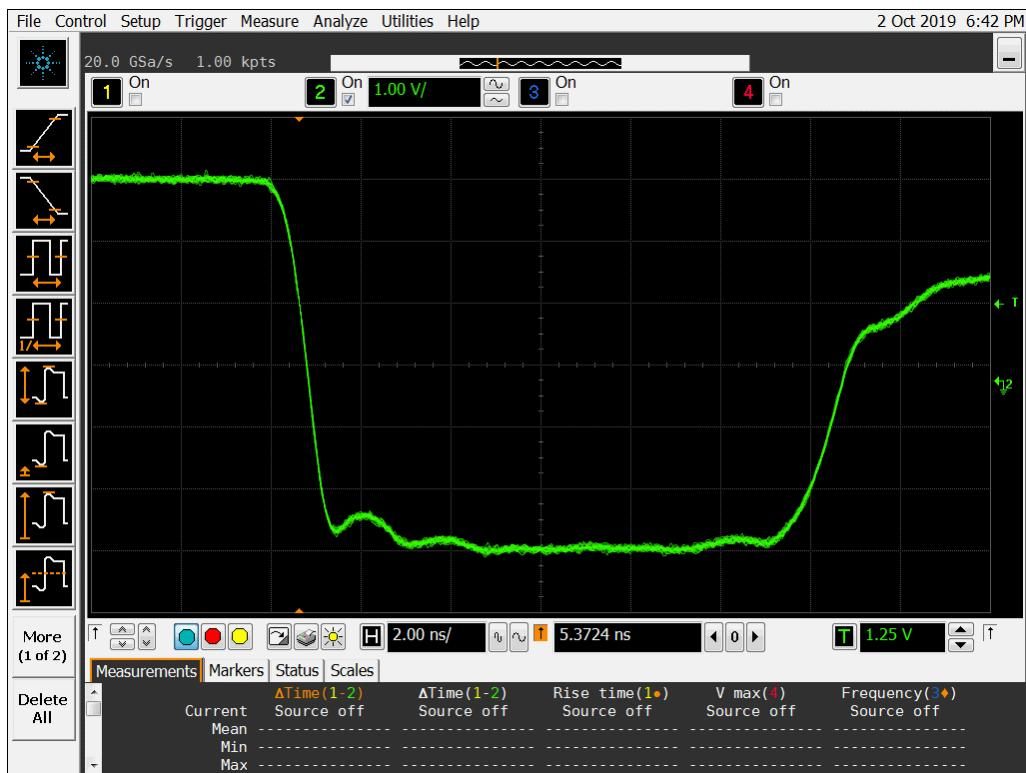
**Figure 18b DUT 6201 Post-Annealing Falling Edge**
