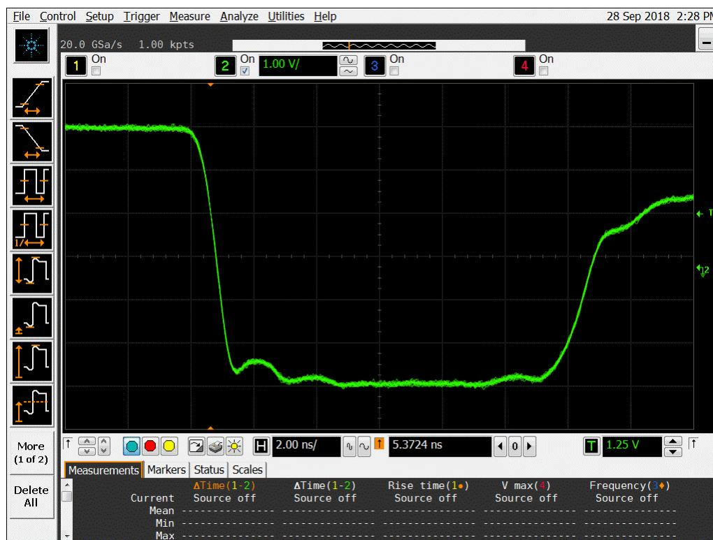
**Figure 17b DUT 7224 Post-Annealing Falling Edge**
