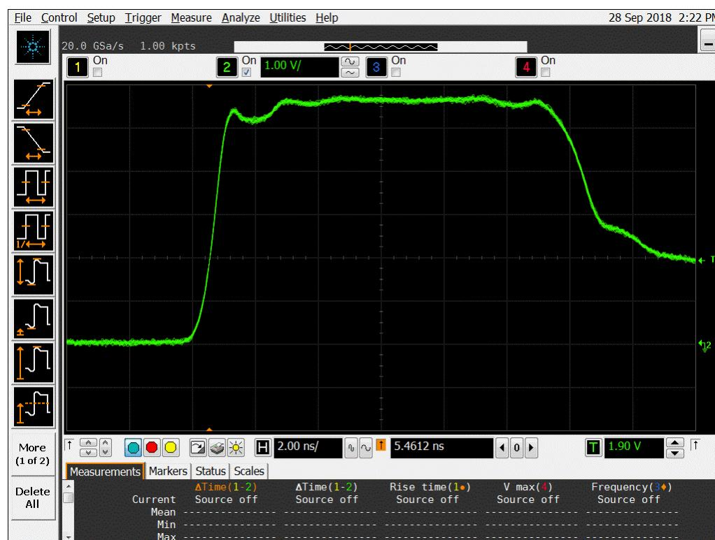
**Figure 13b DUT 7220 Post-Annealing Rising Edge**
