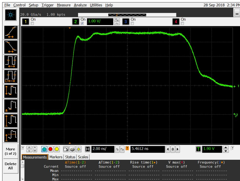
Figure 9b DUT 7253 Post-Annealing Rising Edge
