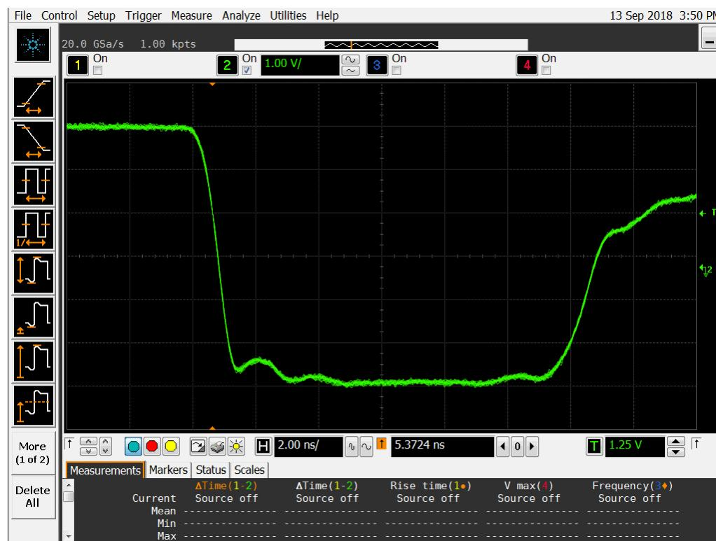
**Figure 19a DUT 7220 Pre-Irradiation Falling Edge**
