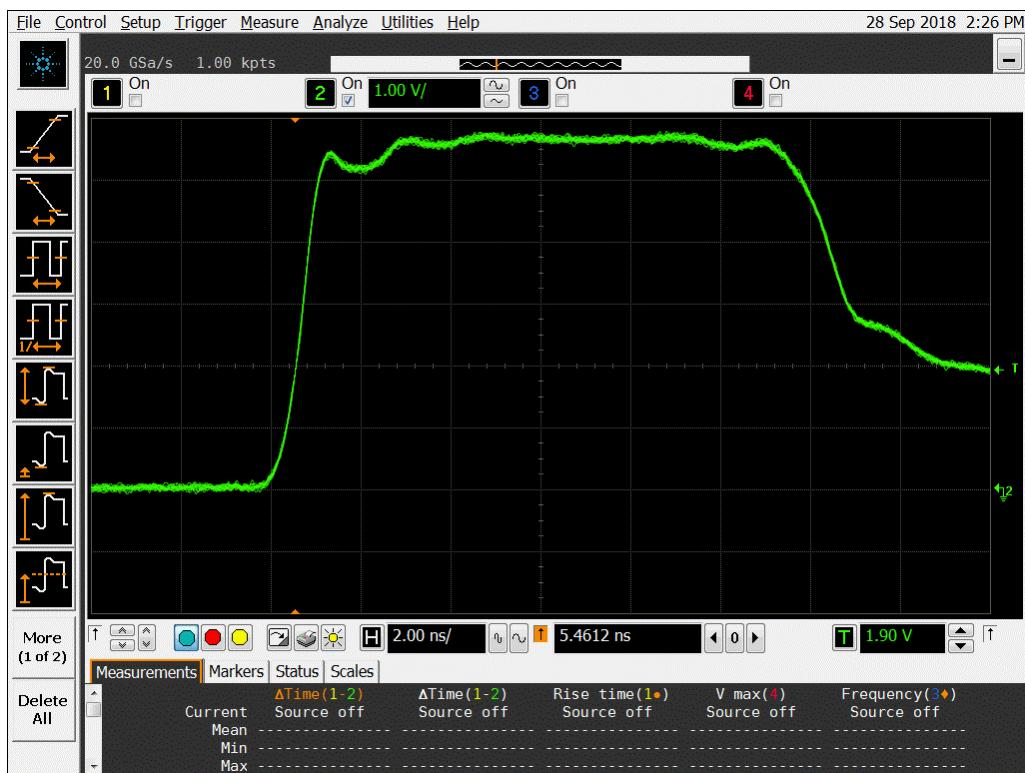
**Figure 14b DUT 7223 Post-Annealing Rising Edge**
