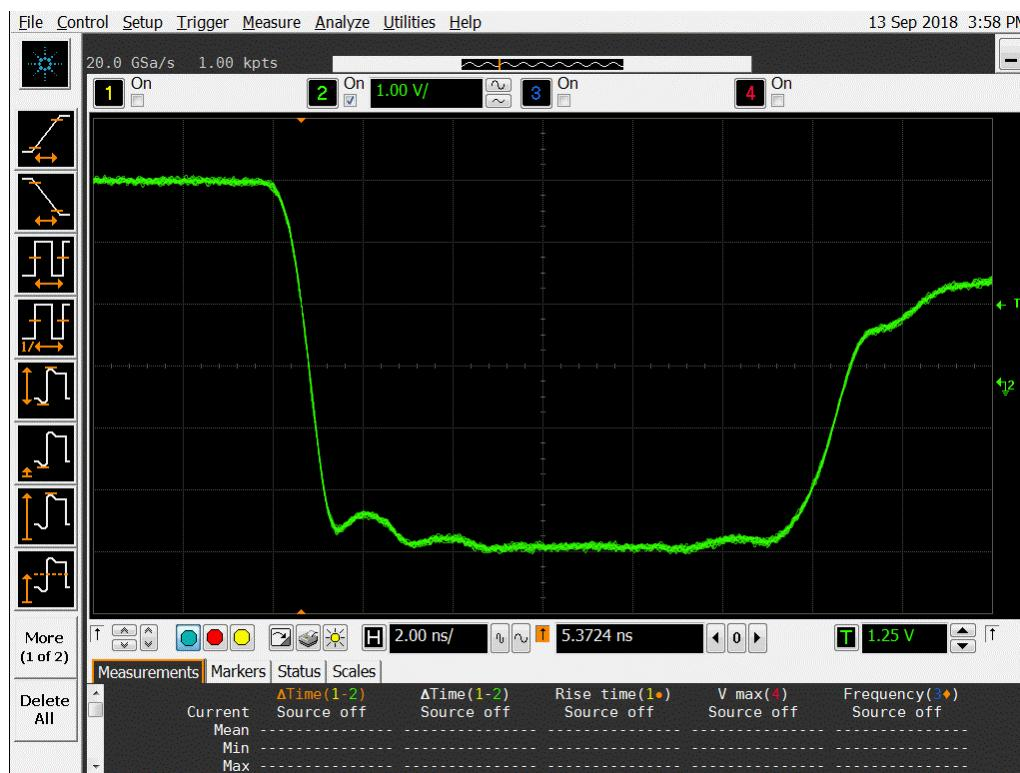
**Figure 17a DUT 7224 Pre-Irradiation Falling Edge**
