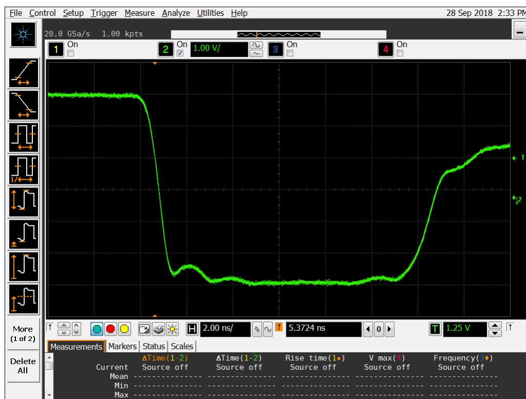
**Figure 18b DUT 7226 Post-Annealing Falling Edge**
