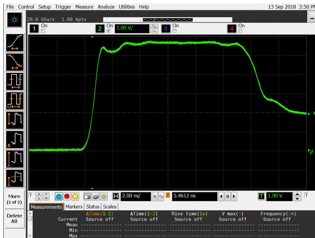
**Figure 13a DUT 7220 Pre-Irradiation Rising Edge**
