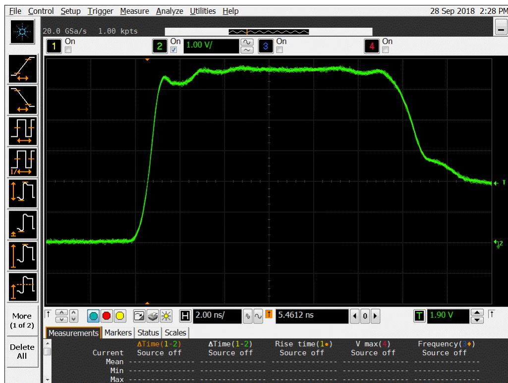
Figure 11b DUT 7224 Post-Annealing Rising edge
