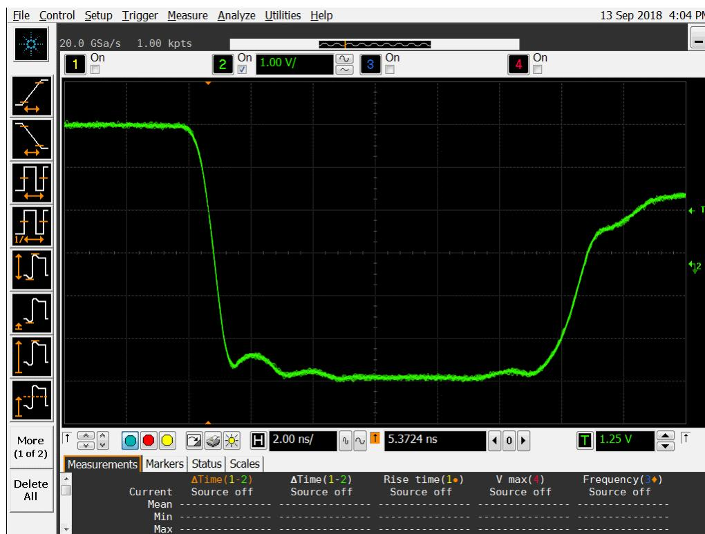
**Figure 15a DUT 7253 Pre-Radiation Falling Edge**
