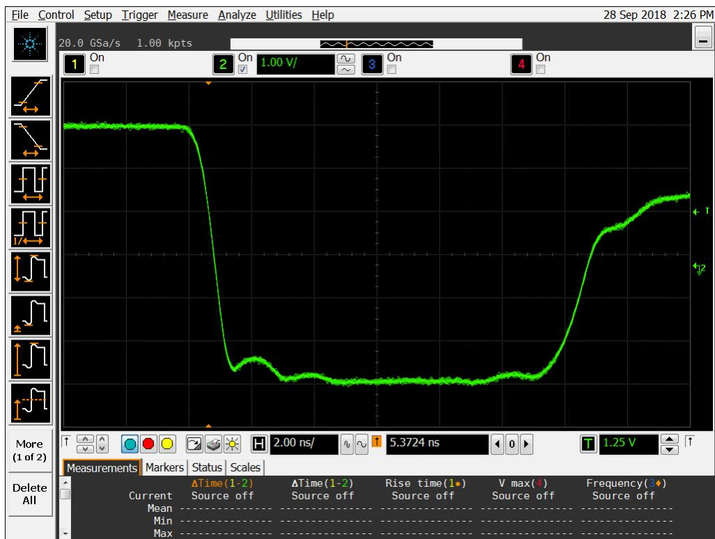
**Figure 20b DUT 7223 Post-Annealing Falling Edge**
