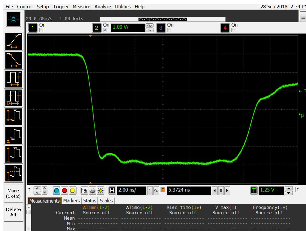
**Figure 15b DUT 7253 Post-Annealing Falling Edge**
