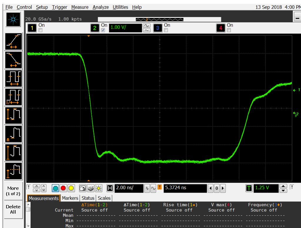
**Figure 18a DUT 7226 Pre-Irradiation Falling Edge**
