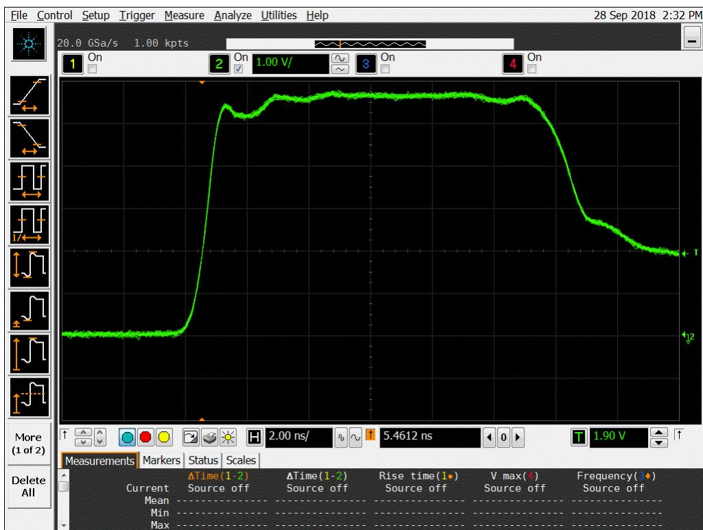
**Figure 12b DUT 7226 Post-Annealing Rising Edge**
