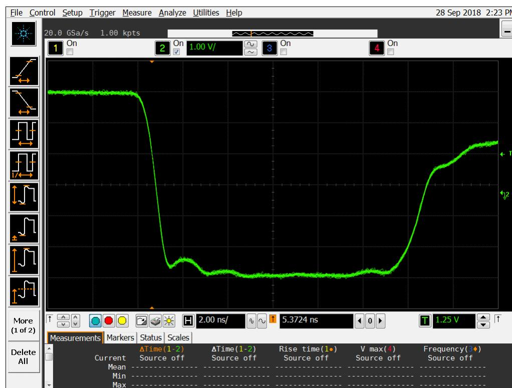
**Figure 19b DUT 7220 Post-Annealing Falling Edge**
