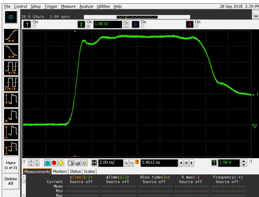
**Figure 10b DUT 7255 Post-Annealing Rising Edge**
