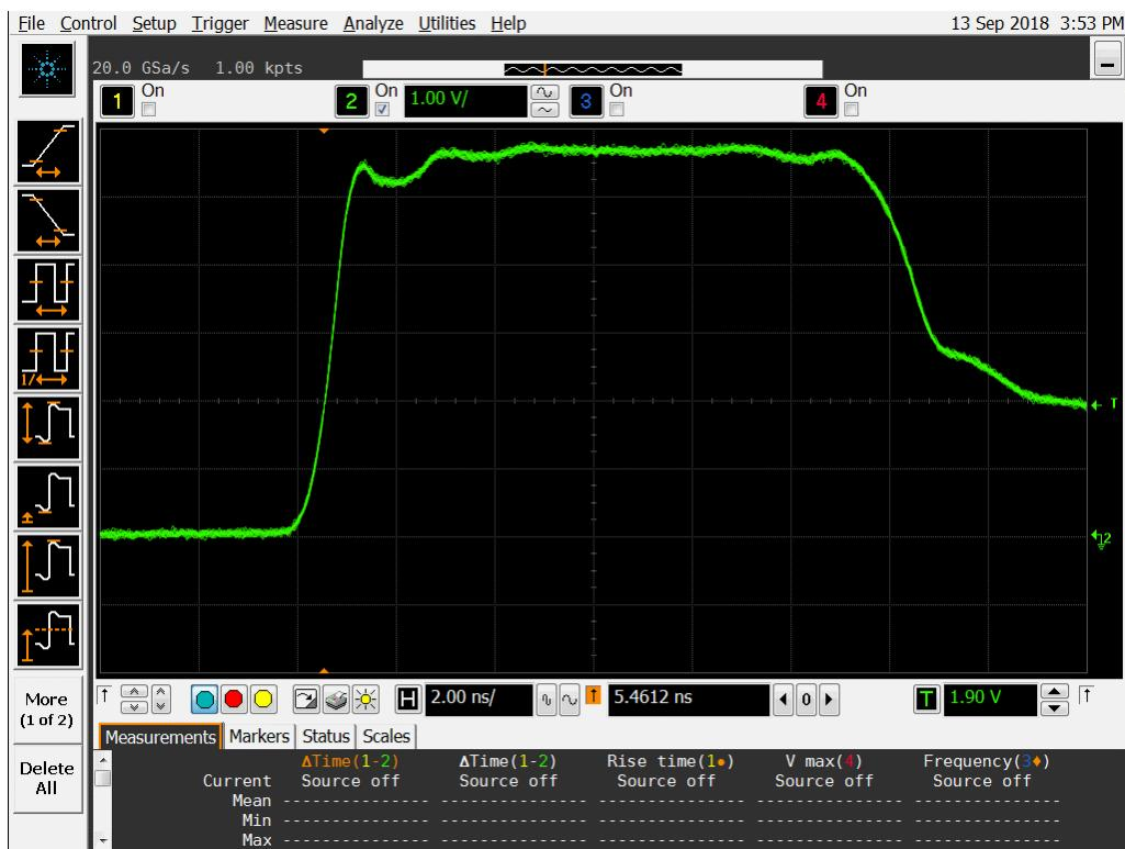
**Figure 14a DUT 7223 Pre-Irradiation Rising Edge**
