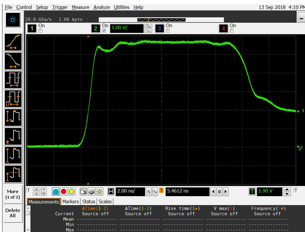
**Figure 10a DUT 7255 Pre-Irradiation Rising Edge**
