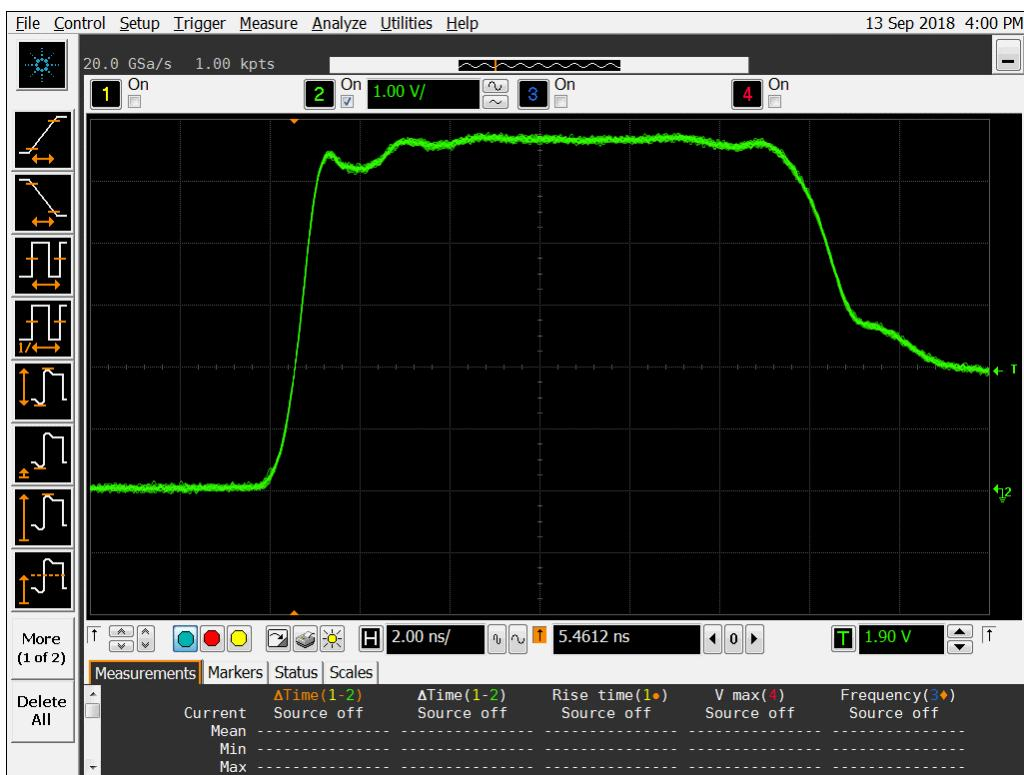
**Figure 12a DUT 7226 Pre-Irradiation Rising Edge**
