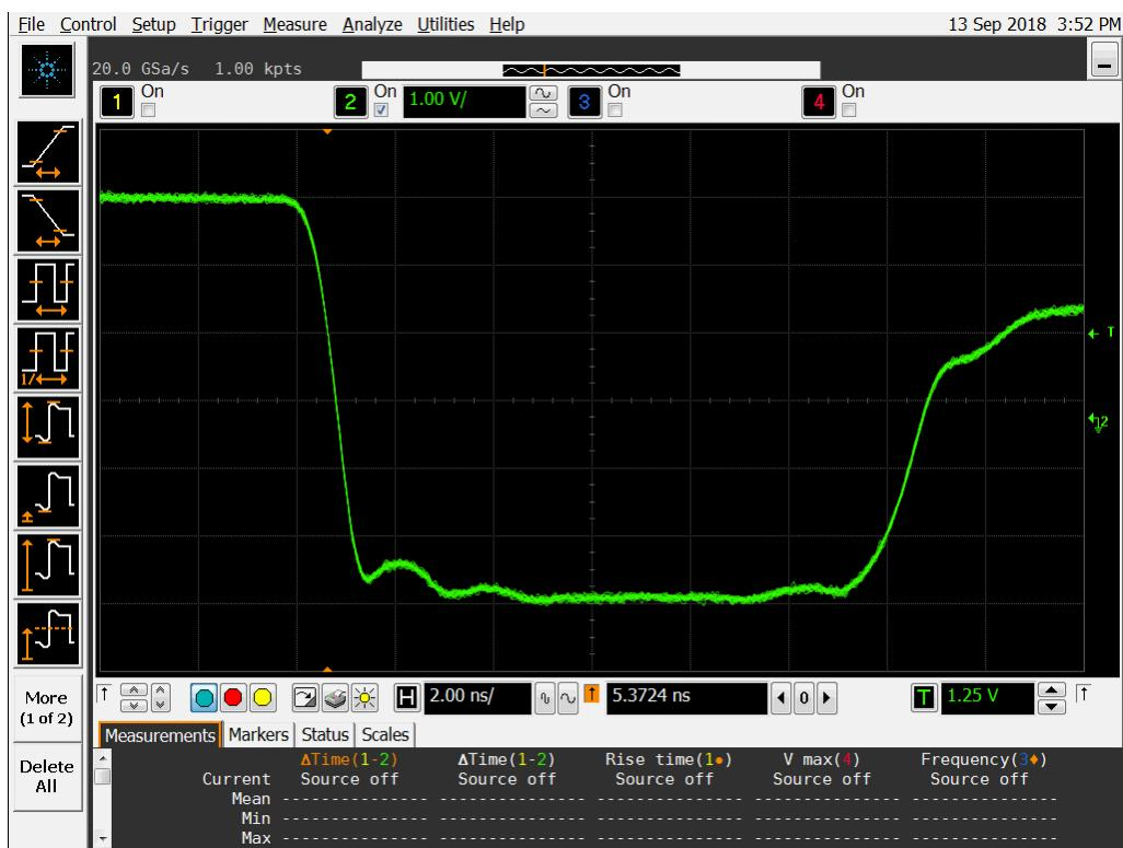
**Figure 20a DUT 7223 Pre-Irradiation Falling Edge**
