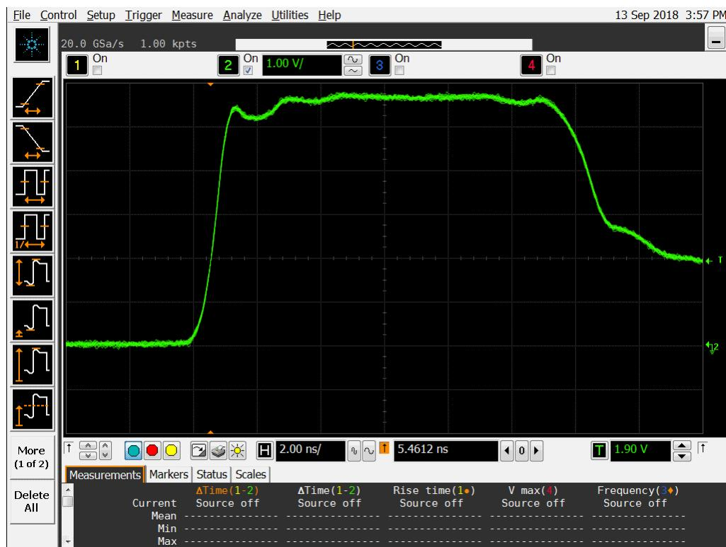
Figure 11a DUT 7224 Pre-Radiation Rising Edge
