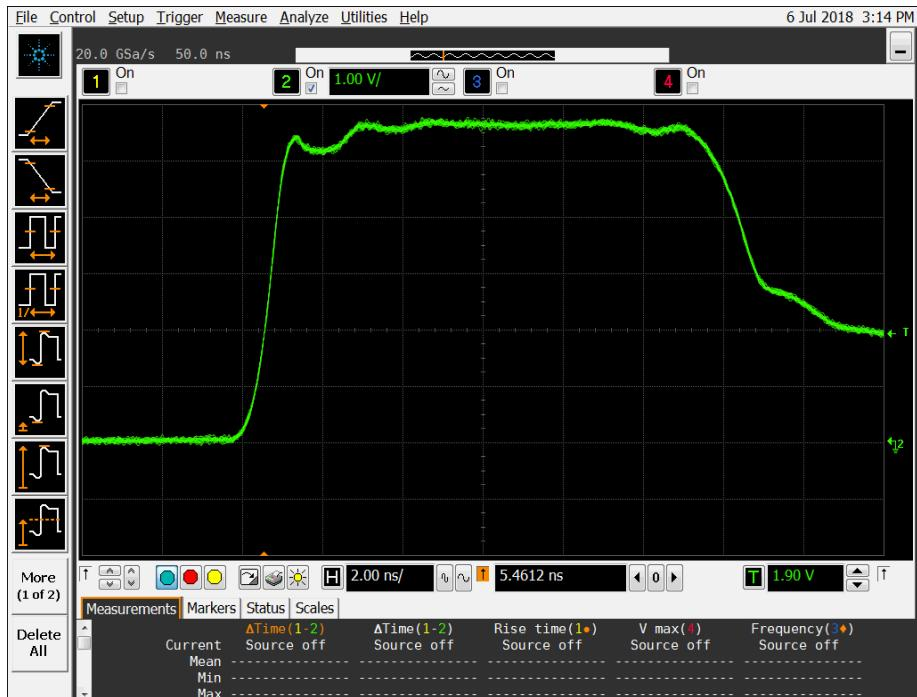
Figure 10a: DUT 3363 Pre-Irradiation Rising Edge
