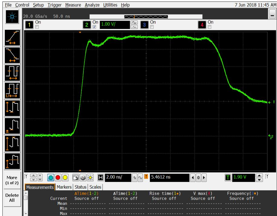
Figure 9b: DUT 3361 Post-Annealing Rising Edge
