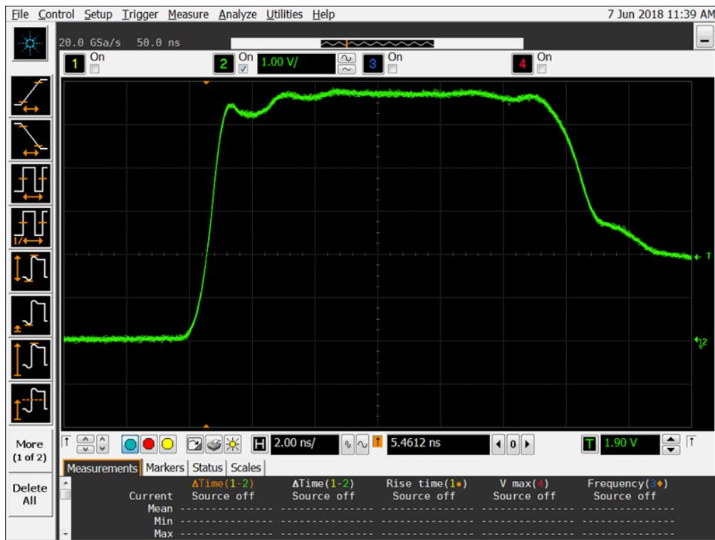
Figure 14b: DUT 3337 Post-Annealing Rising Edge
