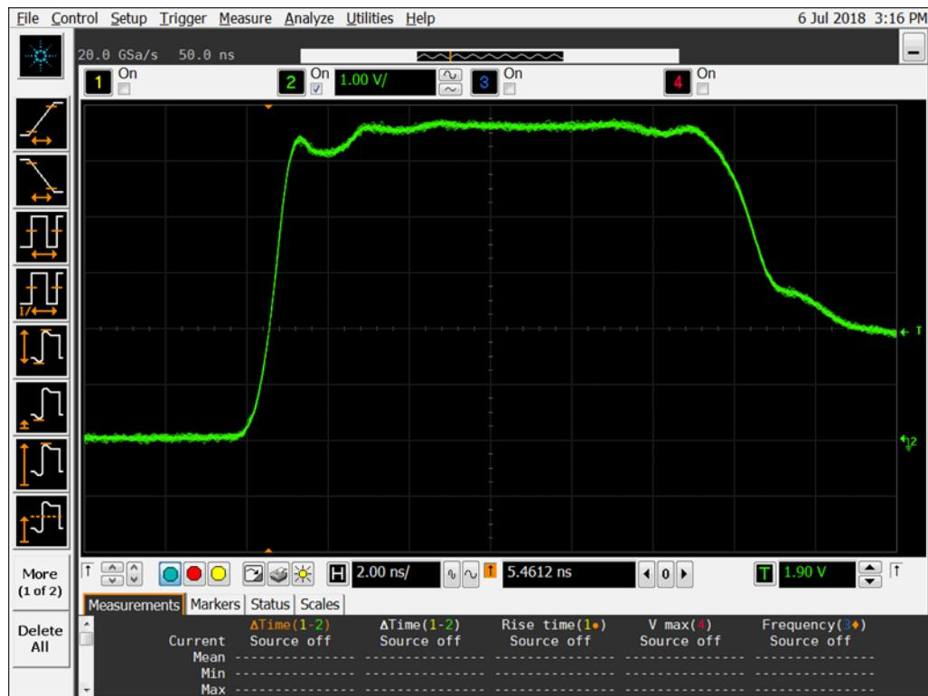
Figure 11a: DUT 3338 Pre-Radiation Rising Edge
