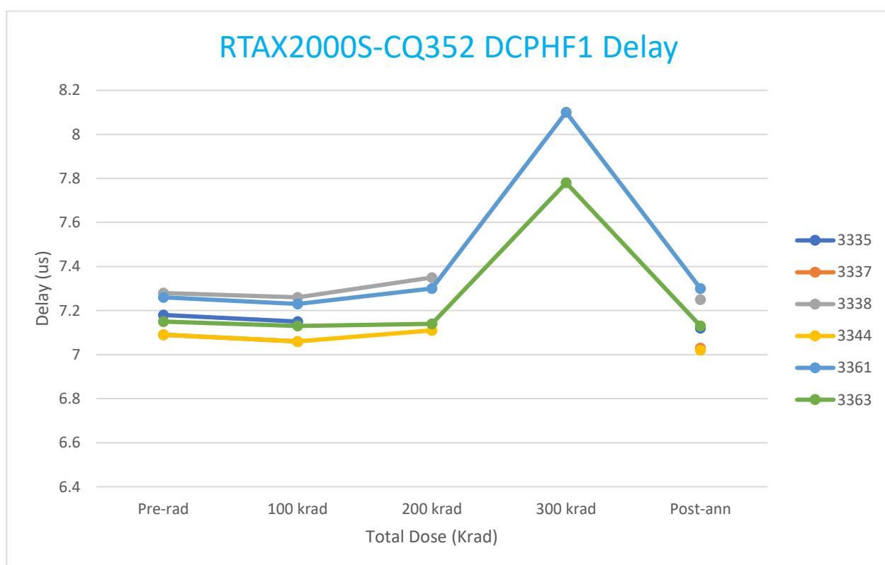
Table 8 Radiation-Induced Propagation Delay Degradations
