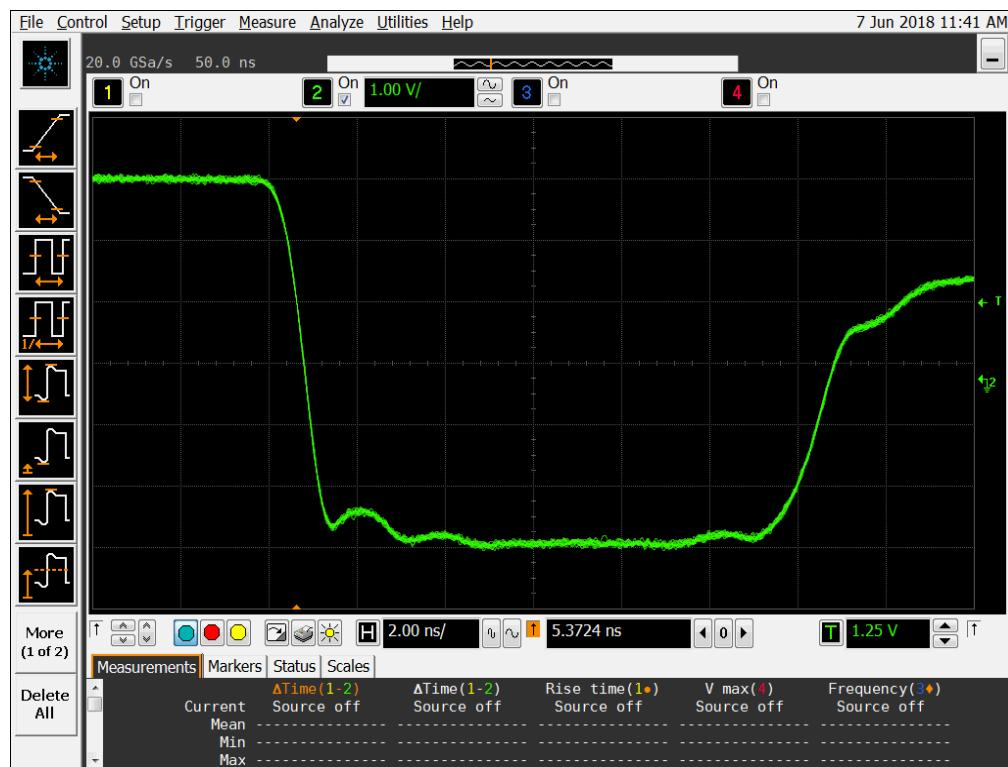
Figure 17b: DUT 3338 Post-Annealing Falling Edge
