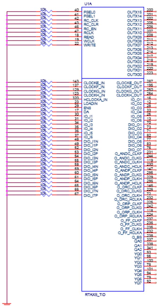
Figure A2: Power Supply, Ground and Special Pins Bias During Irradiation
