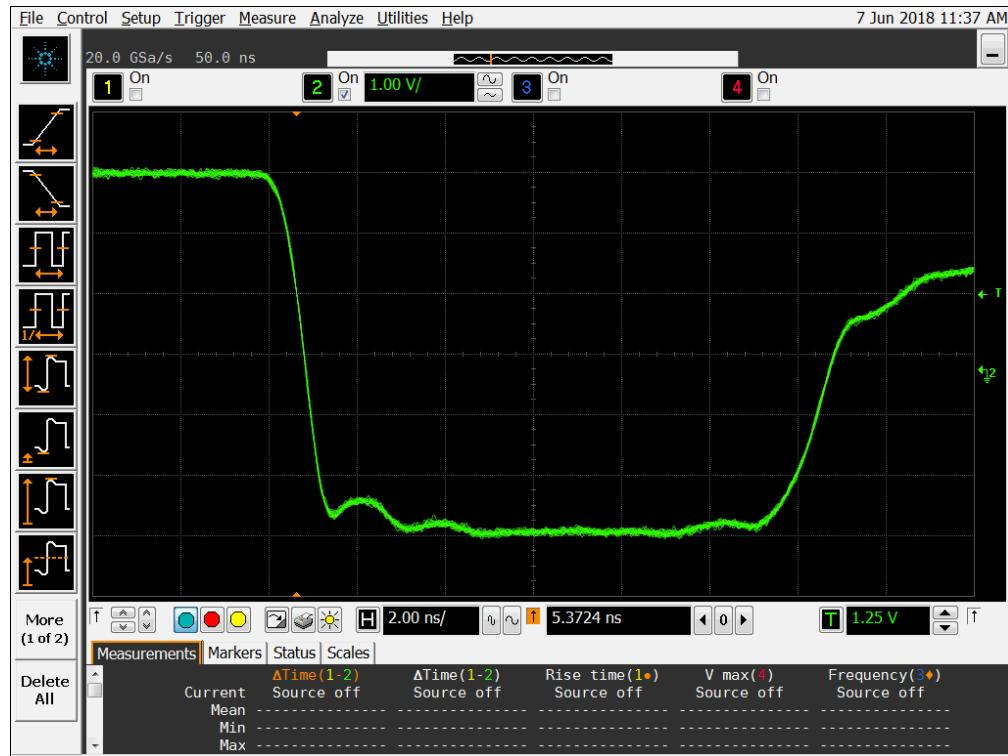
Figure 19b: DUT 3335 Post-Annealing Falling Edge
