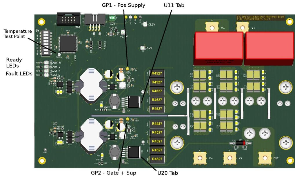
The PCB is shipped configured for  $-5\text{ V}$ ,  $20\text{ V}$  gate drive. R82 and R37 should be shorted to yield  $-5\text{ V}$ ,  $18\text{ V}$  gate drive. Four test points are shown in the above diagram GP1 to U11 tab should measure  $25\text{ V}$  when configured for  $20\text{ V}$  gate drive and  $23\text{ V}$  with  $18\text{ V}$  gate drive. U11 tab to the corresponding module source lead should measure  $5\text{ V}$ . On the low side test point GP2 and U20 tab have the same role.
