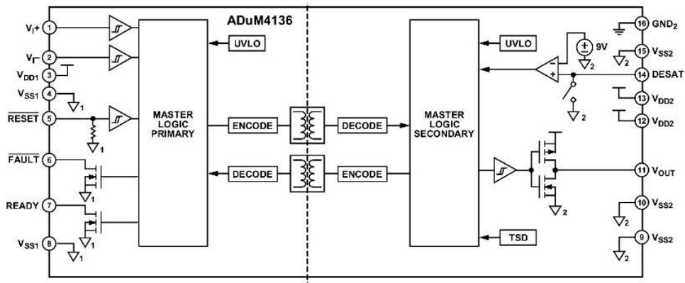
SiC MOSFETs have a much smaller die than their silicon counterpart. As a result they have lower thermal mass and heat faster in a short circuit condition. The following figure is from the ADuM4136 spec showing timing typical of an IGBT. With SiC MOSFETs, a delay of 200 ns–300 ns would be more appropriate than 2 μs delay.
