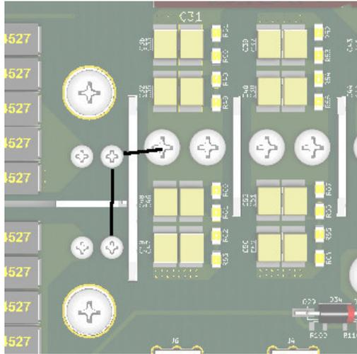
**Figure 7 • Singled-ended Input Connection**
