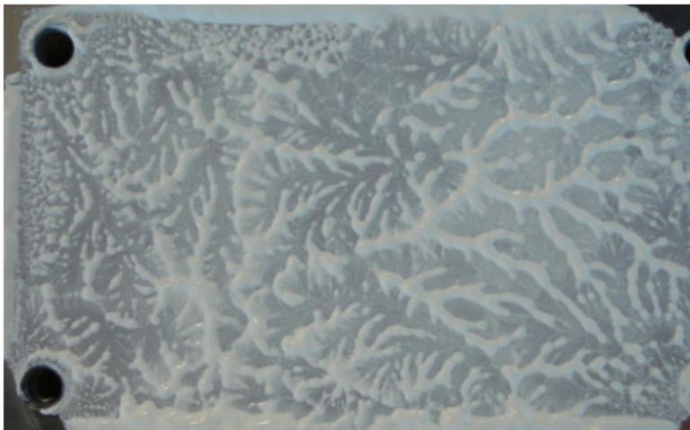
**Figure 3 • Grease on the module after disassembling**
