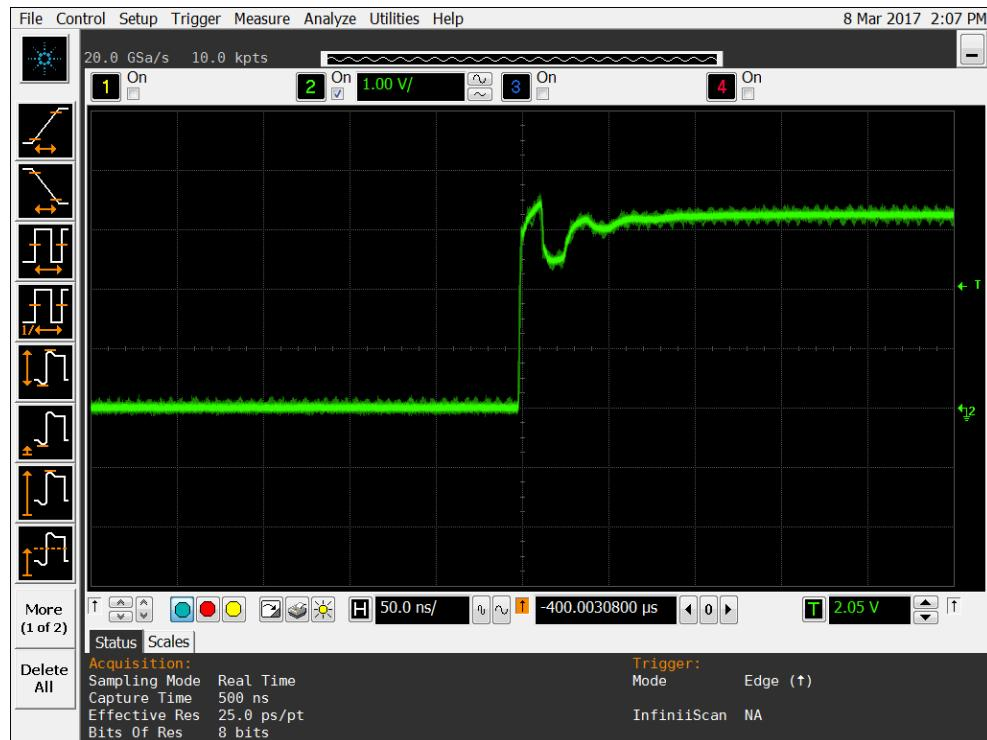
Figure 12a DUT 9416 Pre-Irradiation Rising Edge
