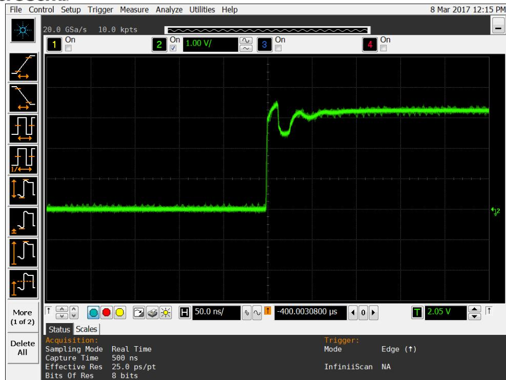
Figure 14a DUT 9440 Pre-Irradiation Rising Edge
