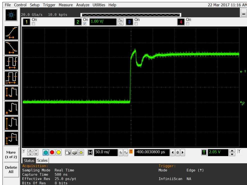
Figure 14b DUT 9440 Post-Annealing Rising Edge
