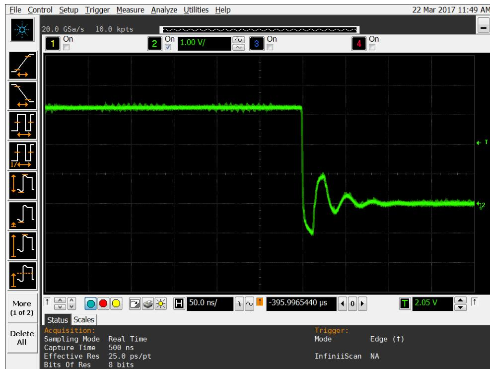
Figure 16b DUT 9400 Post-Annealing Falling Edge
