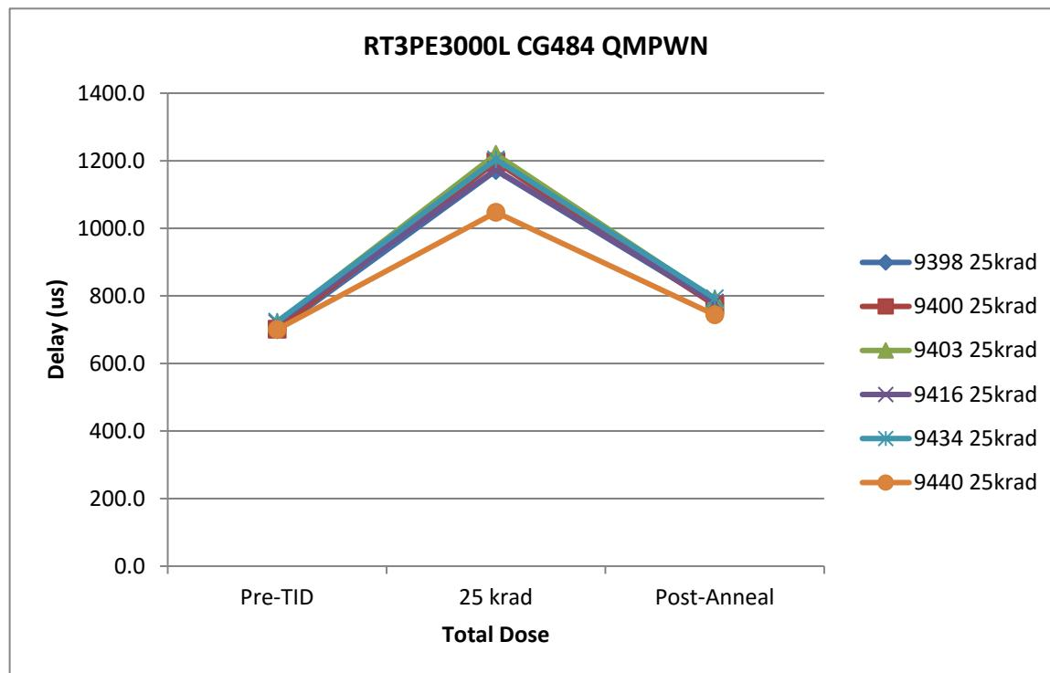
**Figure 8 Degradation of Propagation Delay versus TID and Annealing**
