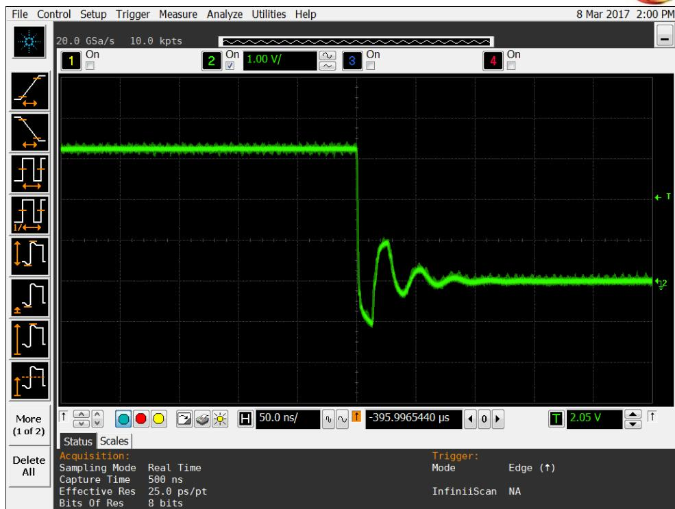
Figure 19a DUT 9434 Pre-Irradiation Falling Edge
