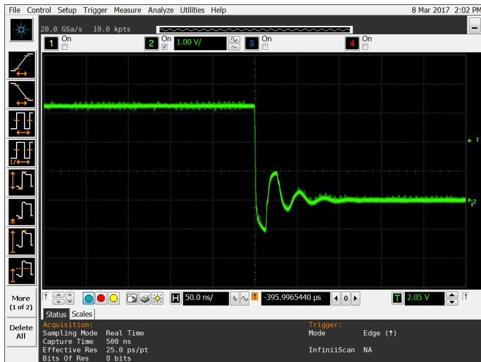
Figure 17a DUT 9403 Pre-Irradiation Falling Edge
