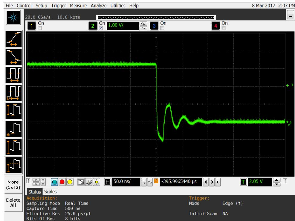
Figure 18a DUT 9416 Pre-Irradiation Falling Edge
