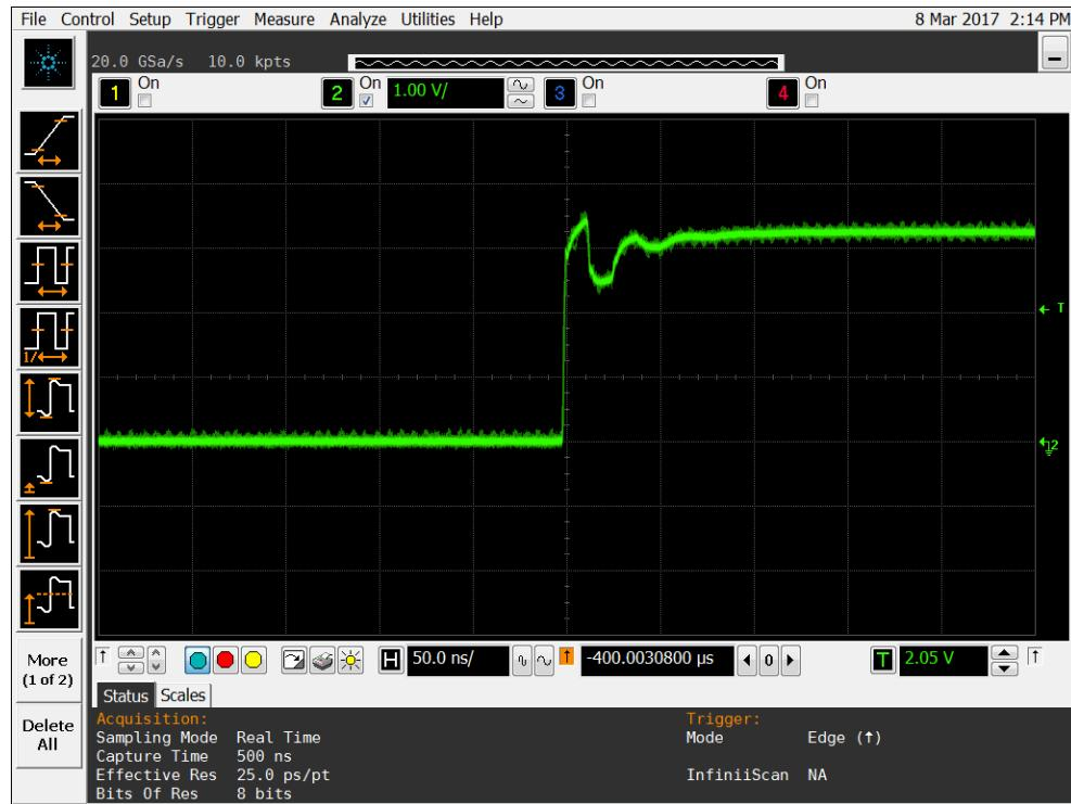
Figure 10a DUT 9400 Pre-Irradiation Rising Edge
