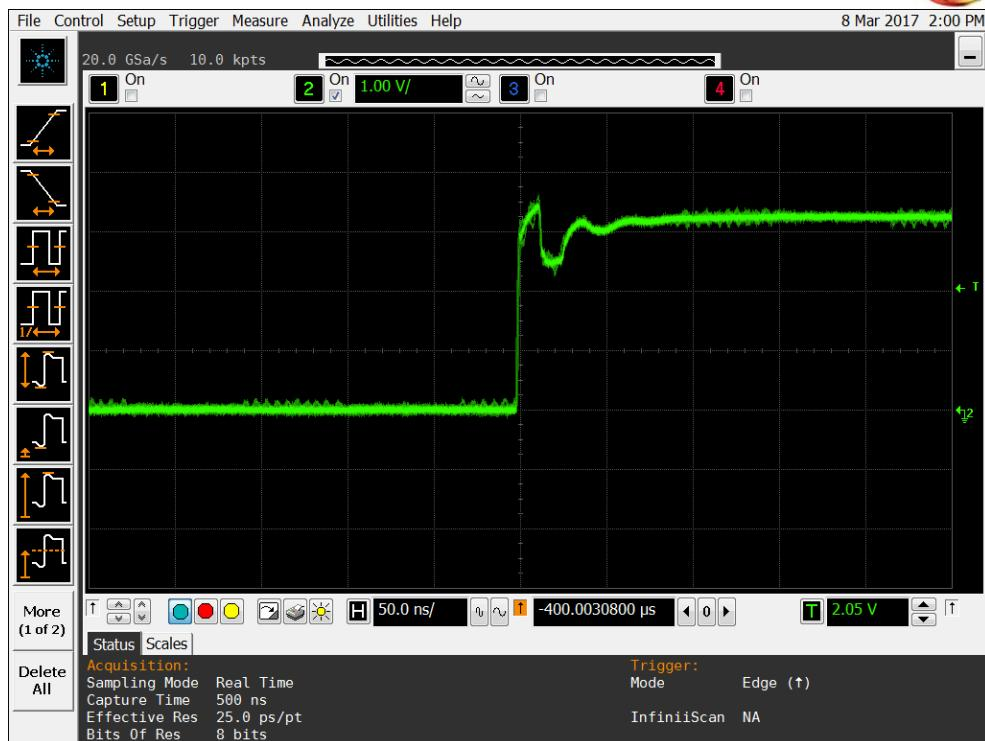
Figure 13a DUT 9434 Pre-Irradiation Rising Edge
