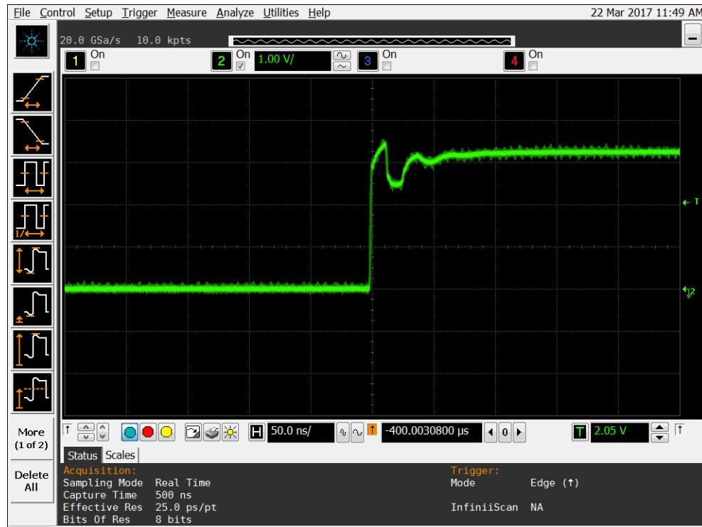
Figure 10b DUT 9400 Post-Annealing Rising Edge
