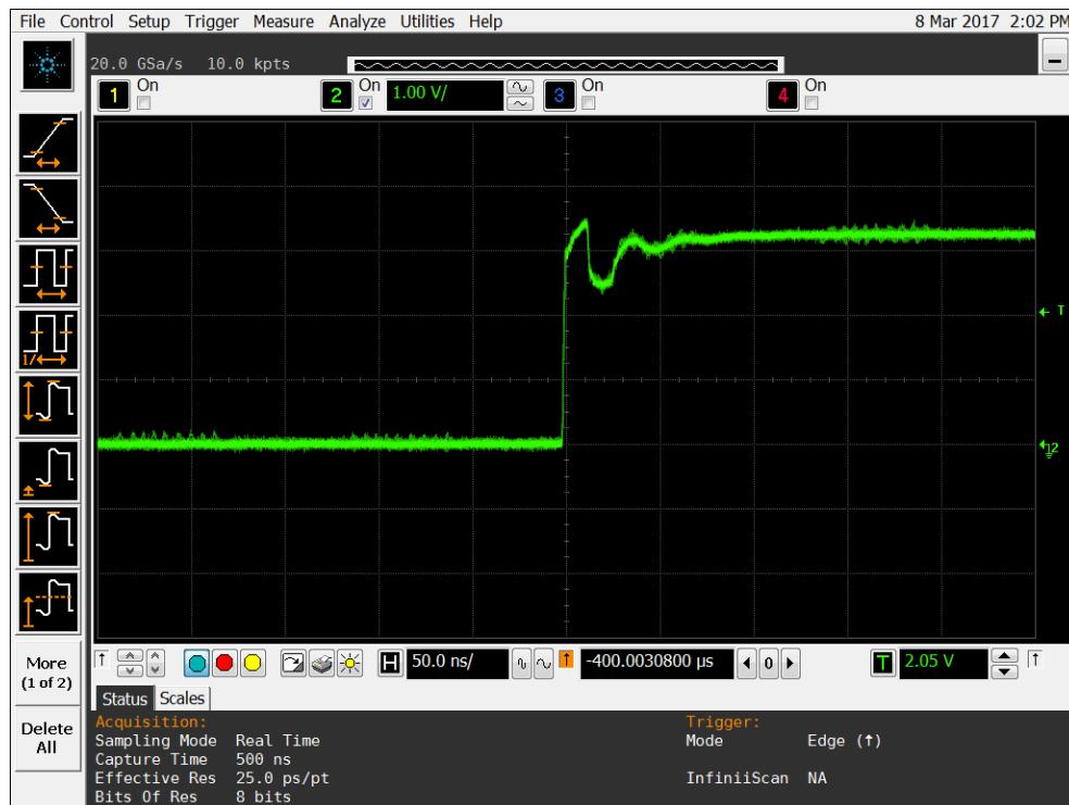
**Figure 11a DUT 9403 Pre-Irradiation Rising Edge**
