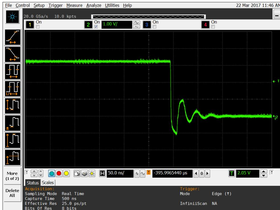
Figure 15b DUT 9398 Post-Annealing Falling Edge
