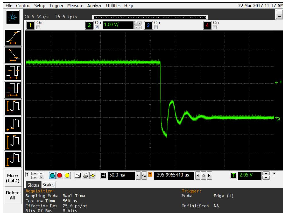
Figure 20b DUT 9440 Post-Annealing Falling Edge
