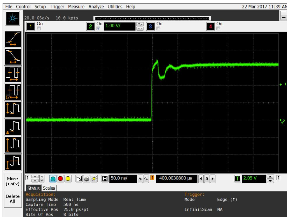
**Figure 11b DUT 9403 Post-Annealing Rising Edge**
