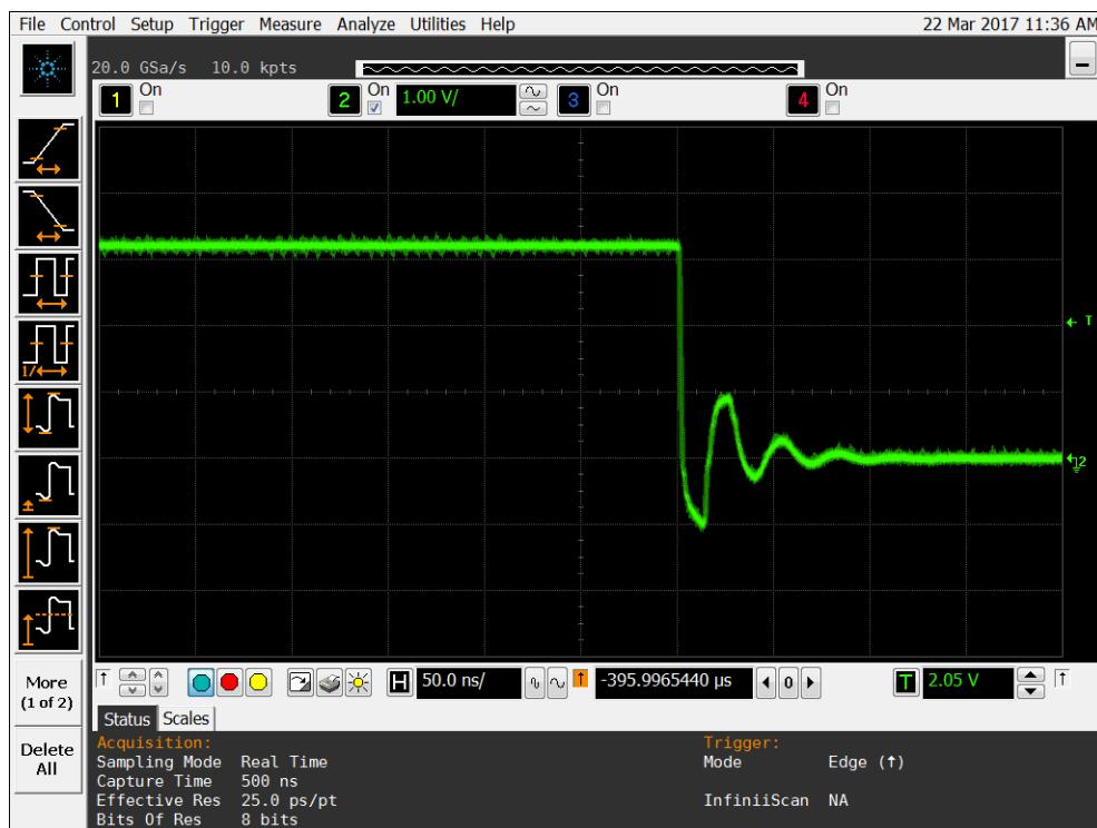
Figure 19b DUT 9434 Post-Annealing Falling Edge
