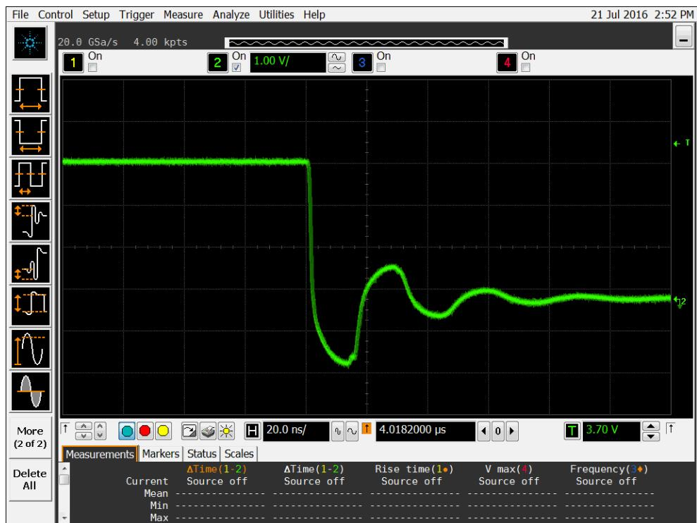
Figure 11a DUT 3439 Pre-Irradiation Falling Edge
