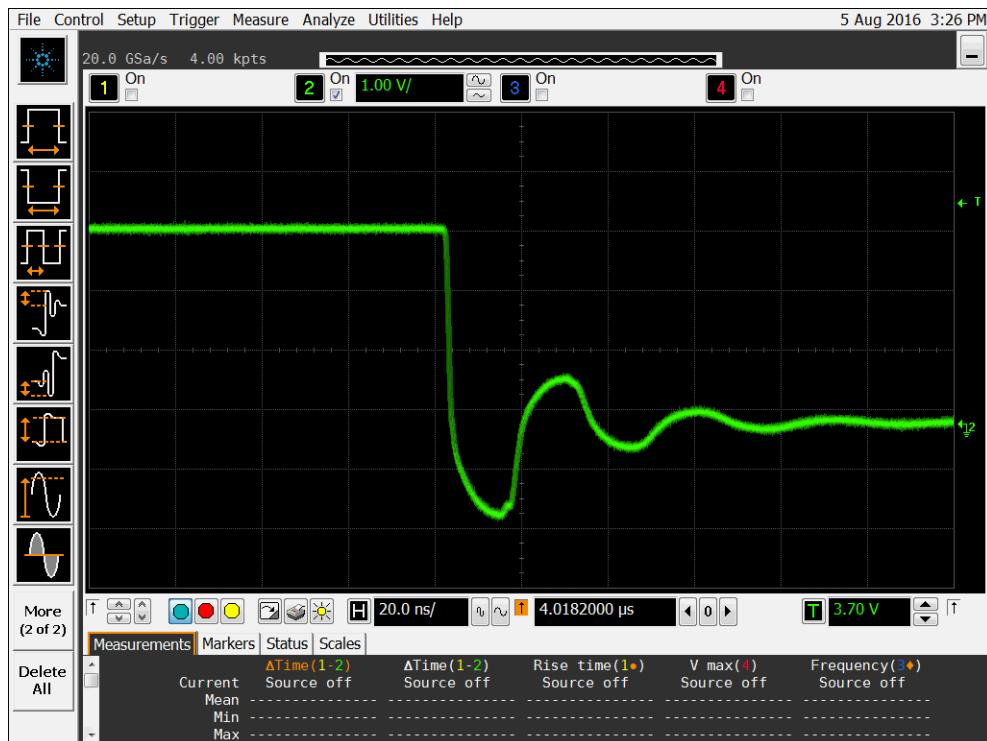
Figure 9b DUT 3436 Post-Annealing Falling Edge
