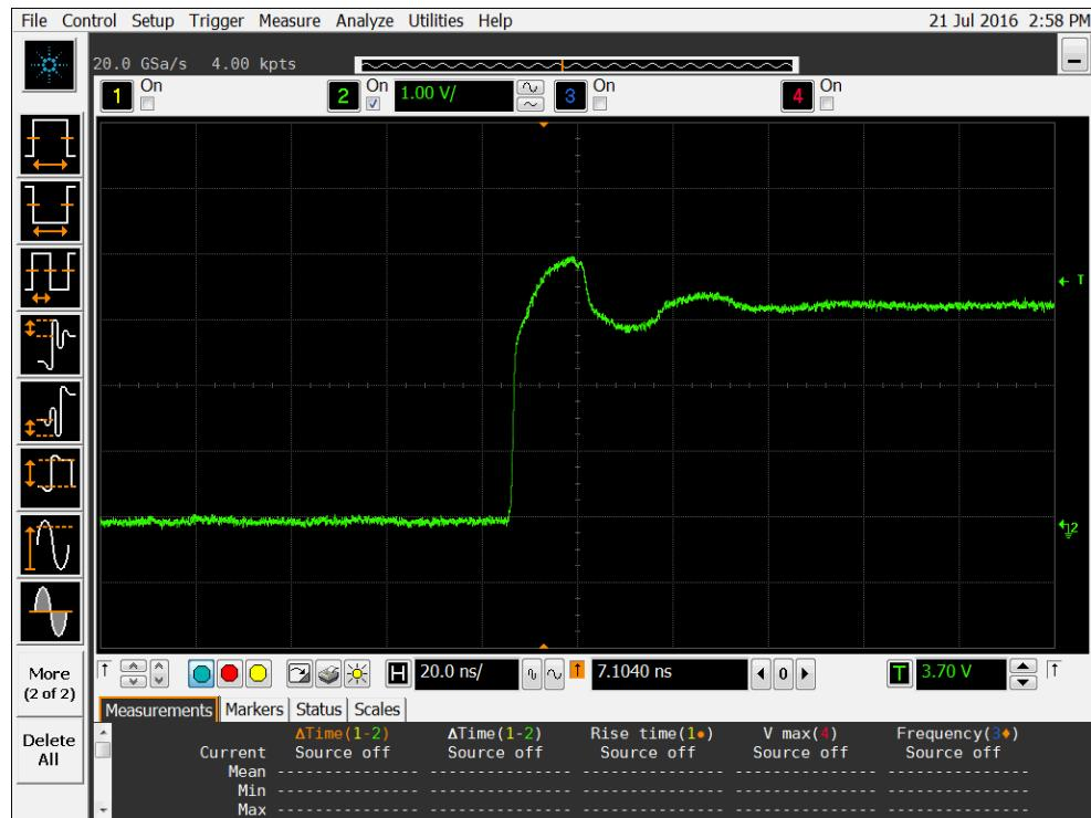
Figure 4a DUT 3436 Pre-Irradiation Rising Edge
