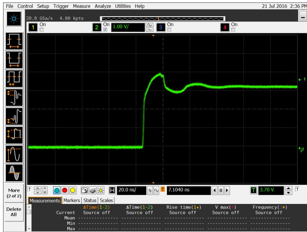
Figure 3a DUT 3435 Pre-Irradiation Rising Edge
