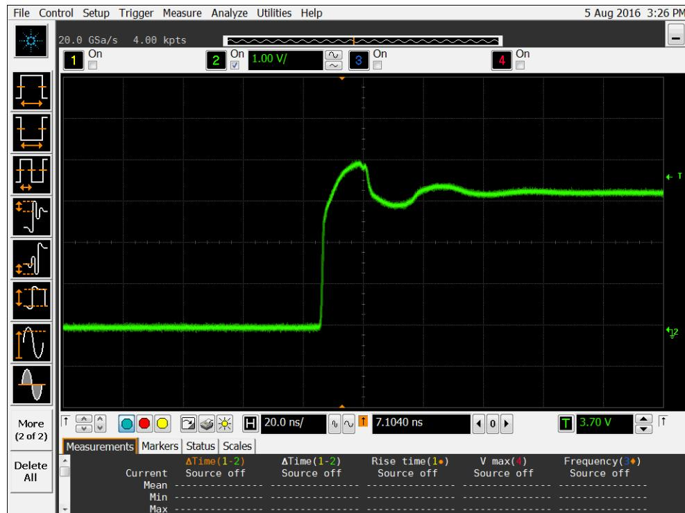
Figure 4b DUT 3436 Post-Annealing Rising Edge
