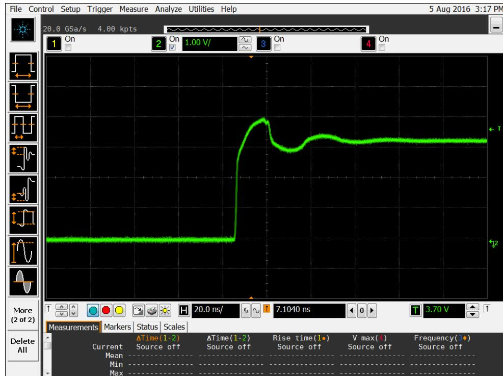
Figure 6b DUT 3439 Post-Annealing Rising Edge
