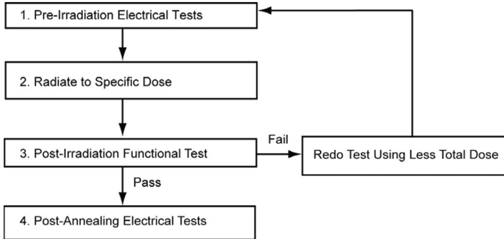
Figure Parametric Test Flow Chart
