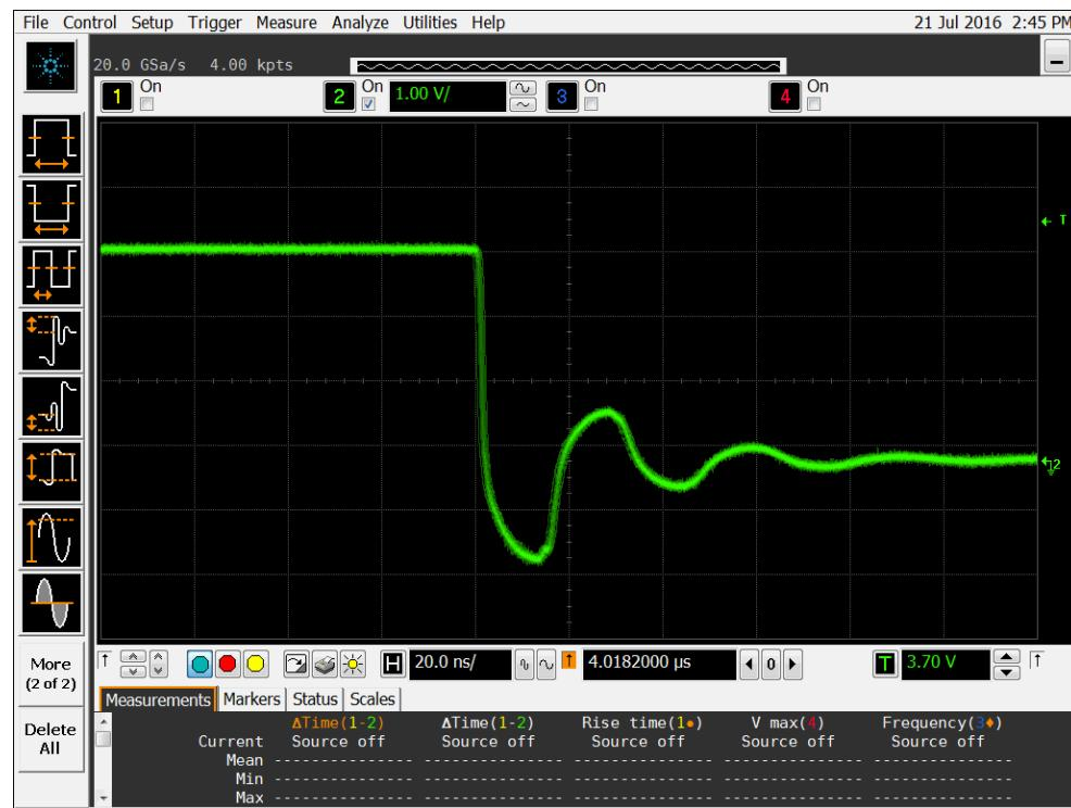
Figure 10a DUT 3437 Pre-Irradiation Falling Edge
