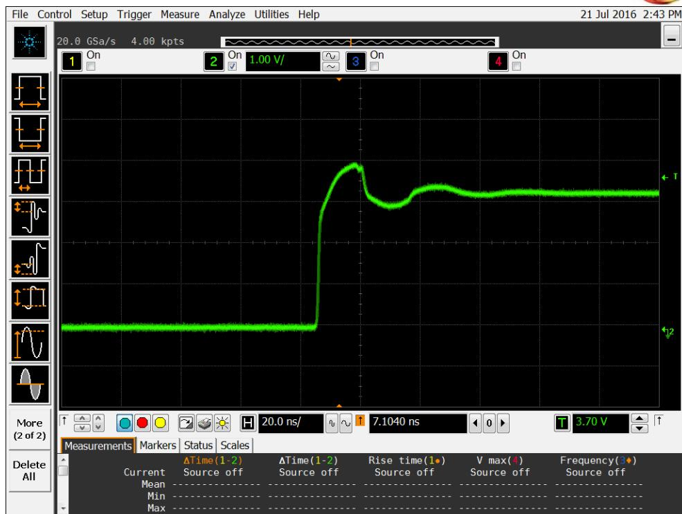
Figure 7a DUT 3556 Pre-Irradiation Rising Edge
