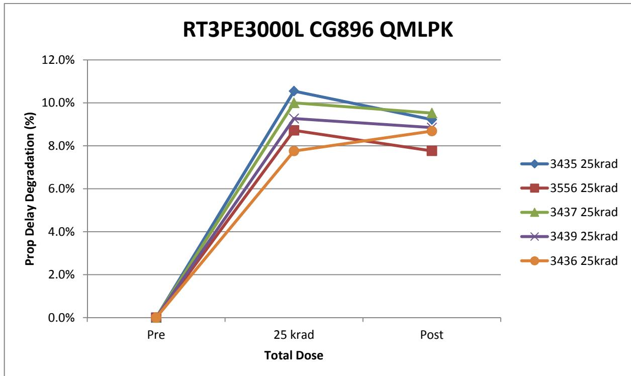
**Figure 2 Degradation of Propagation Delay versus TID and Annealing**
