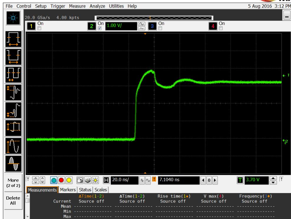
Figure 5a DUT 3437 Pre-Irradiation Rising Edge
