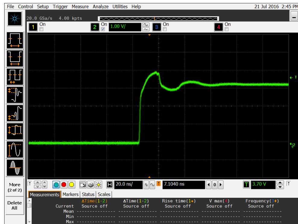
Figure 5b DUT 3437 Post-Annealing Rising Edge
