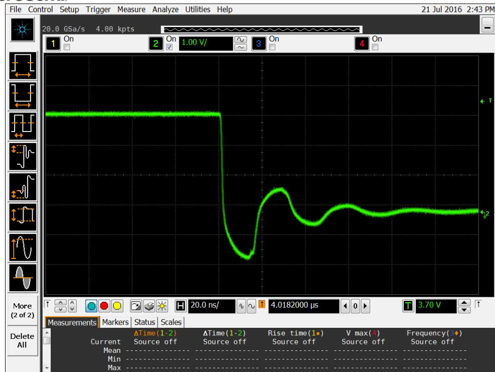
Figure 12a DUT 3556 Pre-Irradiation Falling Edge
