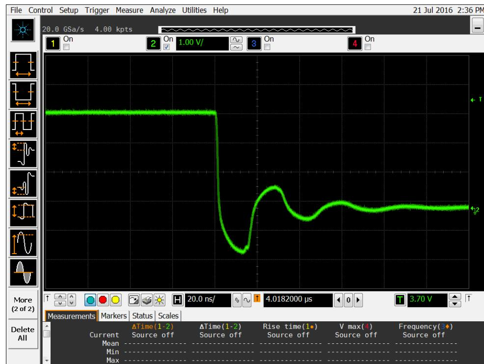
Figure 8a DUT 3435 Pre-Irradiation Falling Edge
