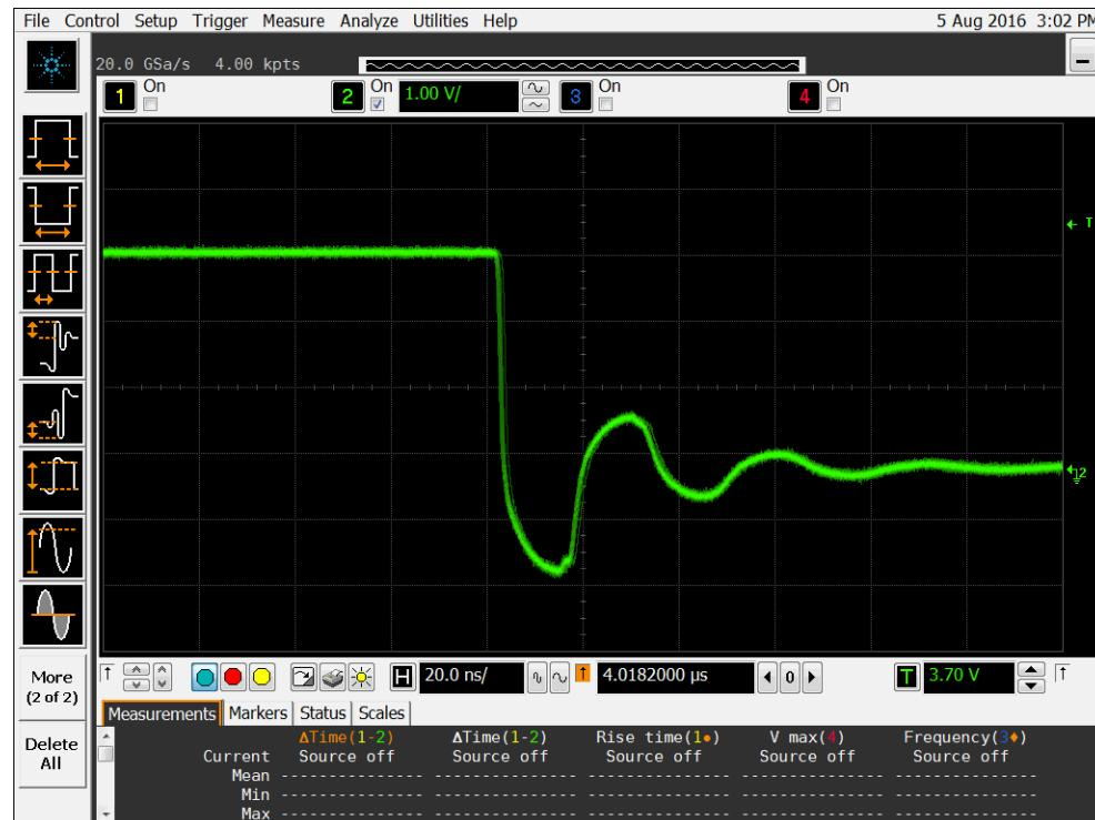
Figure 8b DUT 3435 Post-Annealing Falling Edge
