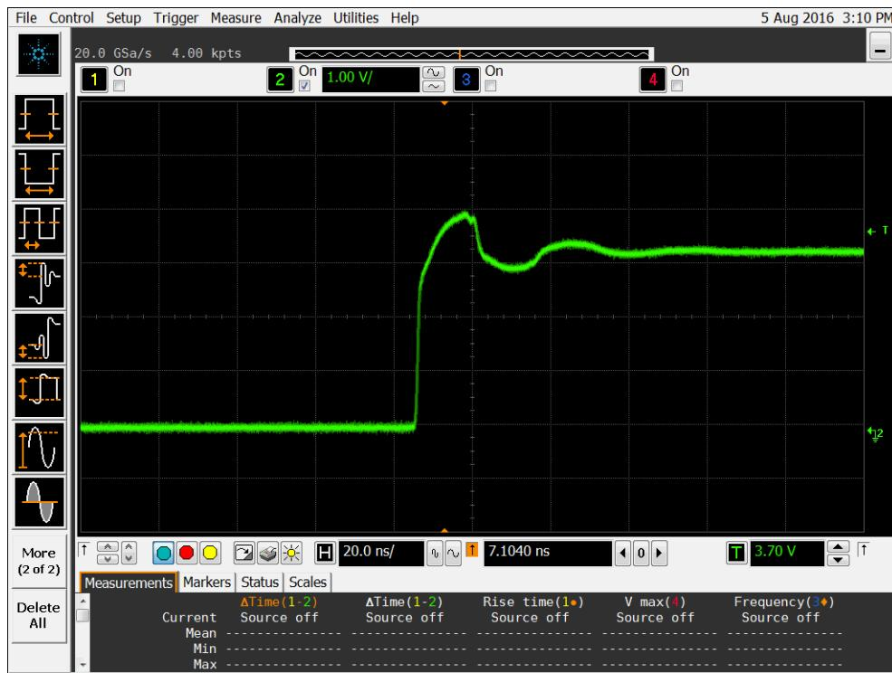
Figure 7b DUT 3556 Post-Annealing Rising Edge
