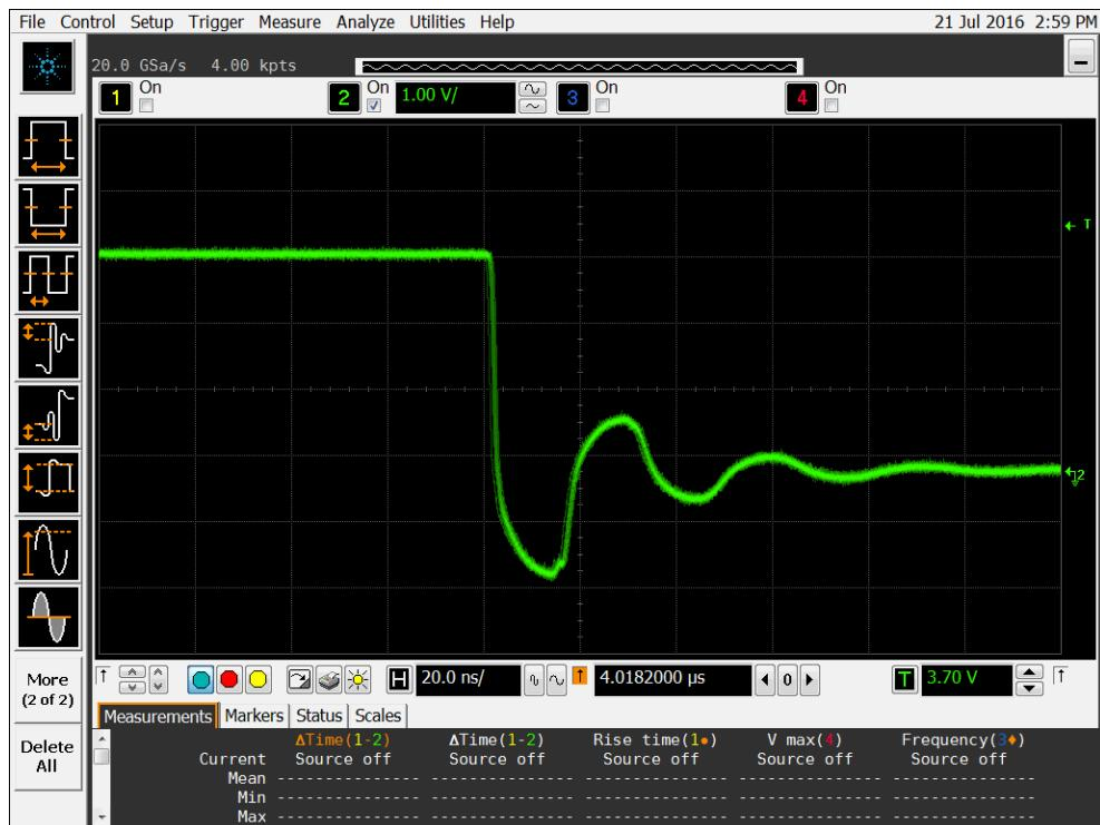
Figure 9a DUT 3436 Pre-Irradiation Falling Edge
