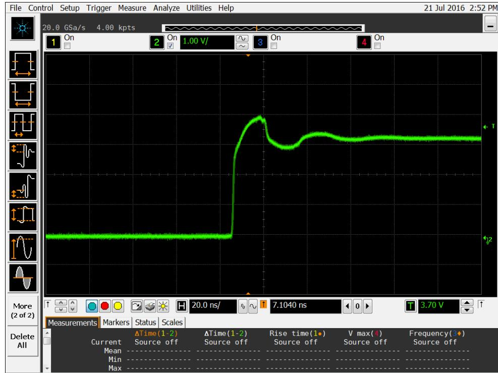
Figure 6a DUT 3439 Pre-Irradiation Rising Edge
