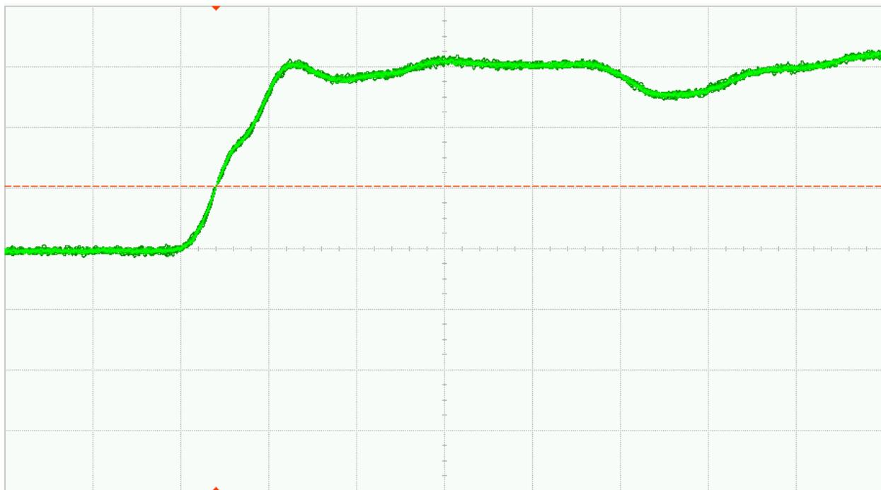
Fig. 29 (a). DUT 1744 pre-irradiation rising edge, abscissa scale is 1V/div and ordinate scale is 2ns/div
