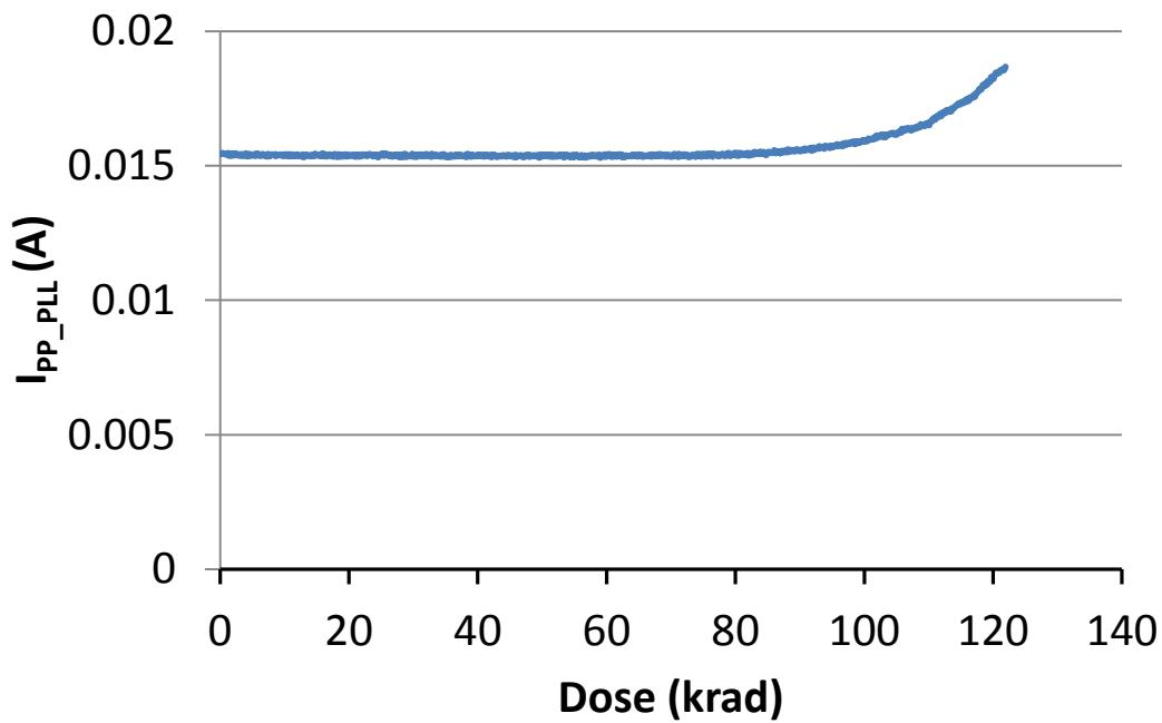
Fig. 24. DUT 1786 charge pump and PLL power supply current ( $I_{PP\_PLL}$ ) versus TID
