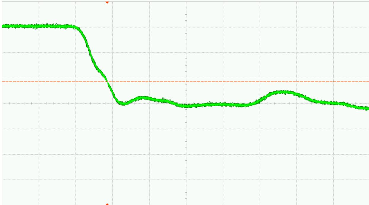
Fig. 36 (b). DUT 1786 post-annealing Falling edge, abscissa scale is 1V/div and ordinate scale is 2ns/div
