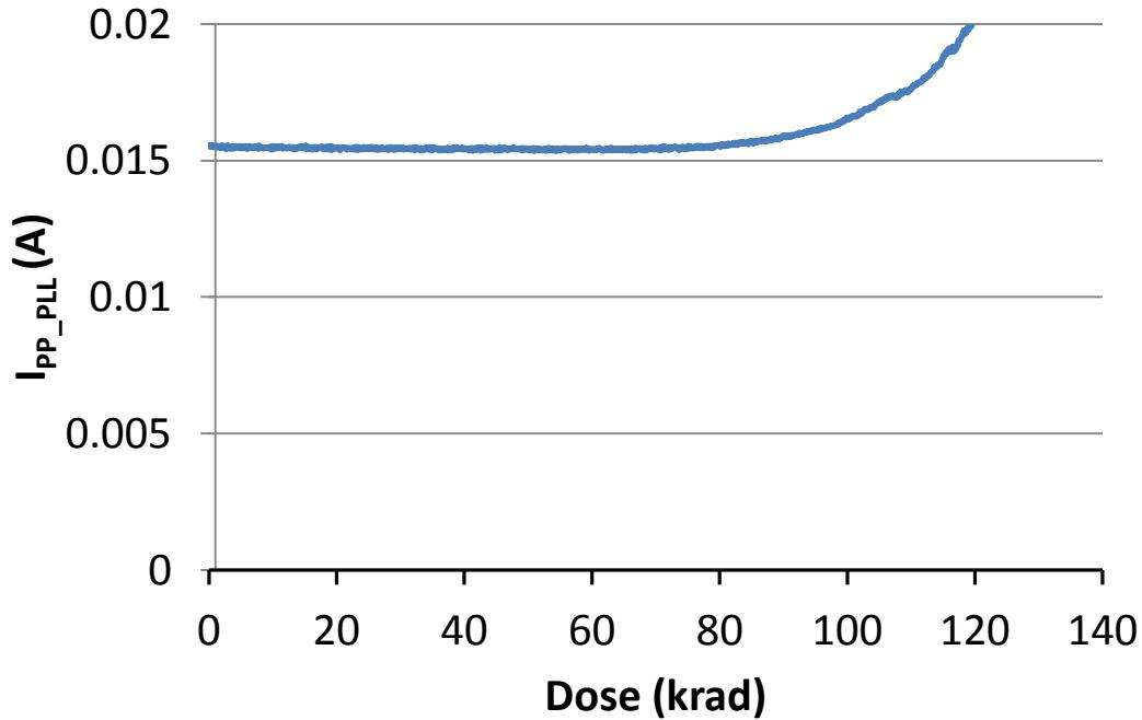
Fig. 25. DUT 1793 charge pump and PLL power supply current ( $I_{PP\_PLL}$ ) versus TID
