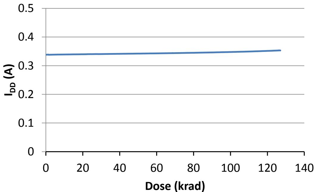
Fig. 4. DUT 1703 core power supply current ( $I_{DD}$ ) versus TID
