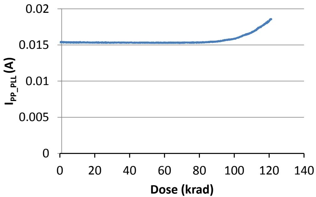
Fig. 21. DUT 1690 charge pump and PLL power supply current ( $I_{PP\_PLL}$ ) versus TID
