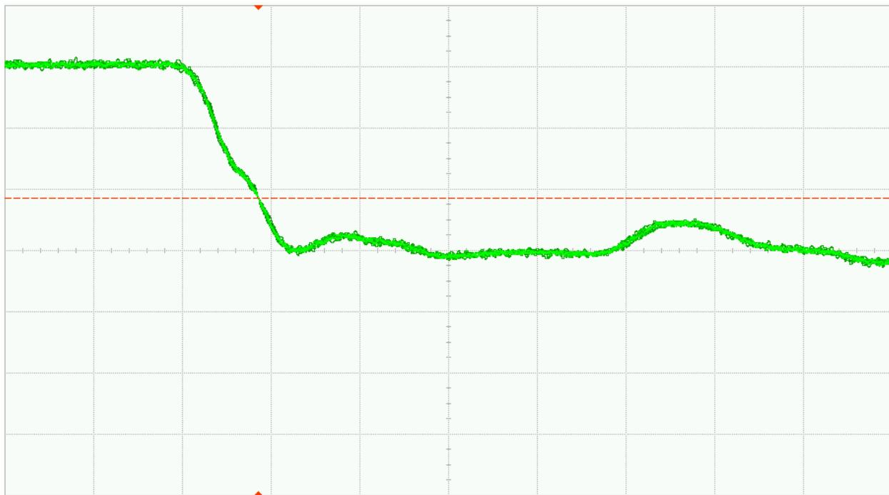
Fig. 32 (b). DUT 1658 post-annealing Falling edge, abscissa scale is 1V/div and ordinate scale is 2ns/div
