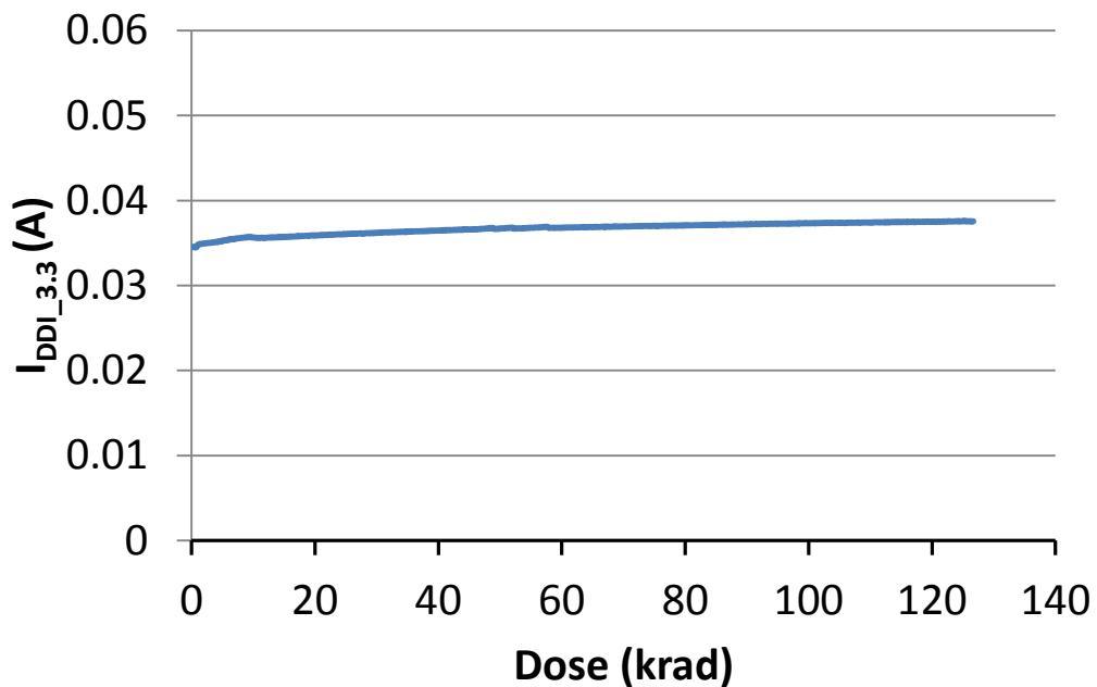
Fig. 18. DUT 1786 I/O bank 3.3V power supply current ( $I_{DDI\_3.3}$ ) versus TID
