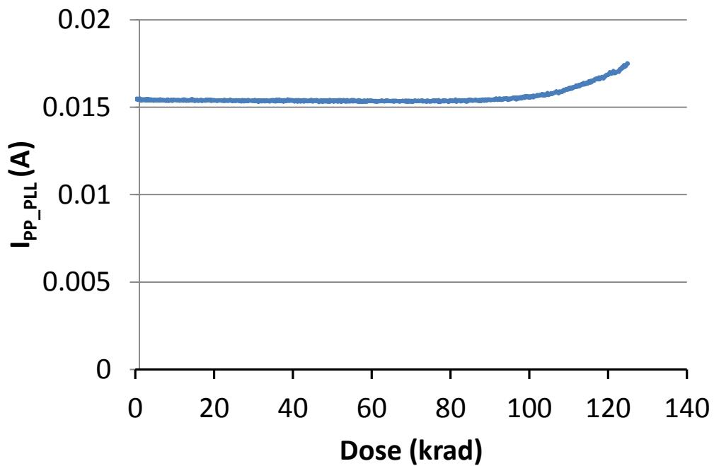
Fig. 22. DUT 1703 charge pump and PLL power supply current ( $I_{PP\_PLL}$ ) versus TID
