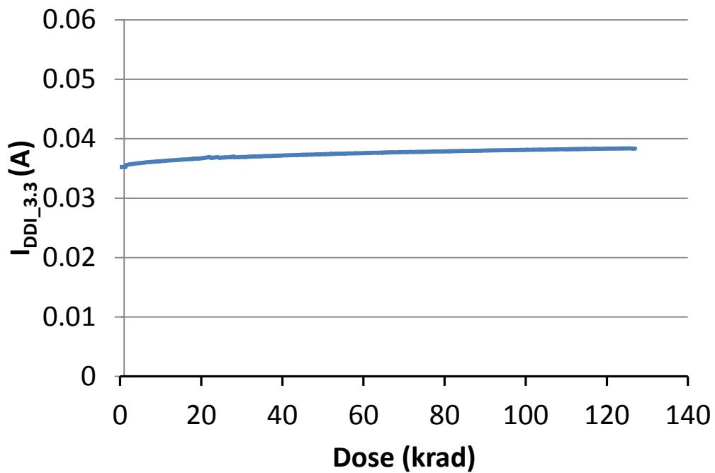
Fig. 16. DUT 1703 I/O bank 3.3V power supply current ( $I_{DDI\_3.3}$ ) versus TID
