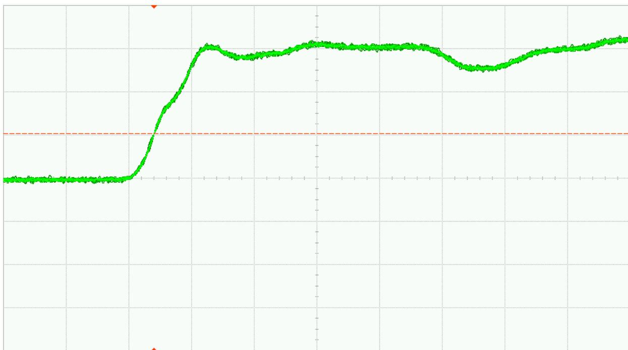
Fig. 30 (a). DUT 1786 pre-irradiation rising edge, abscissa scale is 1V/div and ordinate scale is 2ns/div
