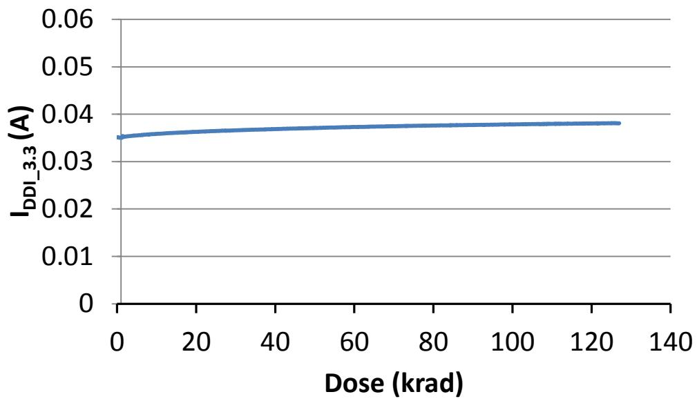
Fig. 14. DUT 1658 I/O bank 3.3V power supply current ( $I_{DDI\_3.3}$ ) versus TID
