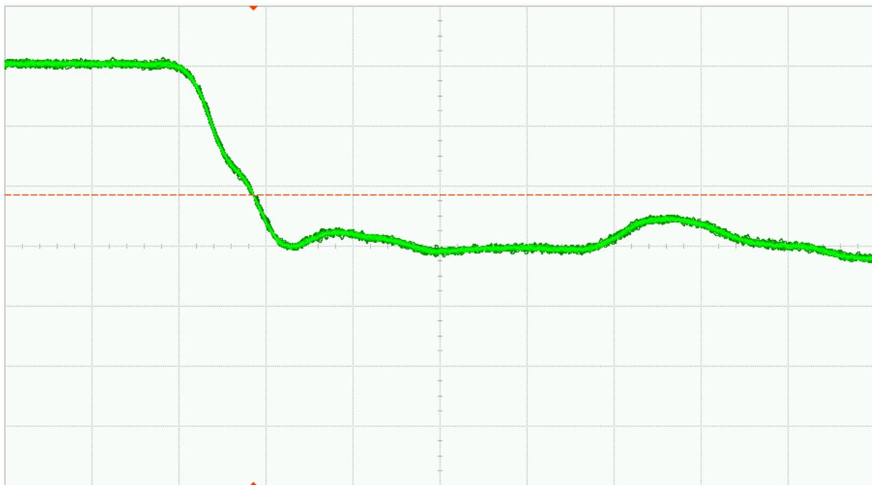
Fig. 33 (a). DUT 1690 pre-irradiation Falling edge, abscissa scale is 1V/div and ordinate scale is 2ns/div
