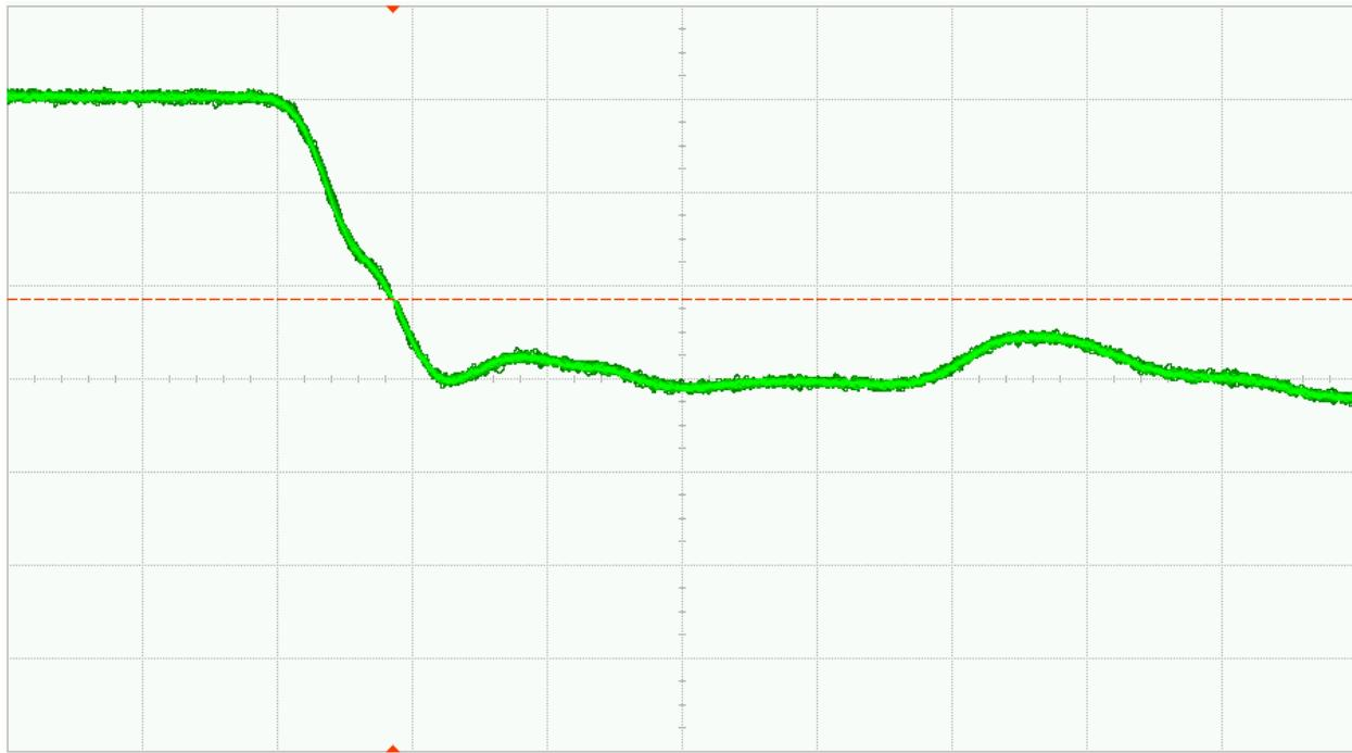
Fig. 35 (b). DUT 1744 post-annealing Falling edge, abscissa scale is 1V/div and ordinate scale is 2ns/div
