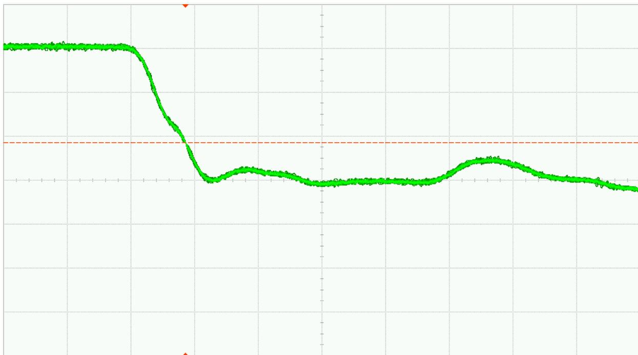
Fig. 35 (a). DUT 1744 pre-irradiation Falling edge, abscissa scale is 1V/div and ordinate scale is 2ns/div
