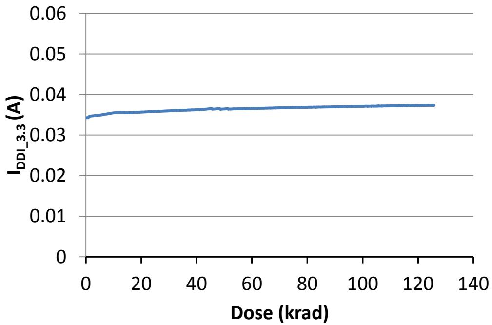
Fig. 19. DUT 1793 I/O bank 3.3V power supply current ( $I_{DDI\_3.3}$ ) versus TID
