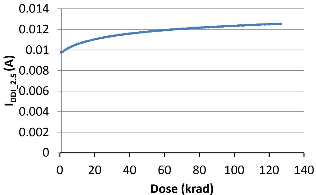
Fig. 10. DUT 1703 I/O bank 2.5V power supply current ( $I_{DDI\_2.5}$ ) versus TID
