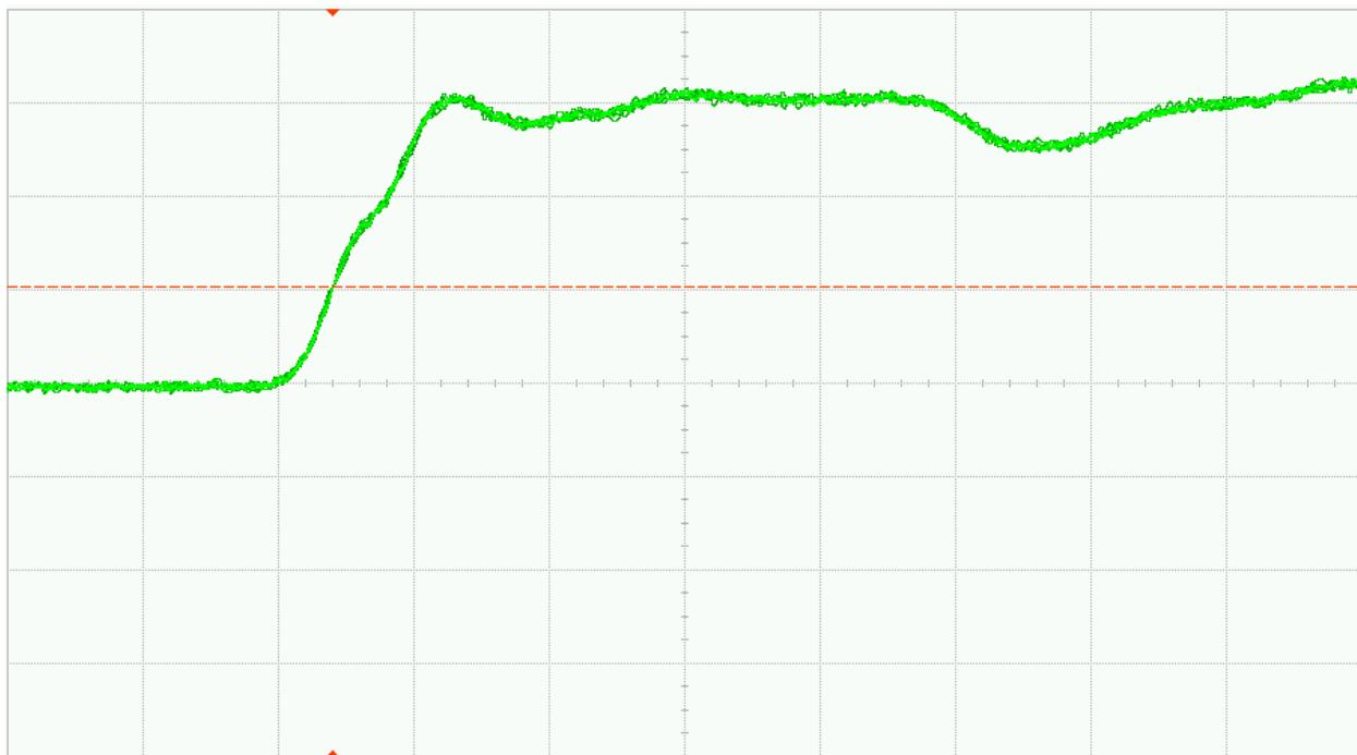
Fig. 28 (a). DUT 1703 pre-irradiation rising edge, abscissa scale is 1V/div and ordinate scale is 2ns/div
