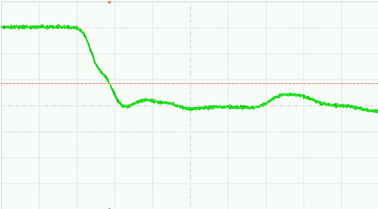
Fig. 37 (b). DUT 1793 post-annealing Falling edge, abscissa scale is 1V/div and ordinate scale is 2ns/div
