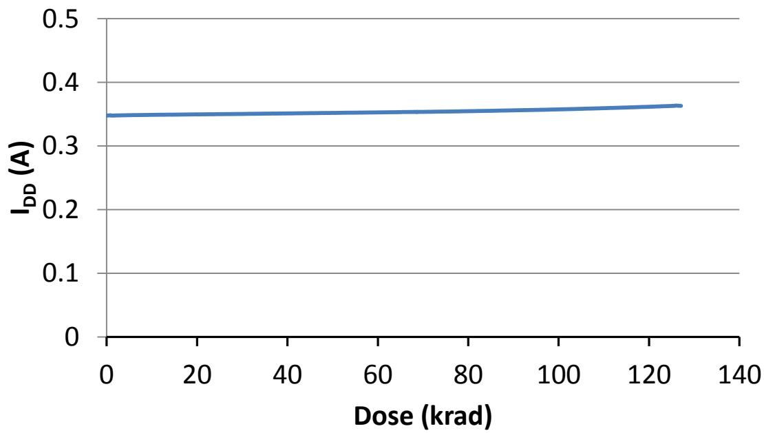
Fig. 3. DUT 1690 core power supply current ( $I_{DD}$ ) versus TID
