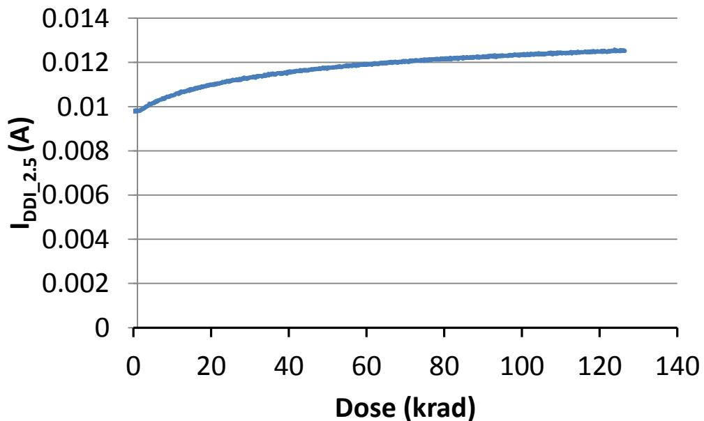
Fig. 11. DUT 1744 I/O bank 2.5V power supply current ( $I_{DDI\_2.5}$ ) versus TID
