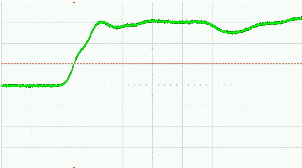
Fig. 26 (b). DUT 1658 post-annealing rising edge, abscissa scale is 1V/div and ordinate scale is 2ns/div
