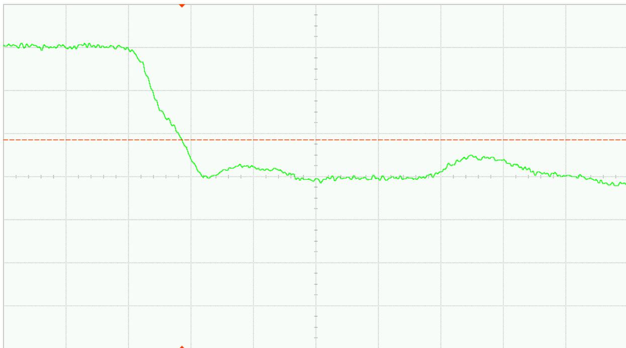
Fig. 32 (a). DUT 1758 pre-irradiation Falling edge, abscissa scale is 1V/div and ordinate scale is 2ns/div
