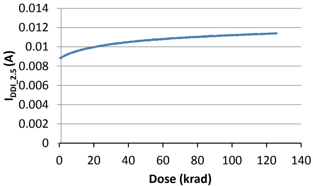
Fig. 13. DUT 1793 I/O bank 2.5V power supply current ( $I_{DDI\_2.5}$ ) versus TID
