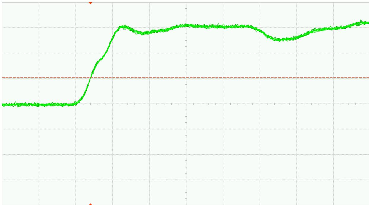
Fig. 31 (b). DUT 1793 post-annealing rising edge, abscissa scale is 1V/div and ordinate scale is 2ns/div
