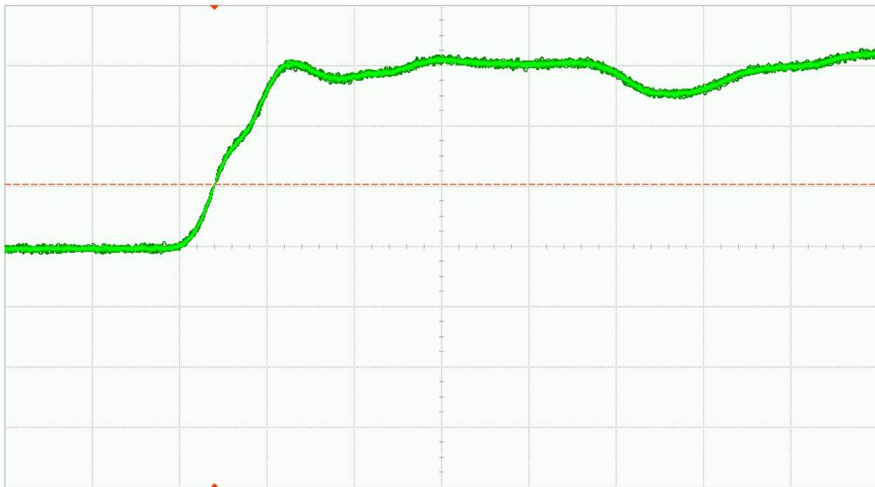
Fig. 28 (b). DUT 1703 post-annealing rising edge, abscissa scale is 1V/div and ordinate scale is 2ns/div
