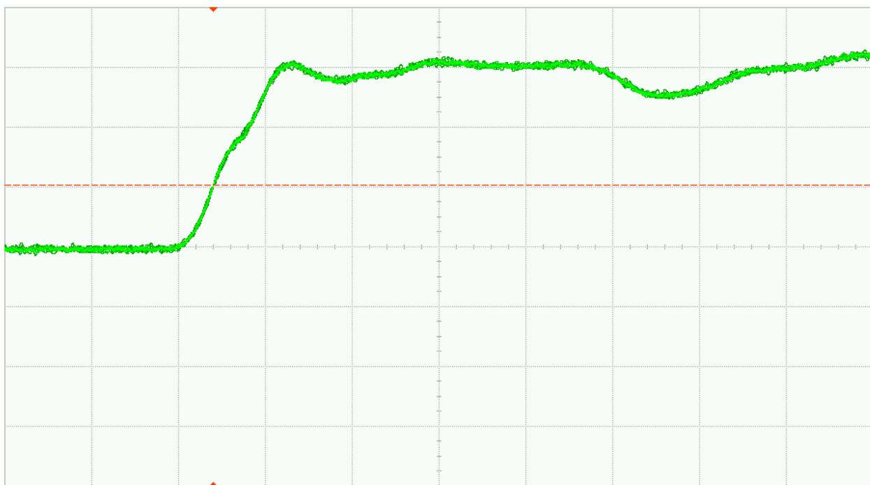
Fig. 31 (a). DUT 1793 pre-irradiation rising edge, abscissa scale is 1V/div and ordinate scale is 2ns/div
