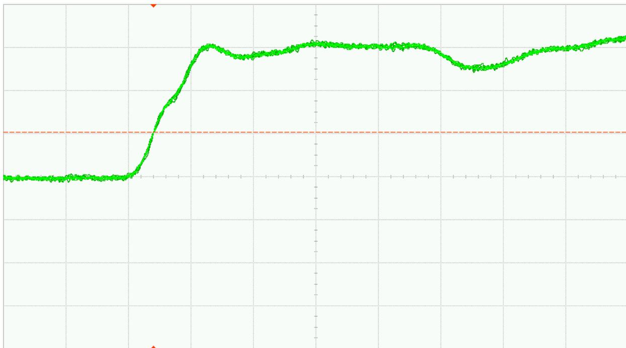
Fig. 27 (a). DUT 1690 pre-irradiation rising edge, abscissa scale is 1V/div and ordinate scale is 2ns/div
