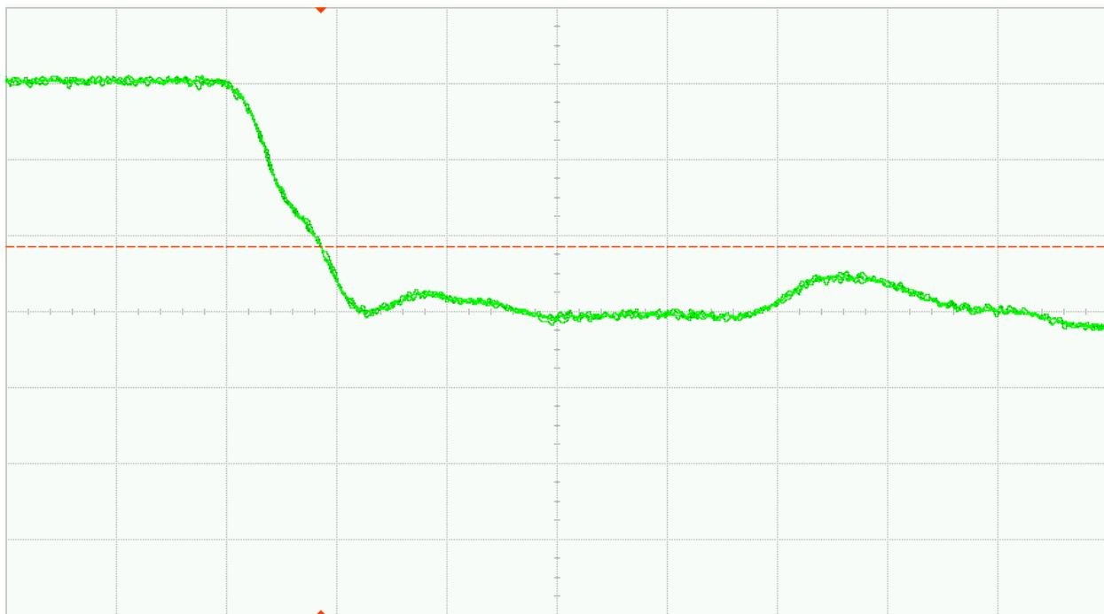
Fig. 34 (a). DUT 1703 pre-irradiation Falling edge, abscissa scale is 1V/div and ordinate scale is 2ns/div
