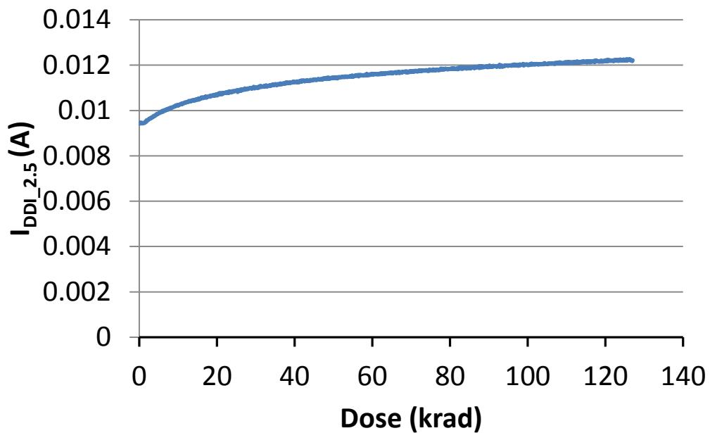
Fig. 8. DUT 1658 I/O bank 2.5V power supply current ( $I_{DDI\_2.5}$ ) versus TID
