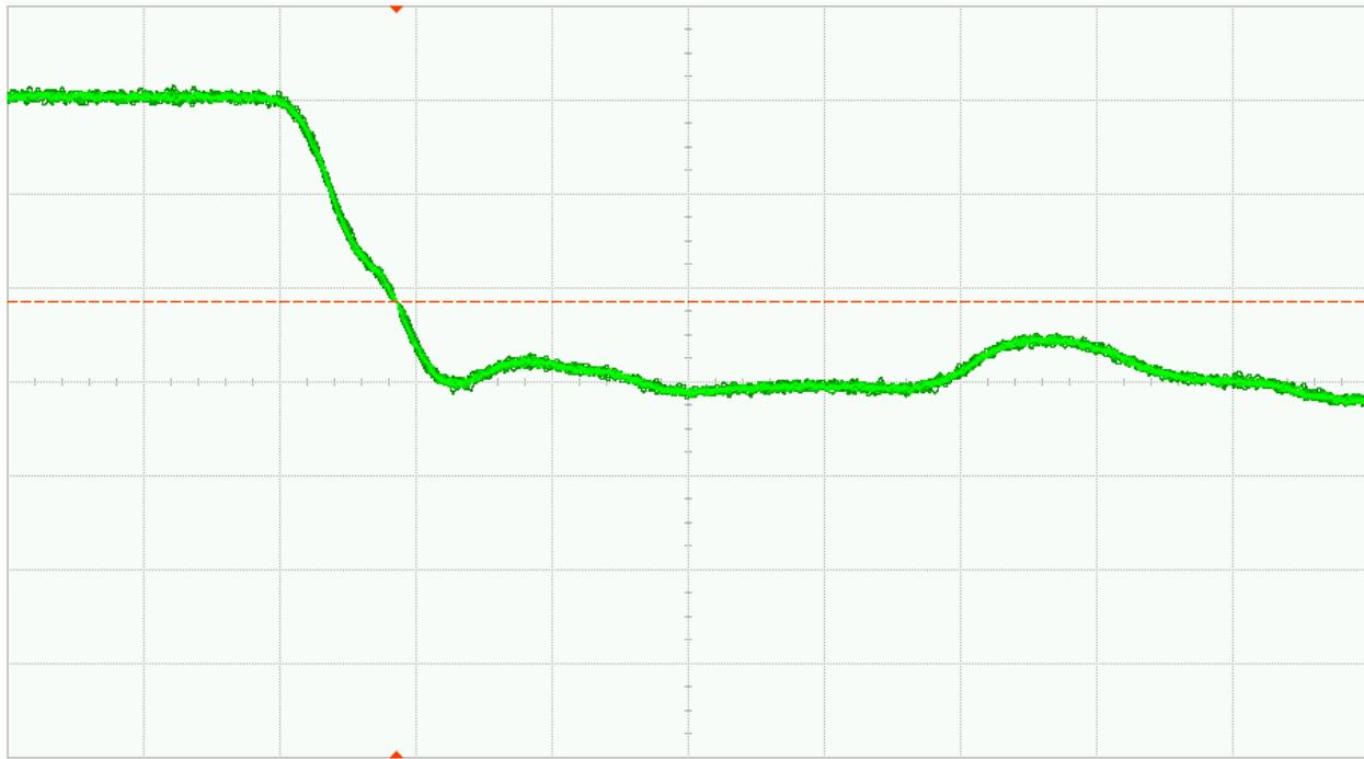
Fig. 33 (b). DUT 1690 post-annealing Falling edge, abscissa scale is 1V/div and ordinate scale is 2ns/div
