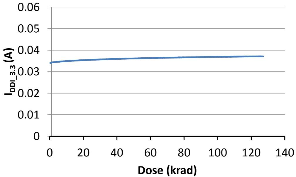
Fig. 15. DUT 1690 I/O bank 3.3V power supply current ( $I_{DDI\_3.3}$ ) versus TID
