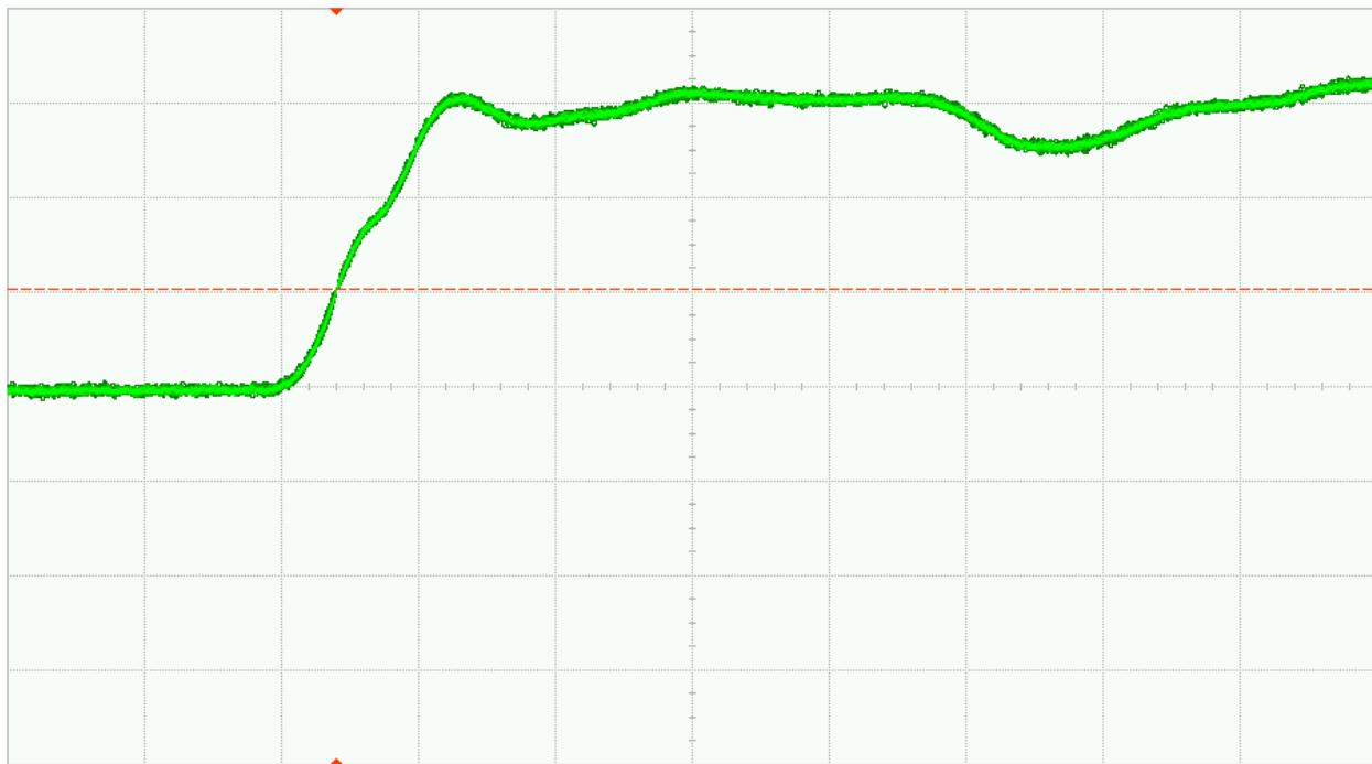
Fig. 30 (b). DUT 1786 post-annealing rising edge, abscissa scale is 1V/div and ordinate scale is 2ns/div
