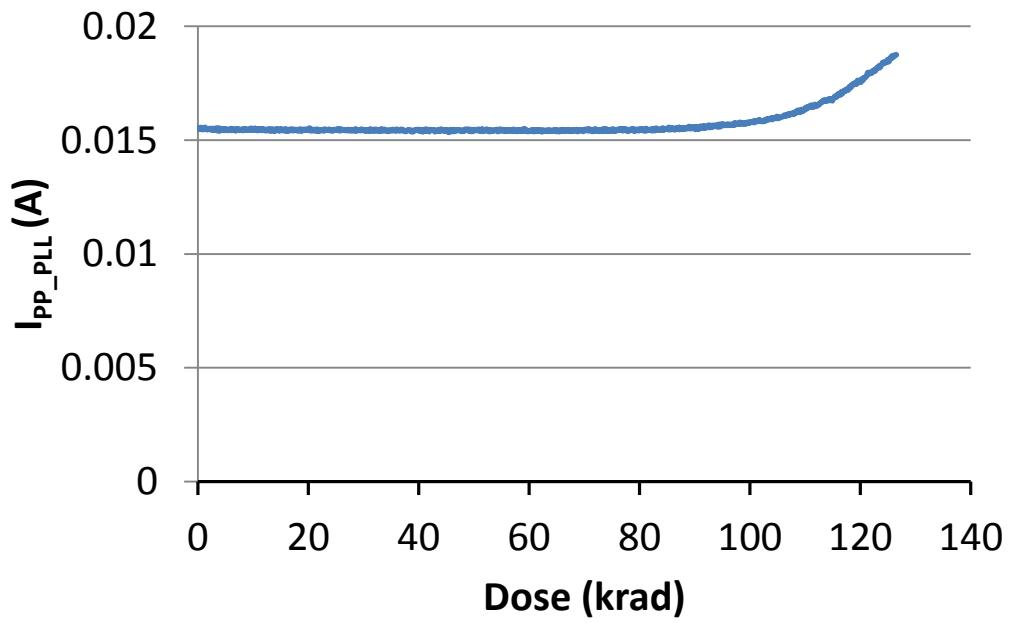
Fig. 23. DUT 1744 charge pump and PLL power supply current ( $I_{PP\_PLL}$ ) versus TID
