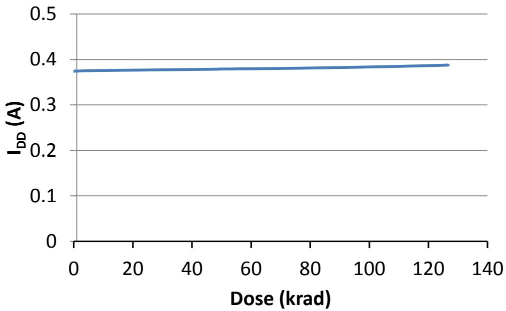
Fig. 6. DUT 1786 core power supply current ( $I_{DD}$ ) versus TID
