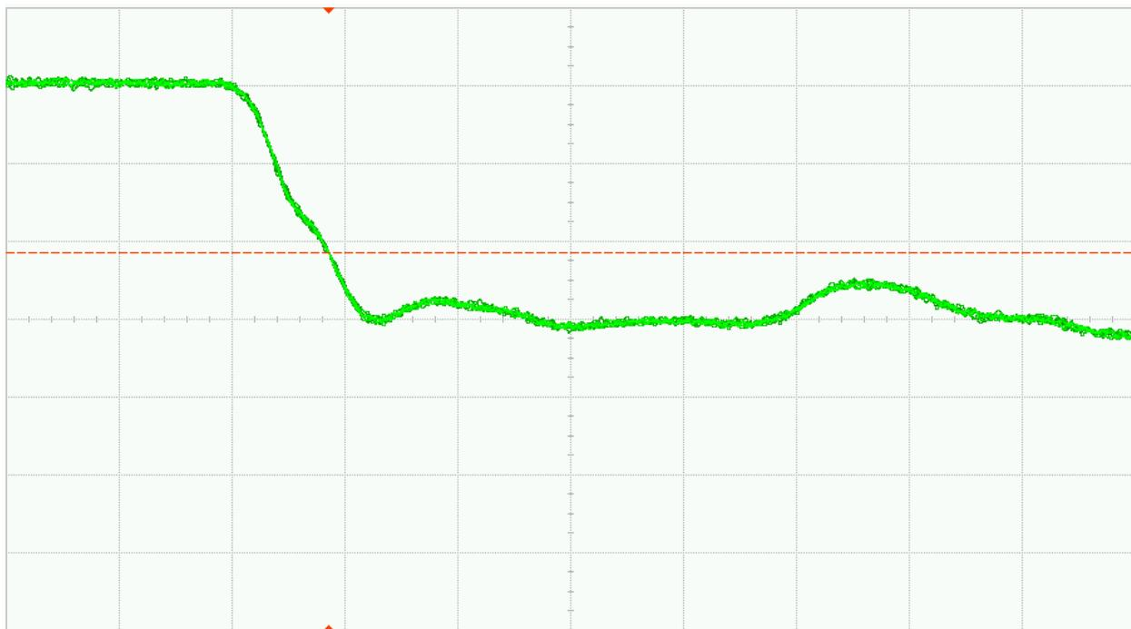
Fig. 37 (a). DUT 1793 pre-irradiation Falling edge, abscissa scale is 1V/div and ordinate scale is 2ns/div
