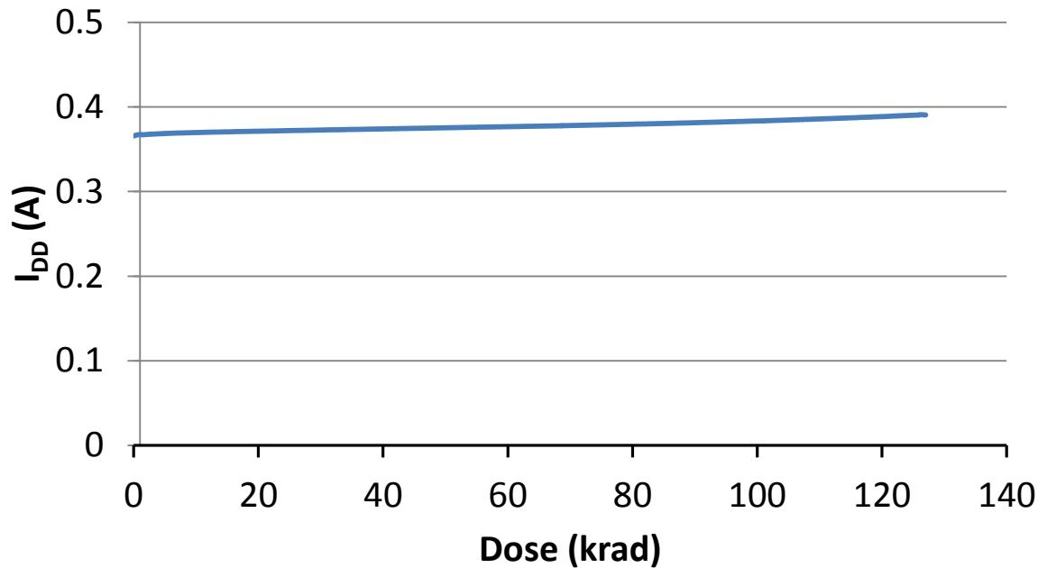
Fig. 2. DUT 1658 core power supply current ( $I_{DD}$ ) versus TID
