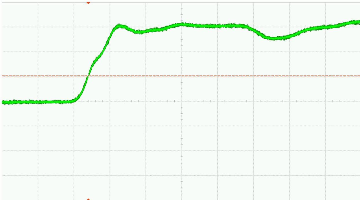
Fig. 27 (b). DUT 1690 post-annealing rising edge, abscissa scale is 1V/div and ordinate scale is 2ns/div
