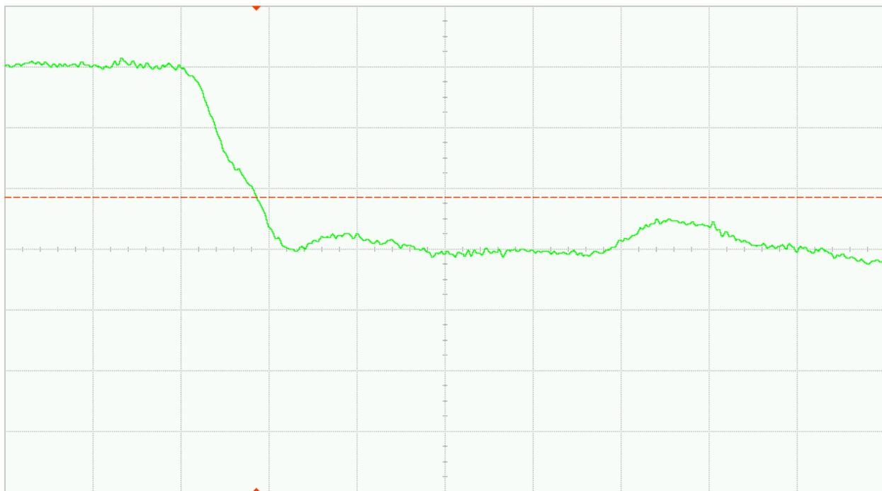
Fig. 36 (a). DUT 1786 pre-irradiation Falling edge, abscissa scale is 1V/div and ordinate scale is 2ns/div
