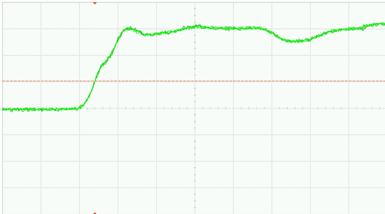
Fig. 26 (a). DUT 1658 pre-irradiation rising edge, abscissa scale is 1V/div and ordinate scale is 2ns/div
