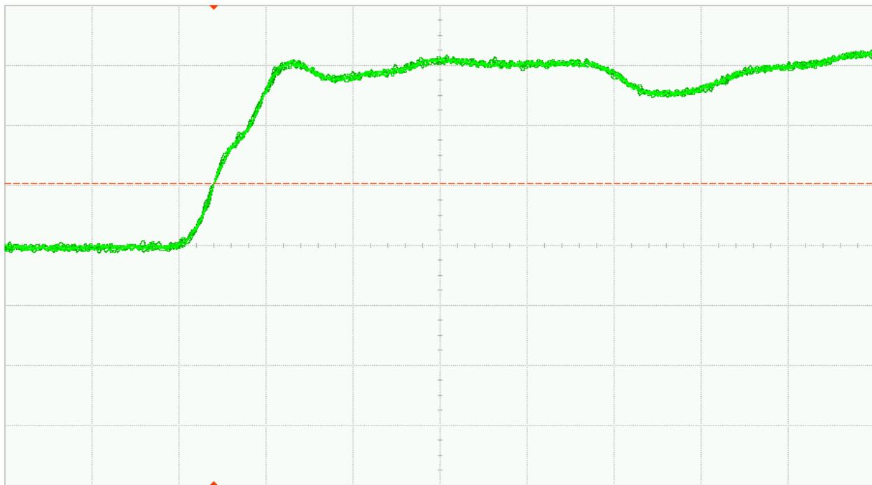
Fig. 29 (b). DUT 1744 post-annealing rising edge, abscissa scale is 1V/div and ordinate scale is 2ns/div
