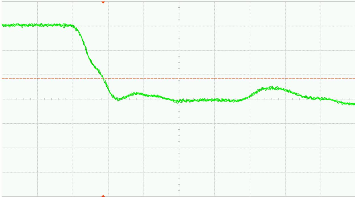
Fig. 34 (b). DUT 1703 post-annealing Falling edge, abscissa scale is 1V/div and ordinate scale is 2ns/div
