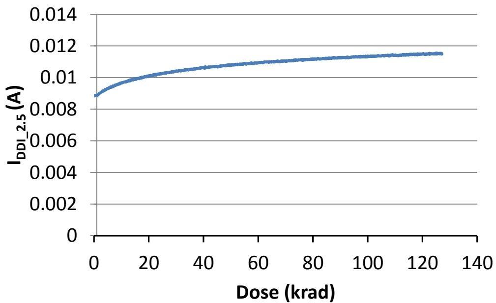
Fig. 9. DUT 1690 I/O bank 2.5V power supply current ( $I_{DDI\_2.5}$ ) versus TID
