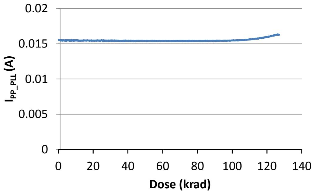
Fig. 20. DUT 1658 charge pump and PLL power supply current ( $I_{PP\_PLL}$ ) versus TID
