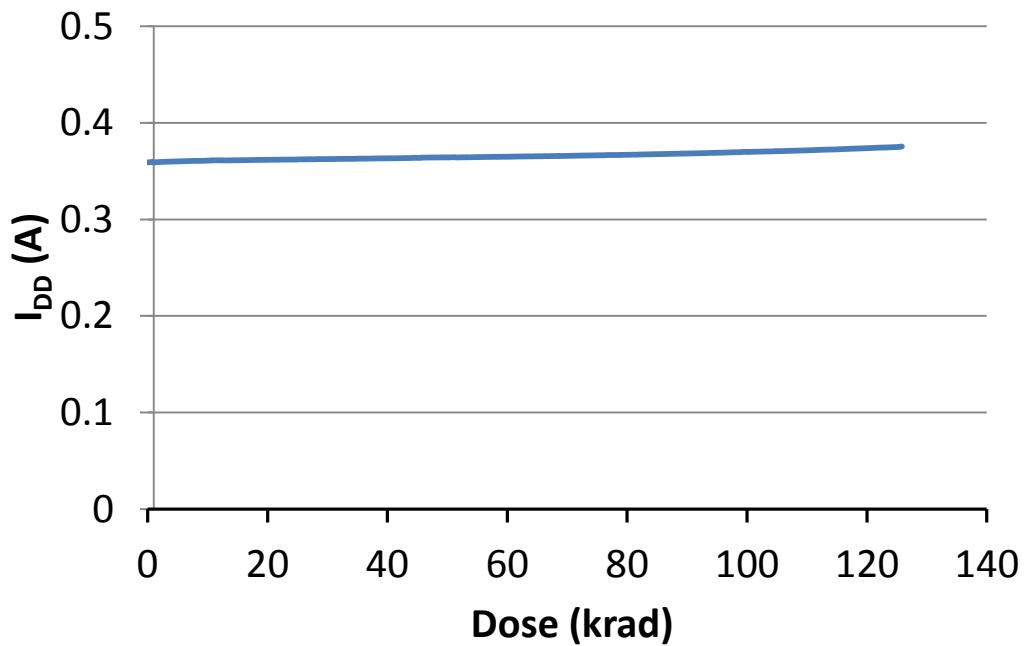
Fig. 7. DUT 1793 core power supply current ( $I_{DD}$ ) versus TID
