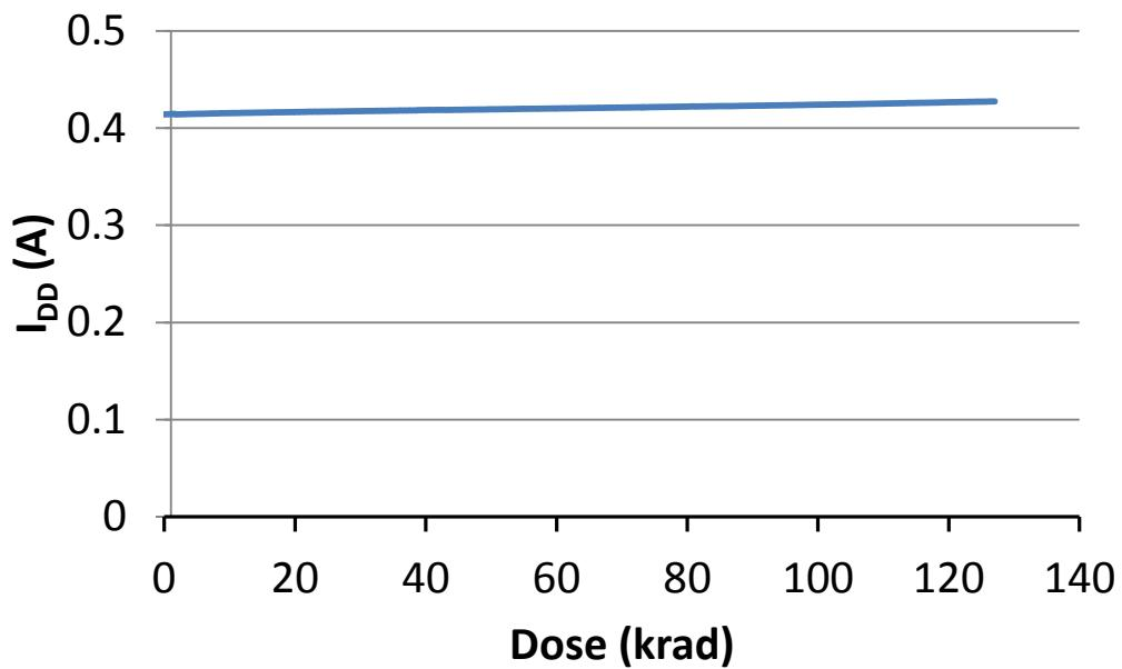
Fig. 5. DUT 1744 core power supply current ( $I_{DD}$ ) versus TID
