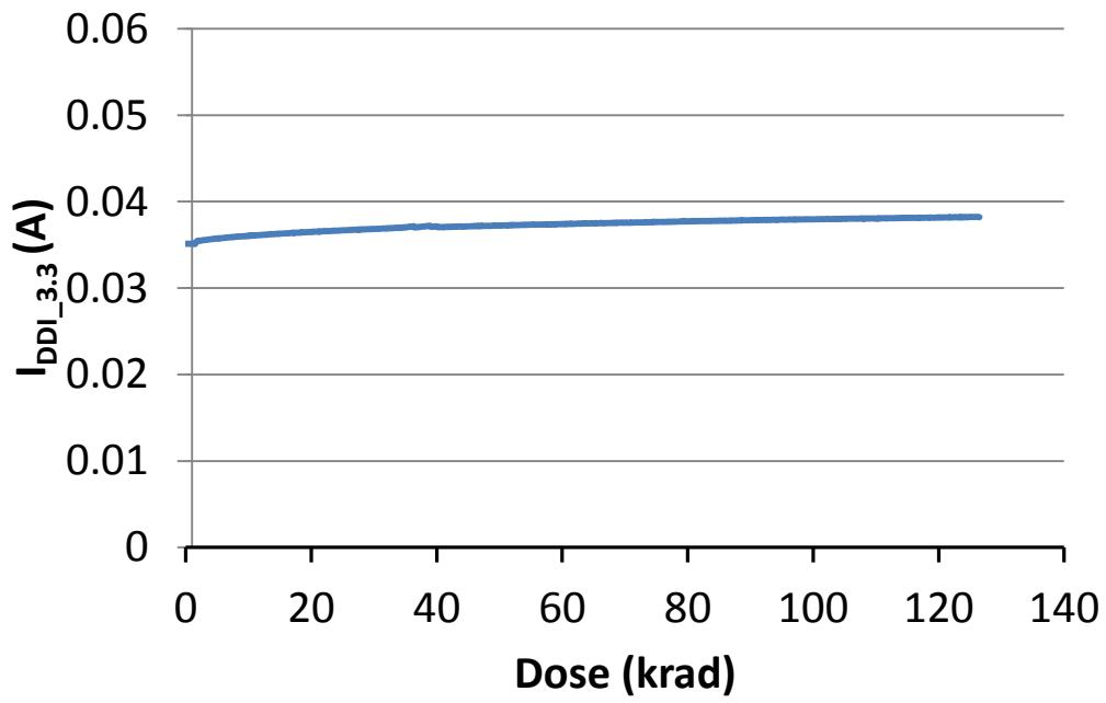
Fig. 17. DUT 1744 I/O bank 3.3V power supply current ( $I_{DDI\_3.3}$ ) versus TID
