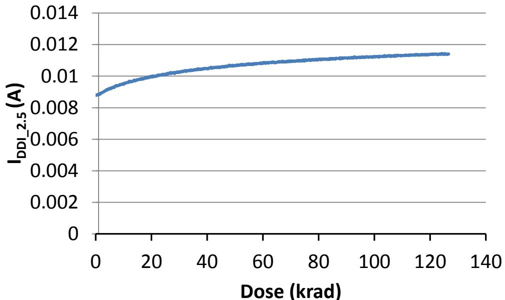
Fig. 12. DUT 1786 I/O bank 2.5V power supply current ( $I_{DDI\_2.5}$ ) versus TID
