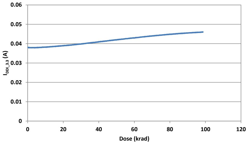
Fig. 13. DUT 9793 I/O bank 3.3V power supply current ( $I_{DD1\_3.3}$ ) versus TID
