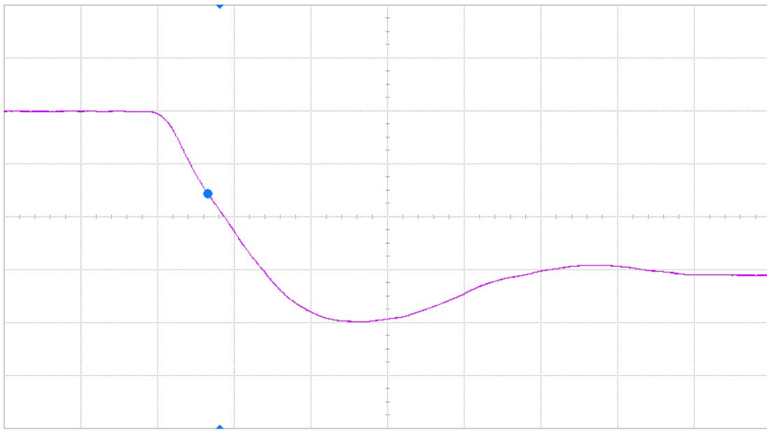
Fig. 24 (a). DUT 9741 pre-irradiation Falling edge, abscissa scale is 1V/div and ordinate scale is 2ns/div
