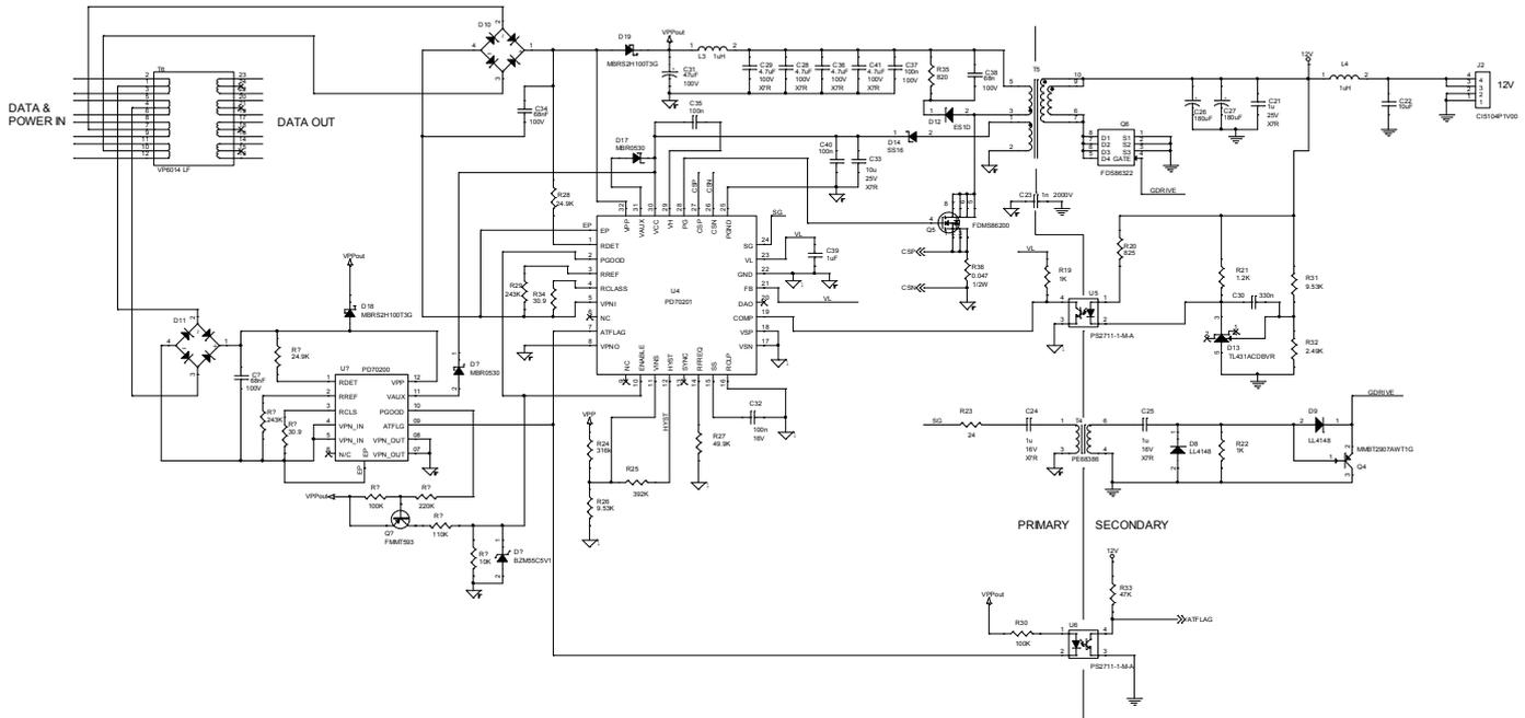
Figure 4: Typical 4 pairs configuration with a PD70200 and PD70201; shows use of ENABLE pin
