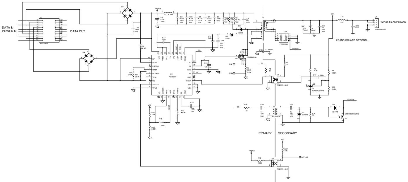
**Figure 3. Typical 2 or 4 Pair Configuration with a Single PD70201 IC.**
