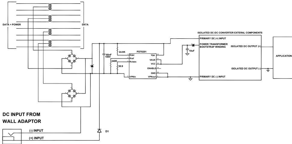
**CONFIGURATION #1: SOURCE CONNECTED TO PD70201 INPUT**
