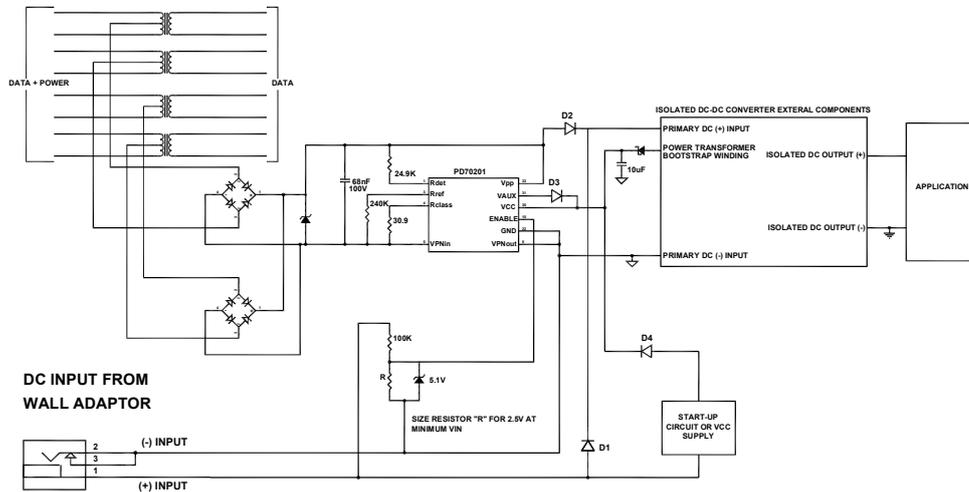
**CONFIGURATION #2: SOURCE CONNECTED TO PD70201 DC-DC CONVERTER**
