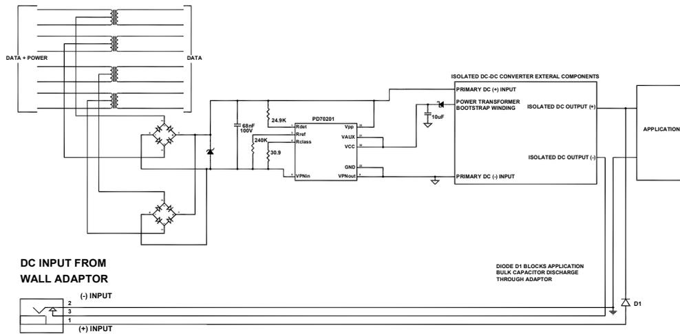
**CONFIGURATION #3: SOURCE CONNECTED TO APPLICATION'S SUPPLY RAILS**
