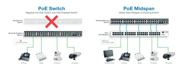
Fig. 3: Midspans offer a variety of advantages over switches for PoE deployment.
