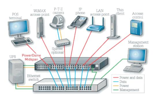
Fig. 1: PoE midspans are installed between the network switch and PDs.
