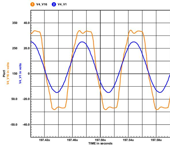
**Figure 26** Drain and Gate Wave Forms N-P HB
