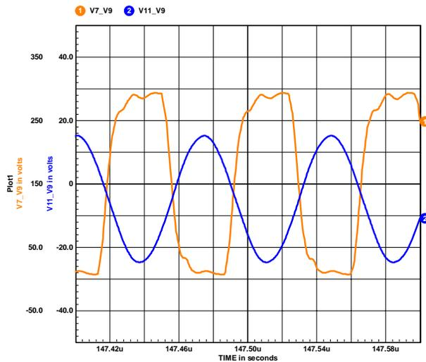
**Figure 20** Drain Wave Forms N-N Low Side
