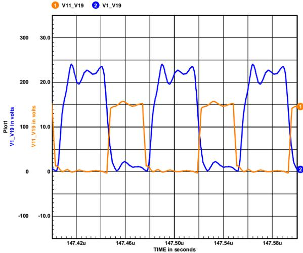
**Figure 6** Drain and Gate Wave Forms N-N HB
