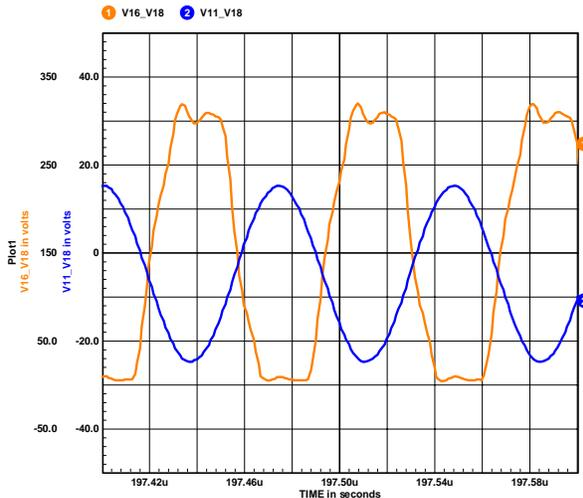
**Figure 27** Drain Wave Forms N-N Low Side
