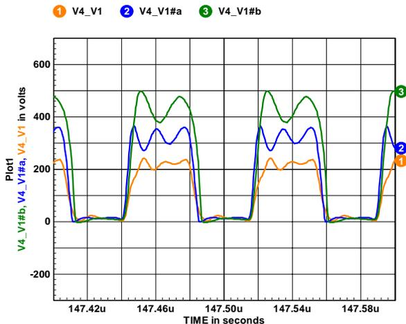
**Figure 7** Drain Wave Forms with L2, L3 and L6 Variations
