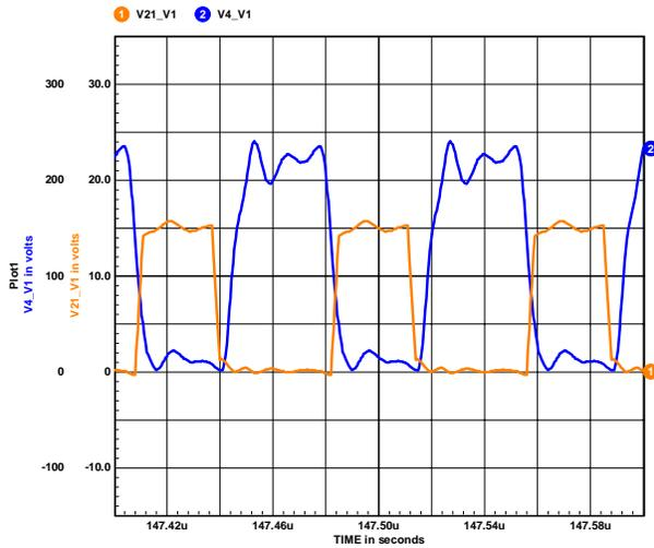
**Figure 5** Drain and Gate Wave Forms N-N HB
