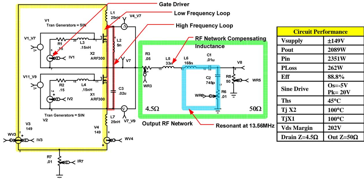
Figure 15 N-N Channel Half Bridge
