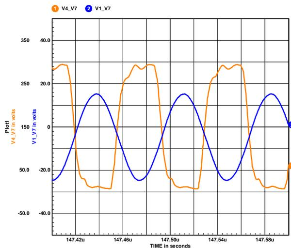
**Figure 19** Drain and Gate Wave Forms N-N HB
