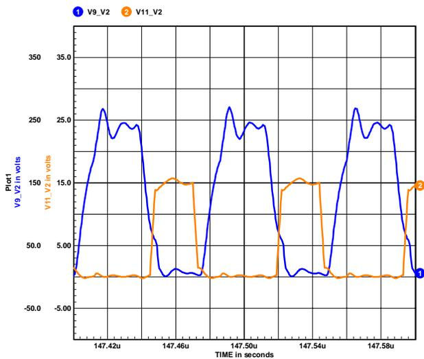
**Figure 13** Drain Wave Forms N-P Low Side
