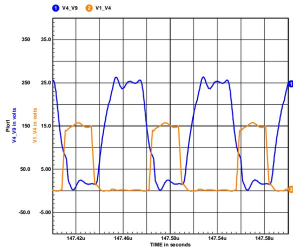
**Figure 12** Drain and Gate Wave Forms N-P HB
