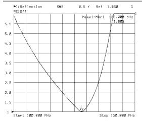
Figure 2 Input VSWR vs Frequency
