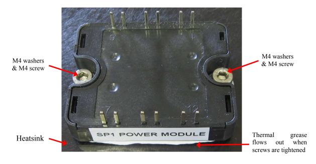
Fig 1: Proper application of thermal grease to the power module.
