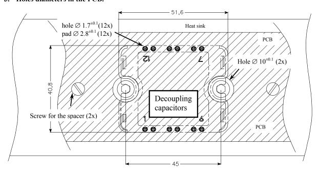
Fig 4: Pad and hole diameters (in millimeters) for a phase leg configuration.
