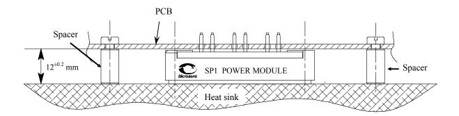
Fig 3: PCB onto the power module.
