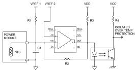
Fig 2: Example of NTC thermistor comparator circuit
