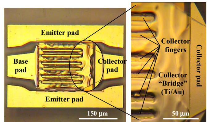
Fig. 2. Micrographs of a 4-finger RF BJT with front-collector-“bridge” contacts and on-wafer RF pad layout.
