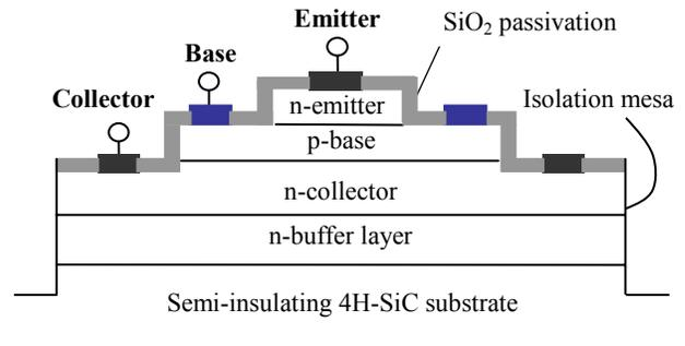
Fig. 1. The schematic cross-sectional structure of a 4H-SiC BJT on a semi-insulating substrate.
