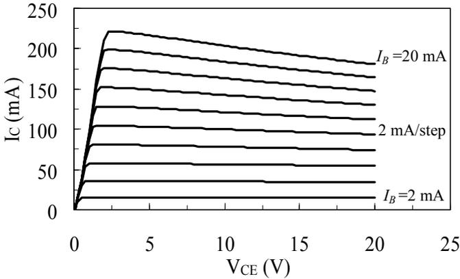
Fig. 3.  $I$ - $V$  characteristics of a 4-finger RF transistor.  $I_B = 2, 4, \dots, 18$  and 20 mA.
