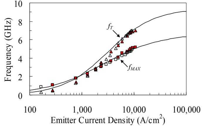
Fig. 5.  $f_T$  and  $f_{MAX}$  extrapolated from s-parameter measurements at different  $J_E$  for two 4-finger RF transistors (open and filled symbols) at two different locations on the wafer. Solid lines represent the calculated values of  $f_T$  and  $f_{MAX}$  using the transit-time model.
