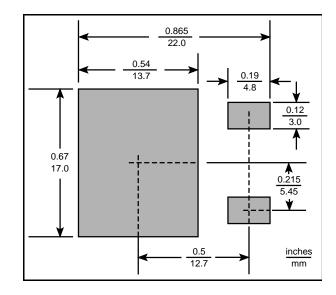
**Figure 1.** Minimum Recommended Footprint for the D<sup>3</sup>PAK.
