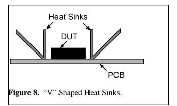
It should be noted that the D<sup>3</sup>PAK mounted to a PCB in still air, even with heat sinks attached, is incapable of matching the thermal performance of an unmounted device is still air! The reason for this is the backside of the device is copper and having it exposed directly to air is better than covering it with a PC board. Therefore, it would seem that a device mounted vertically on the PC board would be a more efficient use of the device.
