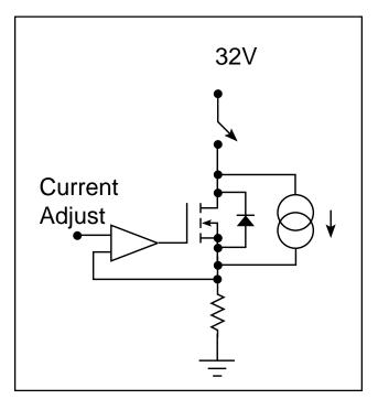
Figure 3. Simplified Test Setup Schematic.
