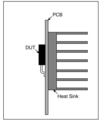
Figure 5. PCB With Heat Sink.
