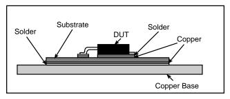
**Figure 9.** Cross Section of the D<sup>3</sup>PAK Mounted on the Substrate and Copper Base.
