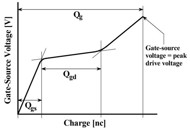
Figure 3.  $v_{GS}$  as a function of gate charge
