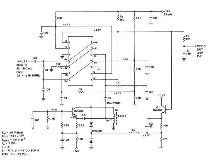
Figure 19 shows the excellent results obtained. If desired, the linearity can be improved further by adding a potentiometer to the 120 ohm resistor on pins 3 and 9 of the CA3102E to adjust the center tuning voltage of the KV2001.
