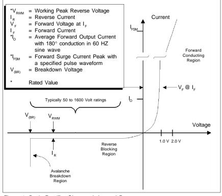
Figure 1: Basic Rectifier Characteristics and Parameters
