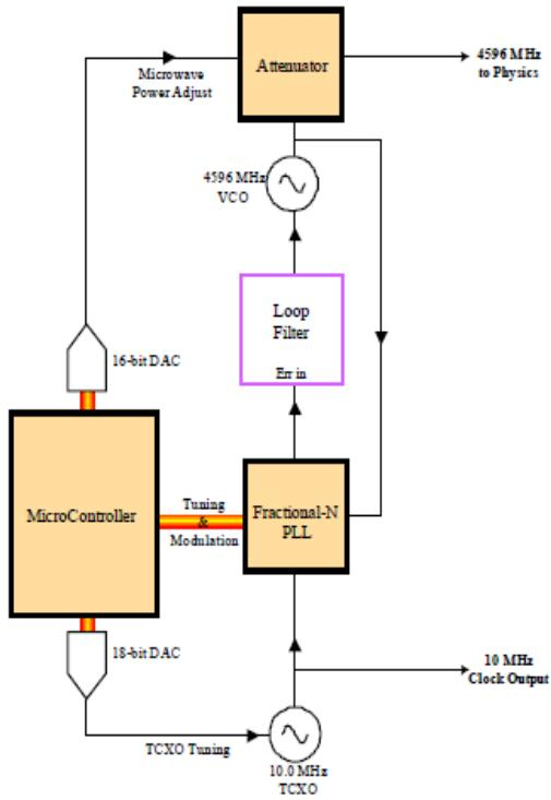
Figure 3: CSAC Microwave Subsystem
