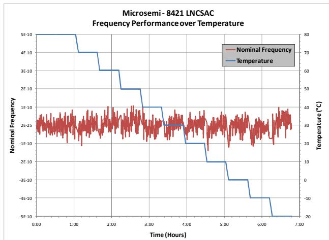
**Figure 6: LNCSAC Frequency vs Temperature**
