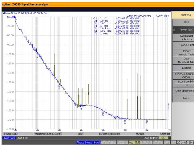
Figure 8: 100 MHz LNCSAC Phase Noise
