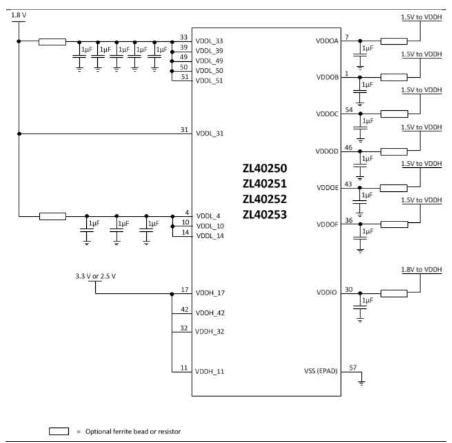
Figure 1 Example ZL40250 – ZL40253 Power Supply Decoupling Scheme Using Power Islands
