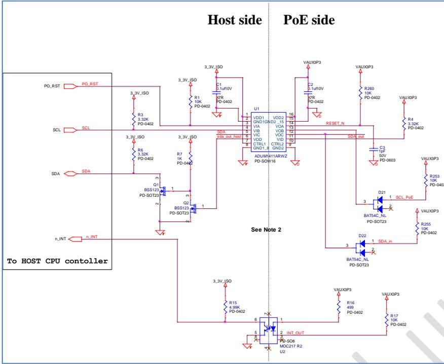
**Figure 7: Digital Isolator + interrupt isolator**
