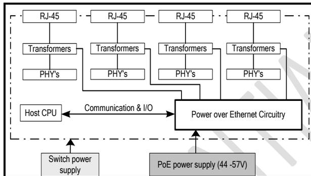
Figure 17: Block Diagram - PoE Circuitry Inside the Switch
