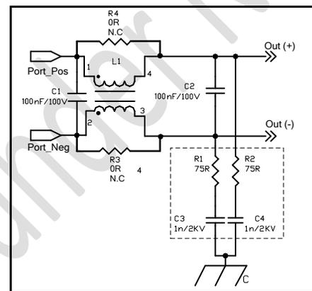
Figure 13: Recommended EMI Filter
