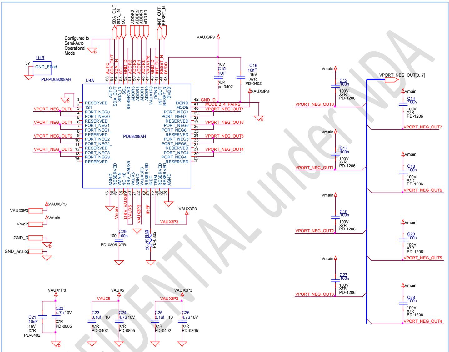
Figure 6: PD69208AH Circuitry for PoE Manager #0 (6 PL)
