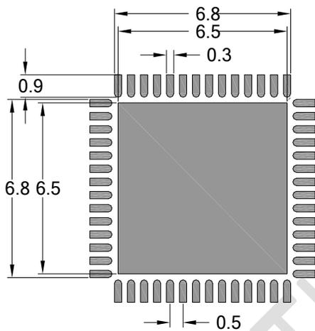
Figure 22: Thermal Pad Array Footprint (CS)
