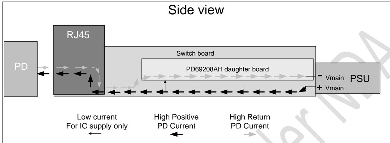
Figure 16: Component Identification for PD69208AH Circuitry
