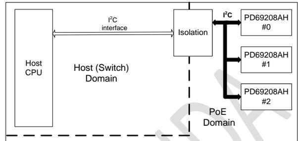
Figure 2: 12-port Configuration block diagram
