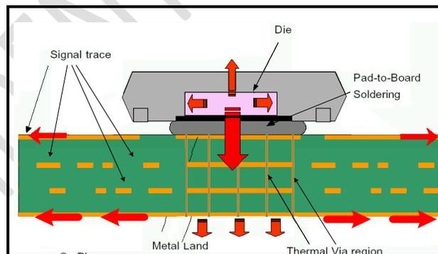
Figure 21: Heat Dissipation in PC
