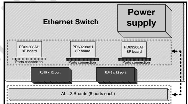
Figure 18: PoE DB Circuitry Inside the Switch
