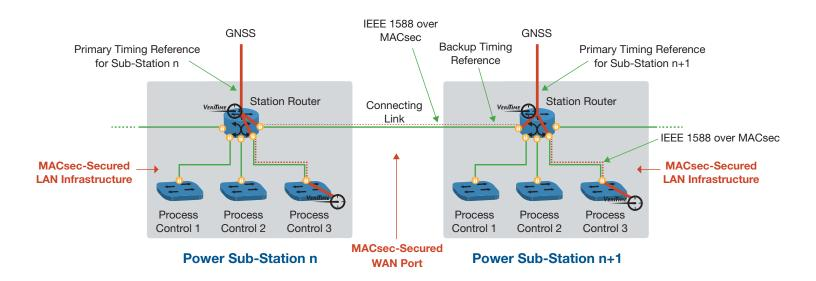
Figure 1. Using PTP over MACsec in a power sub-station application
