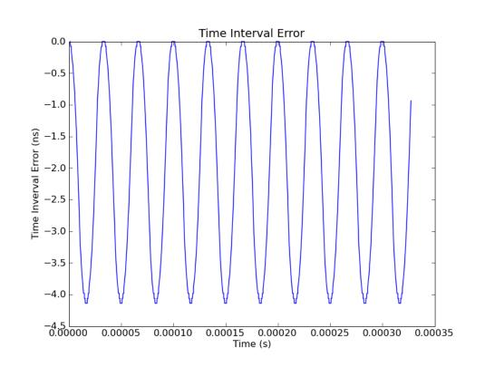
Figure 4 · Time Interval Error of Modulated Signal vs Un-modulated Square Wave
