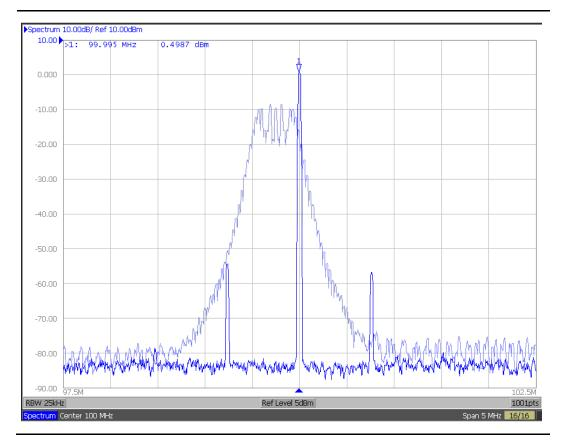
Figure 3 · Unmodulated and Spread Spectrum Signals Superimposed
