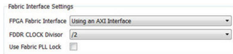
Figure 1-3 • Fabric Interface Settings - AXI Interface and FDDR Clock Divisor Agreement
