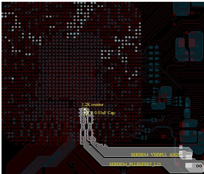
Figure 21 • Layout of SERDES_4_L23_VDDAPLL and SERDES_4_L23_REFRET
