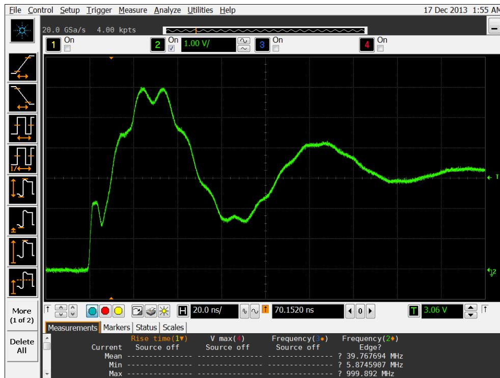
Figure 9a DUT 12287 Pre-Irradiation Rising Edge
