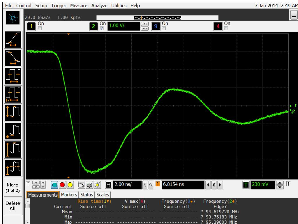
Figure 20b DUT 12350 Post-Annealing Falling Edge
