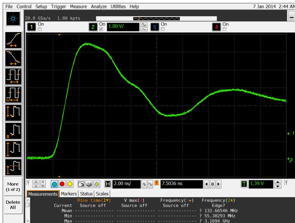
Figure 9b DUT 12287 Post-Annealing Rising Edge
