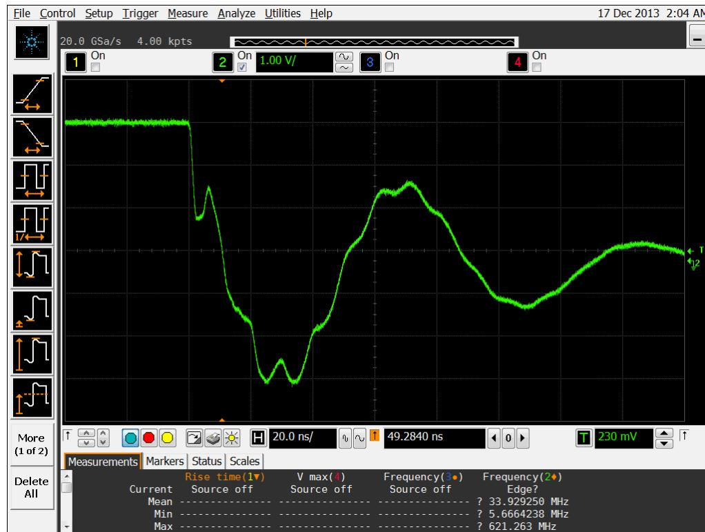
Figure 16a DUT 12310 Pre-Irradiation Falling Edge
