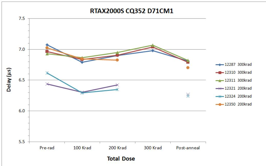
**Figure 8 In-Situ Propagation Delay Versus Total Dose.**
