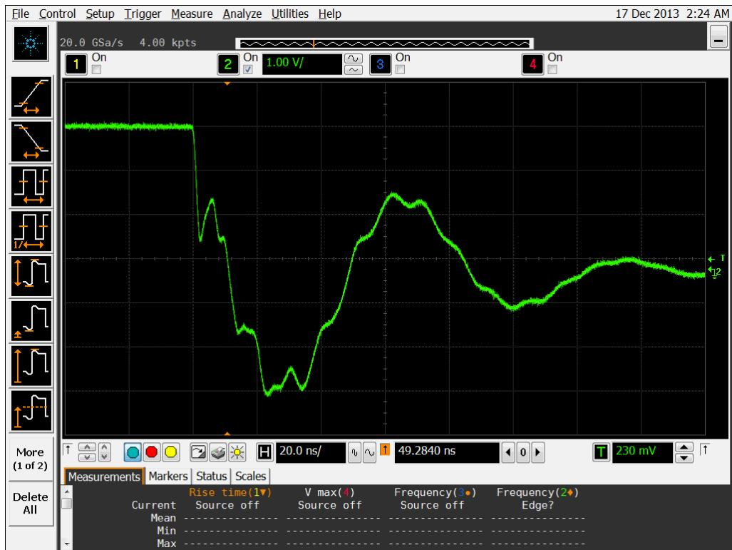
Figure 19a DUT 12324 Pre-Irradiation Falling Edge
