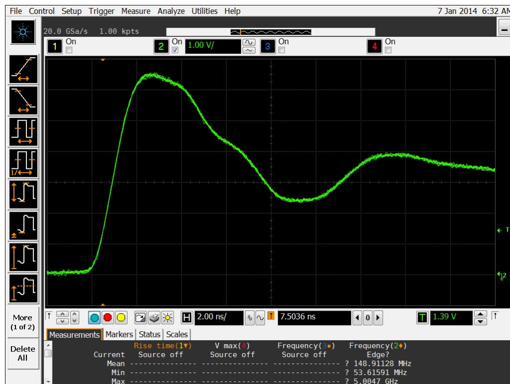
Figure 12b DUT 12321 Post-Annealing Rising Edge
