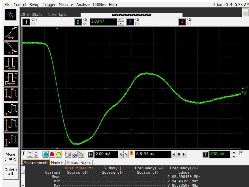
Figure 18b DUT 12321 Post-Annealing Falling Edge
