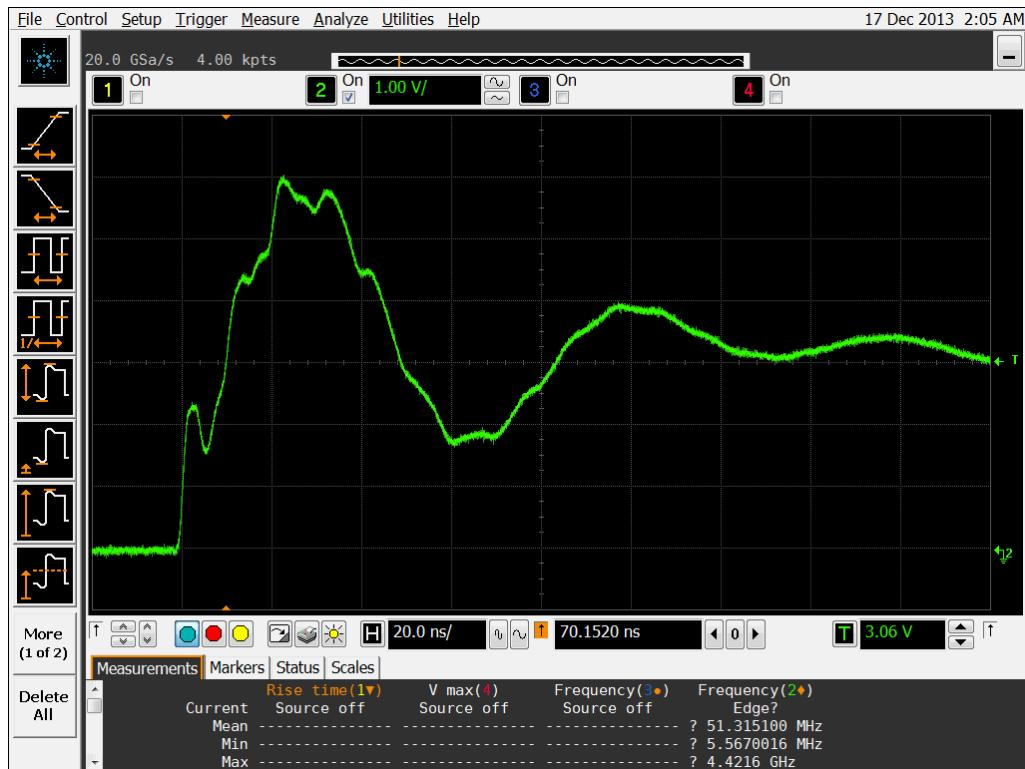
Figure 10a DUT 12310 Pre-Irradiation Rising Edge
