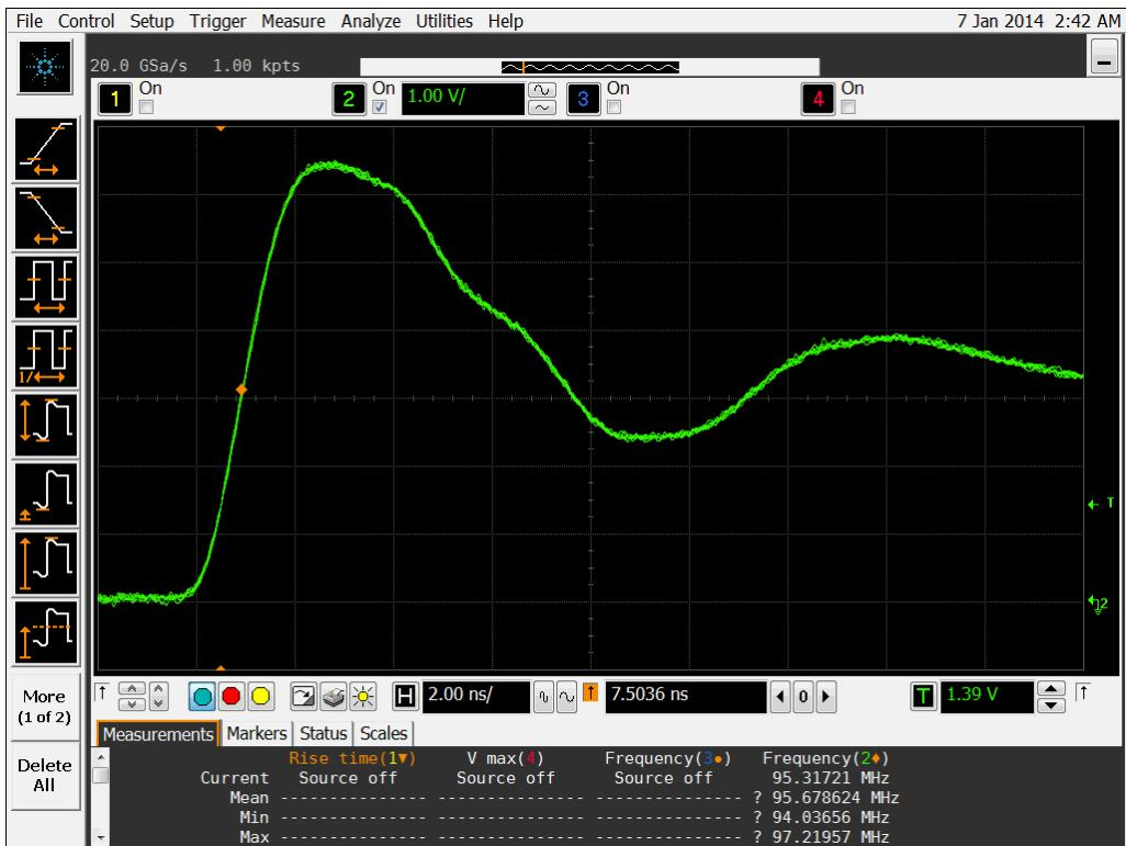
Figure 13b DUT 12324 Post-Annealing Rising Edge
