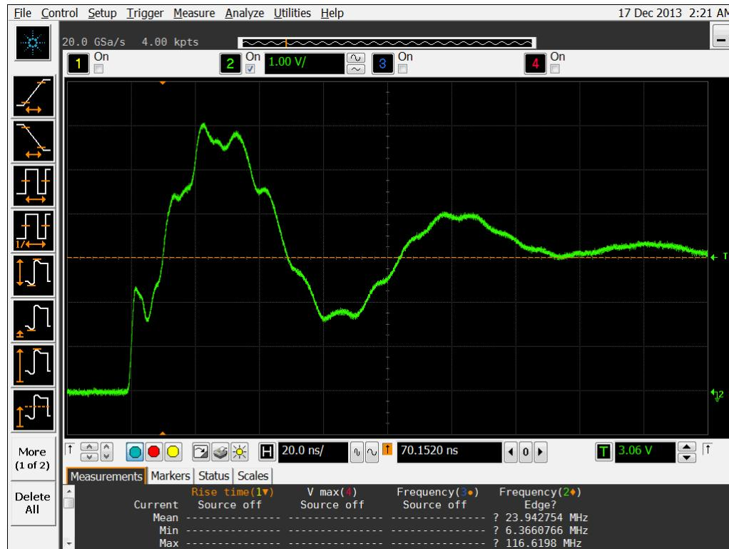
Figure 12a DUT 12321 Pre-Irradiation Rising Edge
