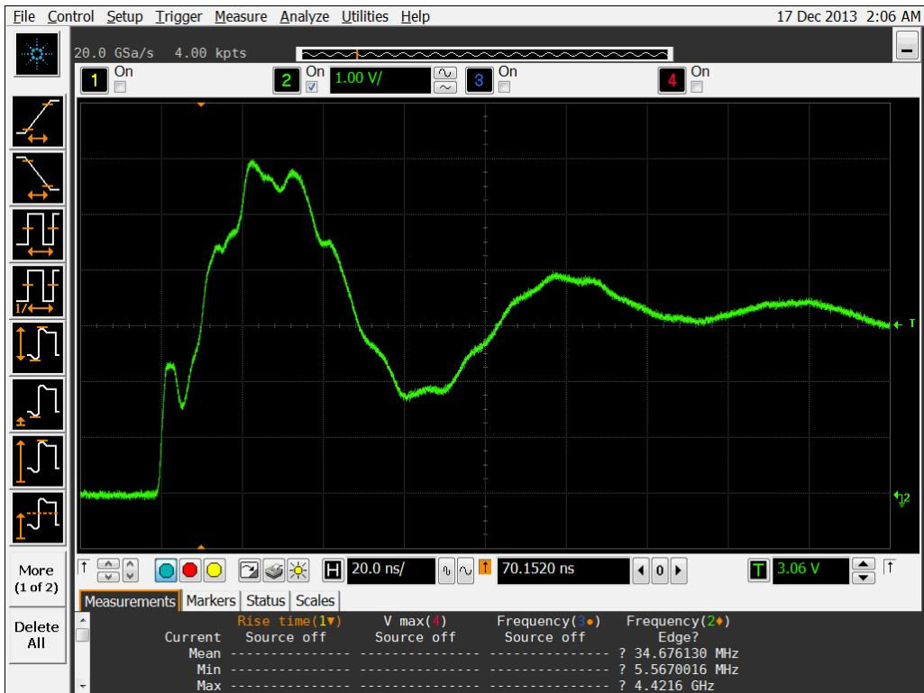
Figure 11a DUT 12311 Pre-Radiation Rising Edge
