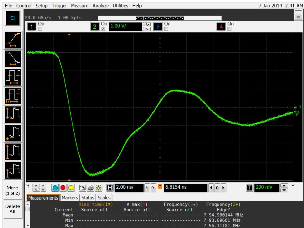
Figure 19b DUT 12324 Post-Annealing Falling Edge
