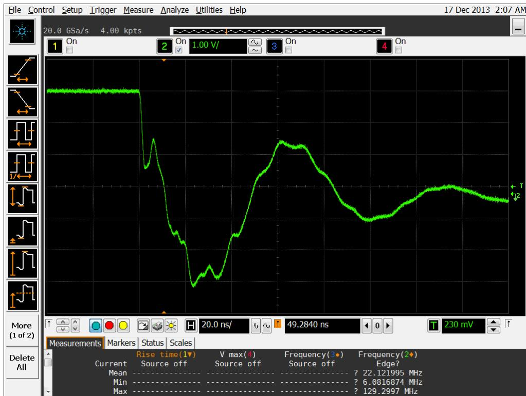
Figure 17a DUT 12311 Pre-Irradiation Falling Edge
