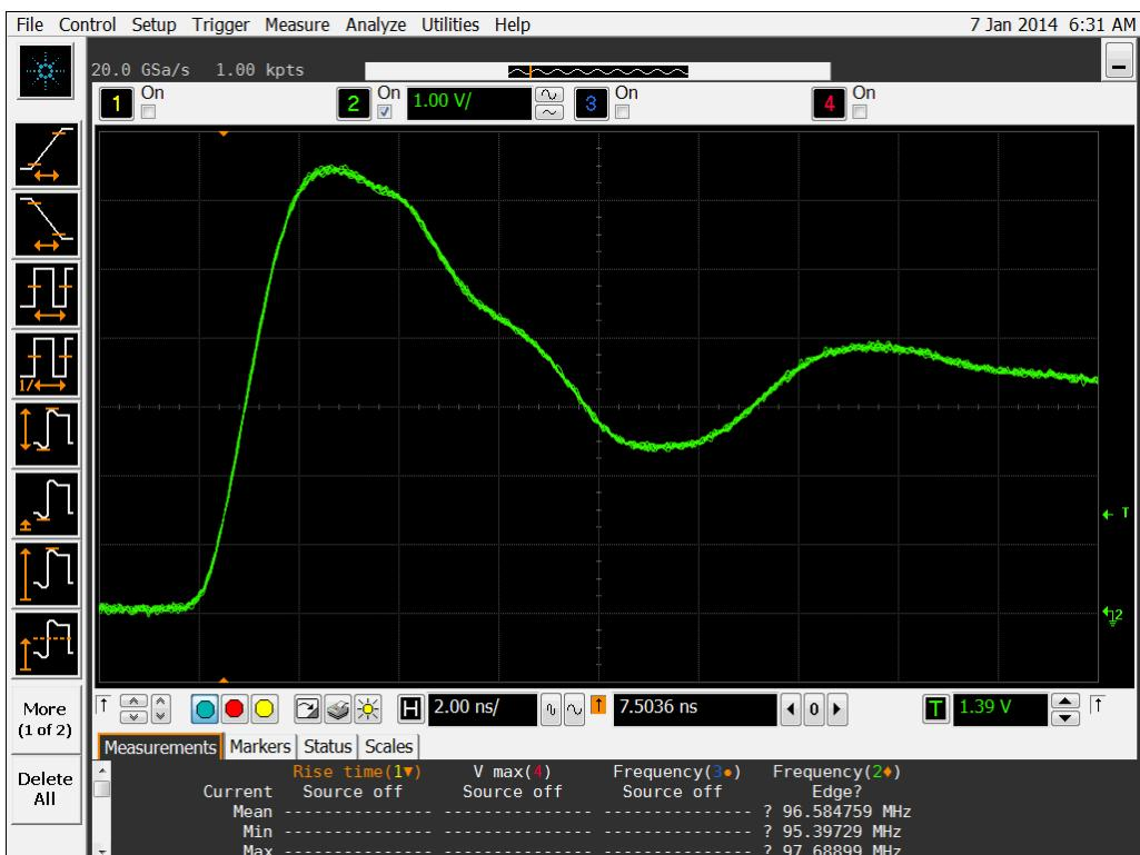
Figure 11b DUT 12311 Post-Annealing Rising Edge
