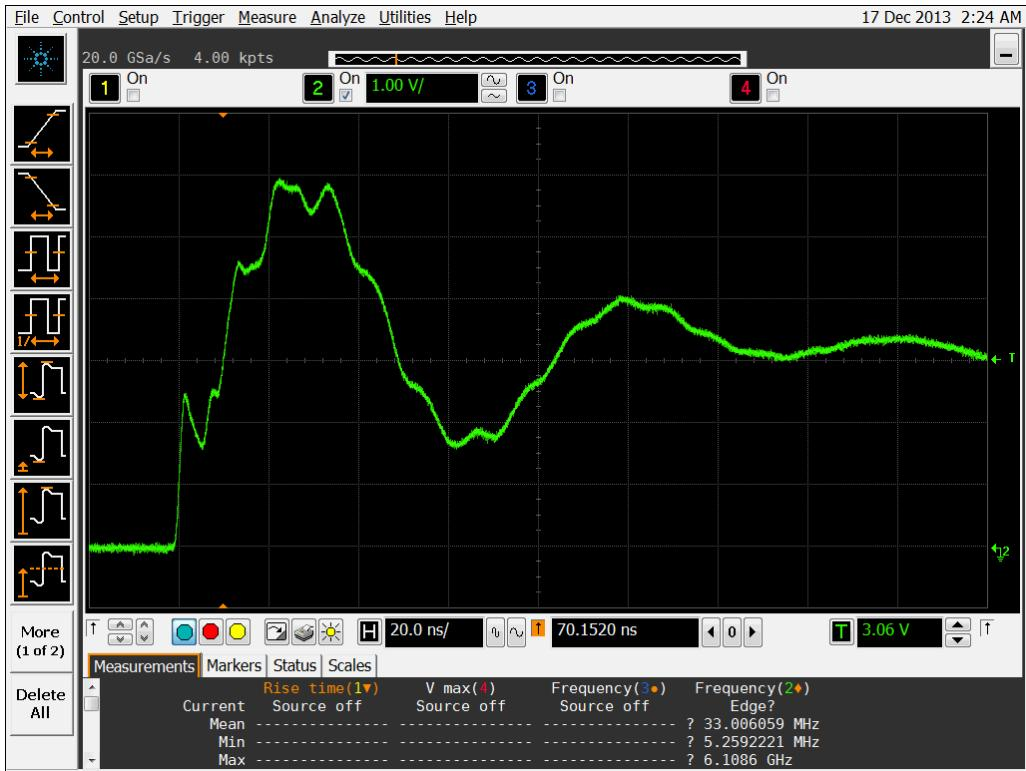
Figure 13a DUT 12324 Pre-Irradiation Rising Edge
