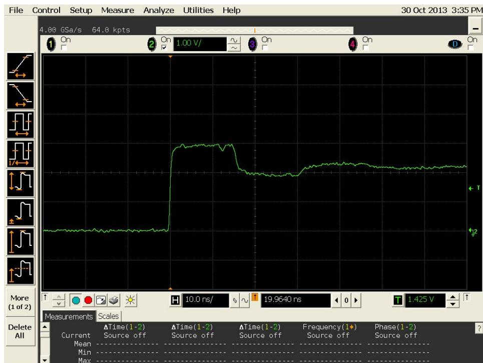
Figure 3a DUT 9485 Pre-Irradiation Rising Edge
