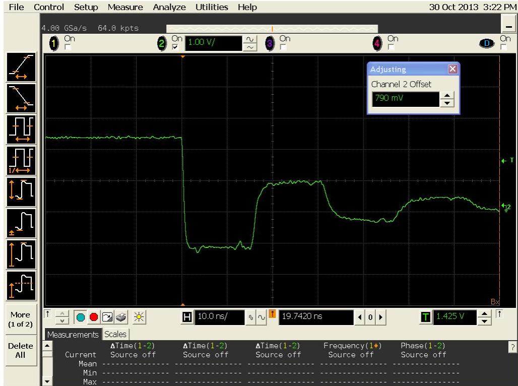
Figure 9a DUT 9525 Pre-Irradiation Falling Edge
