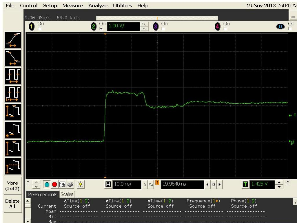
Figure 4b DUT 9499 Post-Annealing Rising Edge
