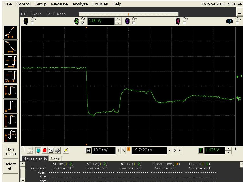
Figure 8b DUT 9499 Post-Annealing Falling Edge
