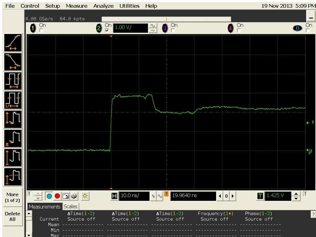
Figure 5b DUT 9525 Post-Annealing Rising Edge
