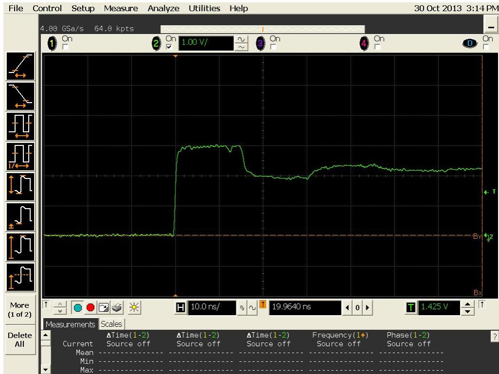
Figure 5a DUT 9525 Pre-Irradiation Rising Edge
