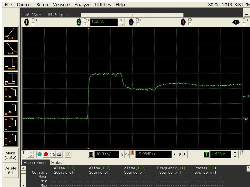
Figure 6a DUT 9526 Pre-Irradiation Rising Edge
