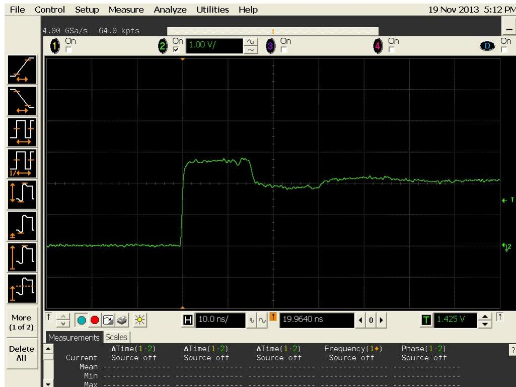
Figure 6b DUT 9526 Post-Annealing Rising Edge
