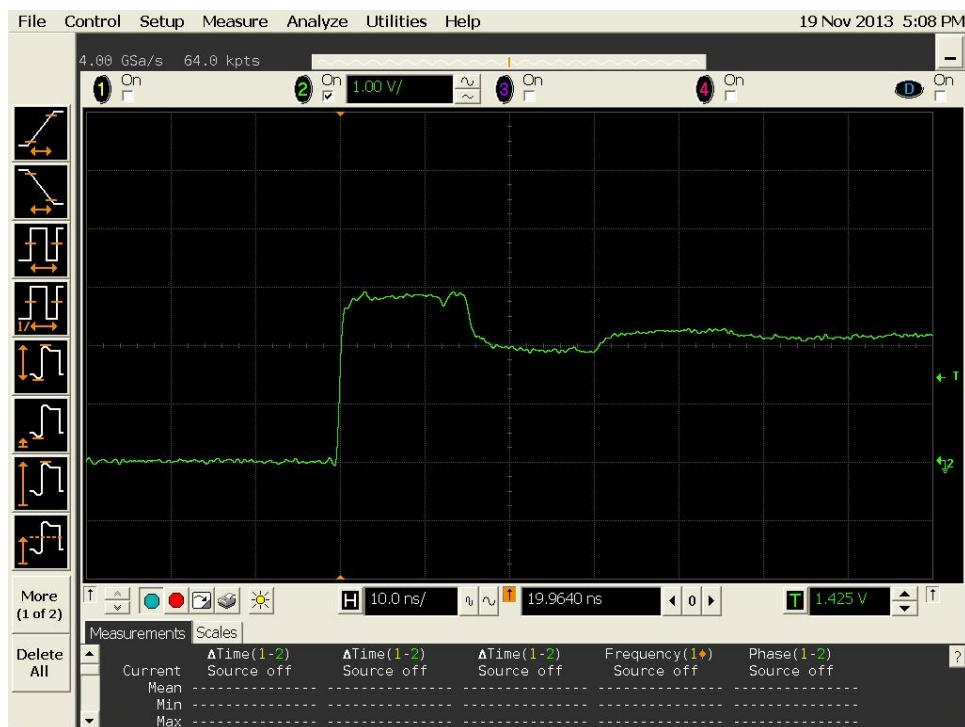
Figure 3b DUT 9485 Post-Annealing Rising Edge
