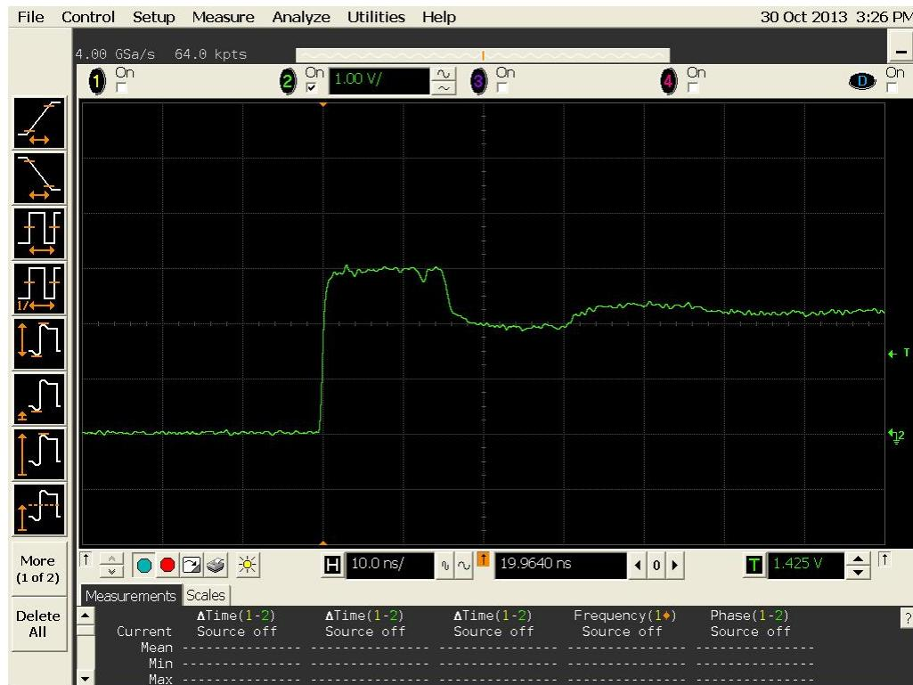
Figure 4a DUT 9499 Pre-Irradiation Rising Edge
