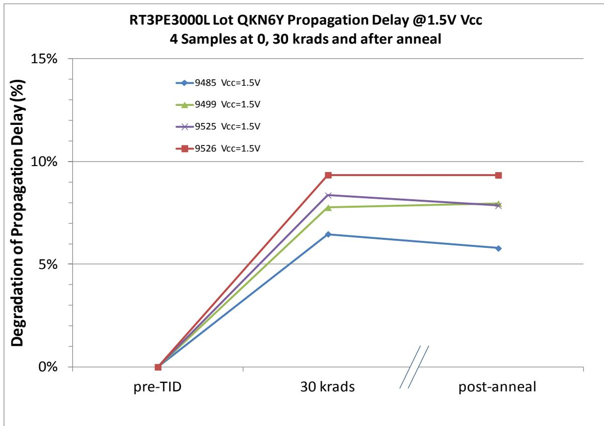
Figure 2 Degradation of Propagation Delay versus TID and Annealing
