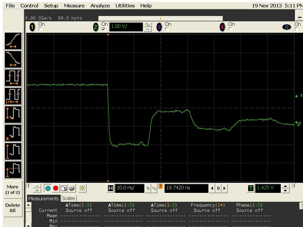
Figure 10b DUT 9526 Post-Annealing Falling Edge
