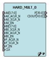
Figure 3-1 • Hard Multiplier Ports, Normal Mode
