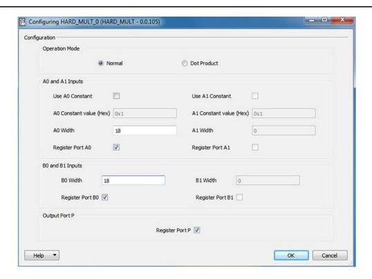
Figure 1-1 • Hard Multiplier Configuration Options - Normal Mode
