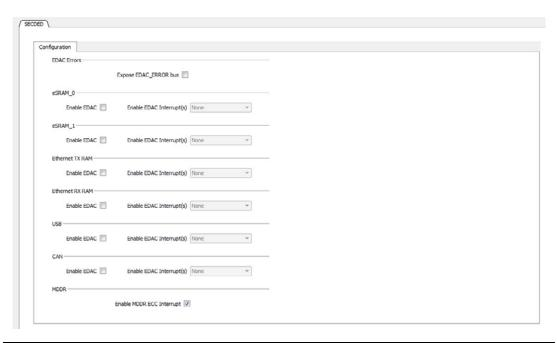
Figure 1-2 • MSS SECDED Configurator
