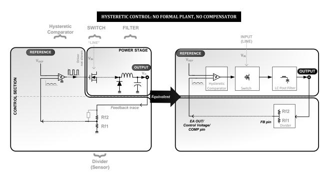
Figure 10: Functional Blocks of the Hysteretic Converter
