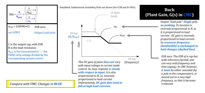
Figure 6: Plant Transfer Function for a Buck, Using CMC
