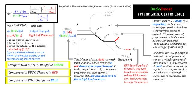
Figure 8: Plant Transfer Function for a Buck-Boost, Using CMC
