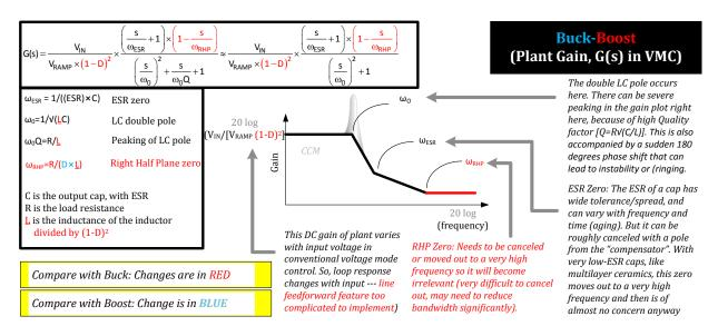
Figure 5: Plant Transfer Function for a Buck-Boost, Using VMC
