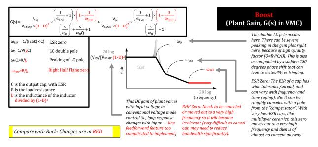
Figure 4: Plant Transfer Function for a Boost, Using VMC
