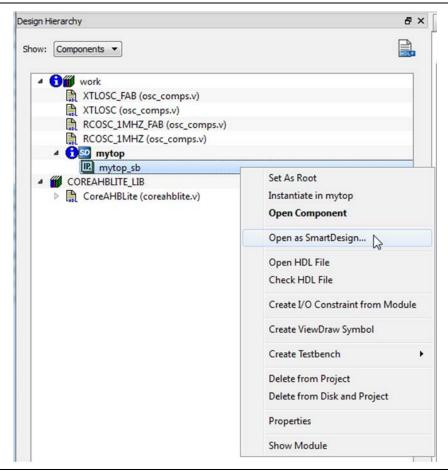
Figure 3 System Builder Component in the Design Hierarchy Window
