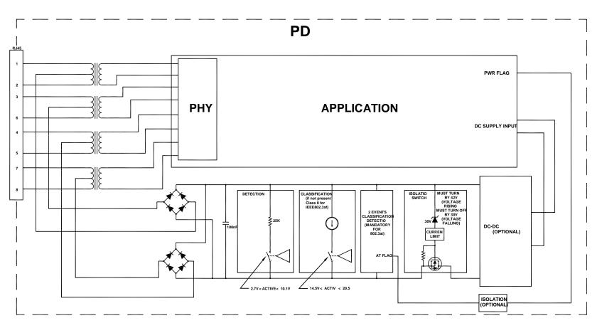
Figure 4: Basic PD Block Diagram
