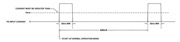
Figure 3: PoE Maintain Power Signature (MPS) Requirements
