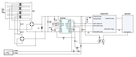
Figure 7: External Power Input connected to PD70210A Output
