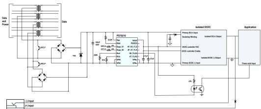
Figure 8: External Power Input connected to Application supply Rails – Switched Connection
