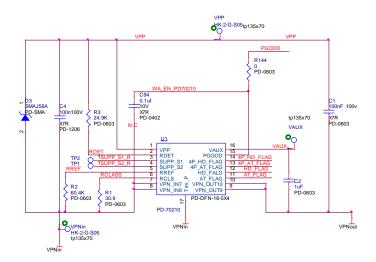
Figure 10: HDBASET Type 3 front end- PD device (2 of 2)
