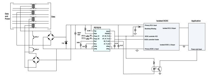
Figure 5: Typical 2 or 4 Pair Configuration with a Single PD70210 IC
