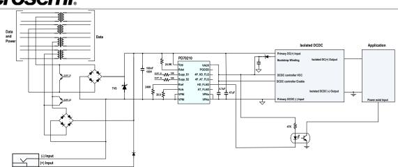
Figure 6: External Power Input connected to PD70210 Input
