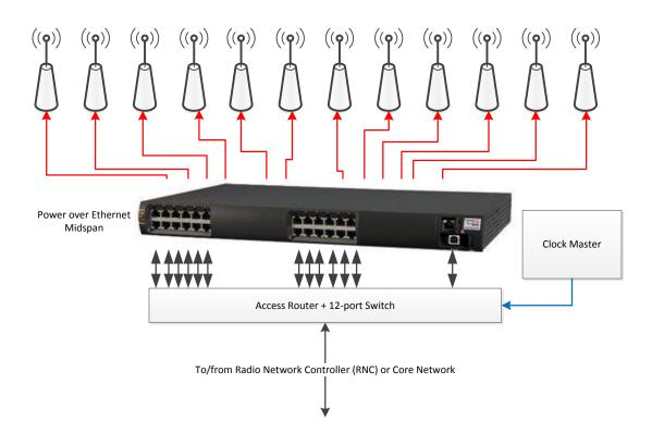
Figure 1 Small Cell Cluster Deployment with PoE
