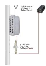
Figure 3 Indoor to Outdoor Small Cell/Wi-Fi Hotspot Deployment
