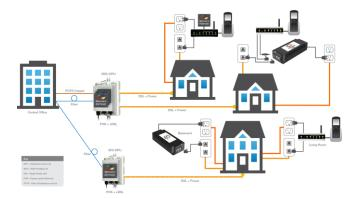
Figure 6 Reverse Power Feeding for Fiber to the Distribution Point
