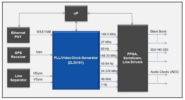
Block diagram of a Master Sync Generator is shown in Figure 2.
