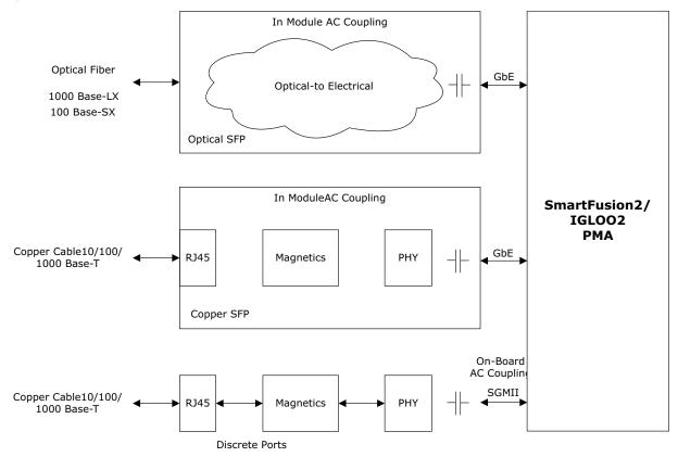
RJ45 connectors are used for copper cable physical transport layer, or 1000BASE-T. This interface requires a PHY device to inter-operate and to re-time the interface.
