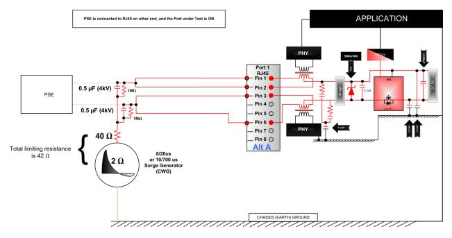
capacitance of it *will fall across the line* during a surge, and will absorb the surge energy, protecting the PD in the bargain, which is effectively just in parallel with the PSE.
