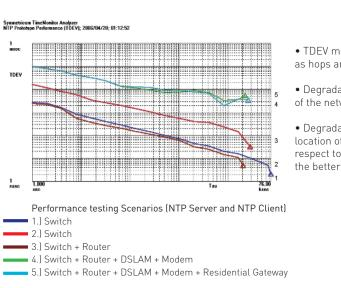
FIG 1 The effect of network jitter on NTP accuracy
