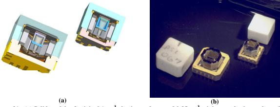
Figure 21: (a) Solid models of original 1 cm<sup>3</sup> physics package and 0.35 cm<sup>3</sup> miniature physics package (b) photos of same
