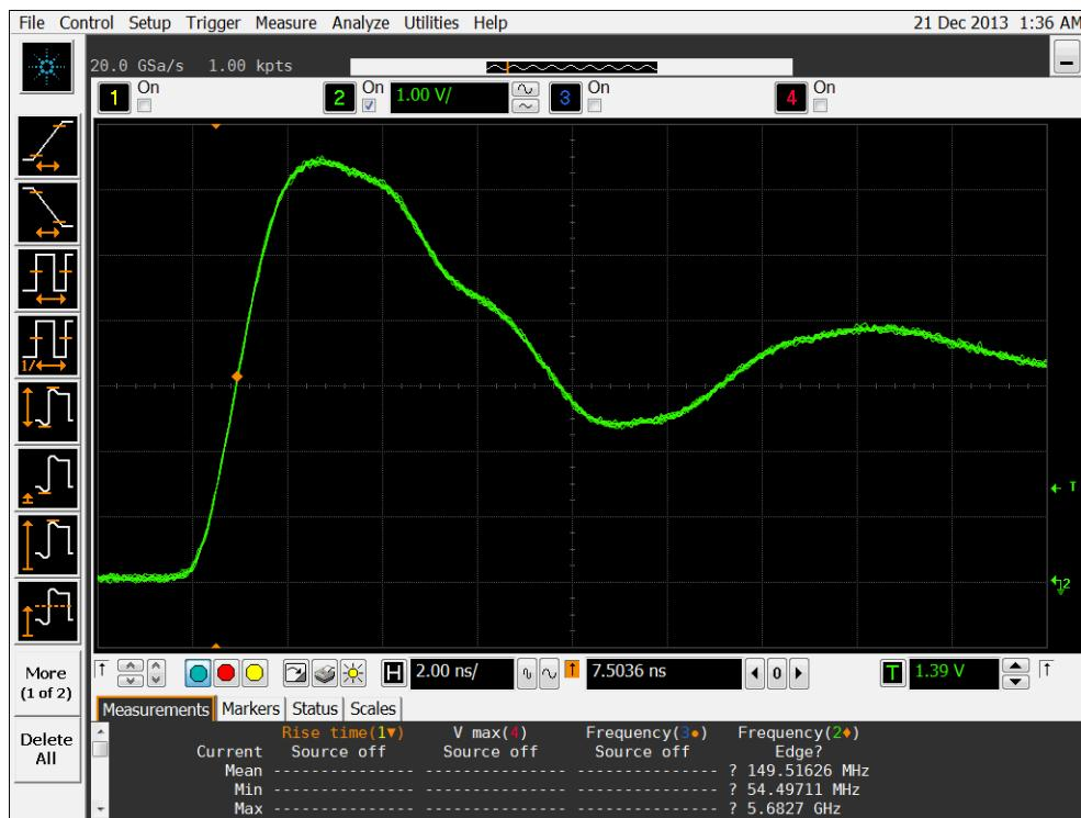
Figure 9b DUT 6121 Post-Annealing Rising Edge
