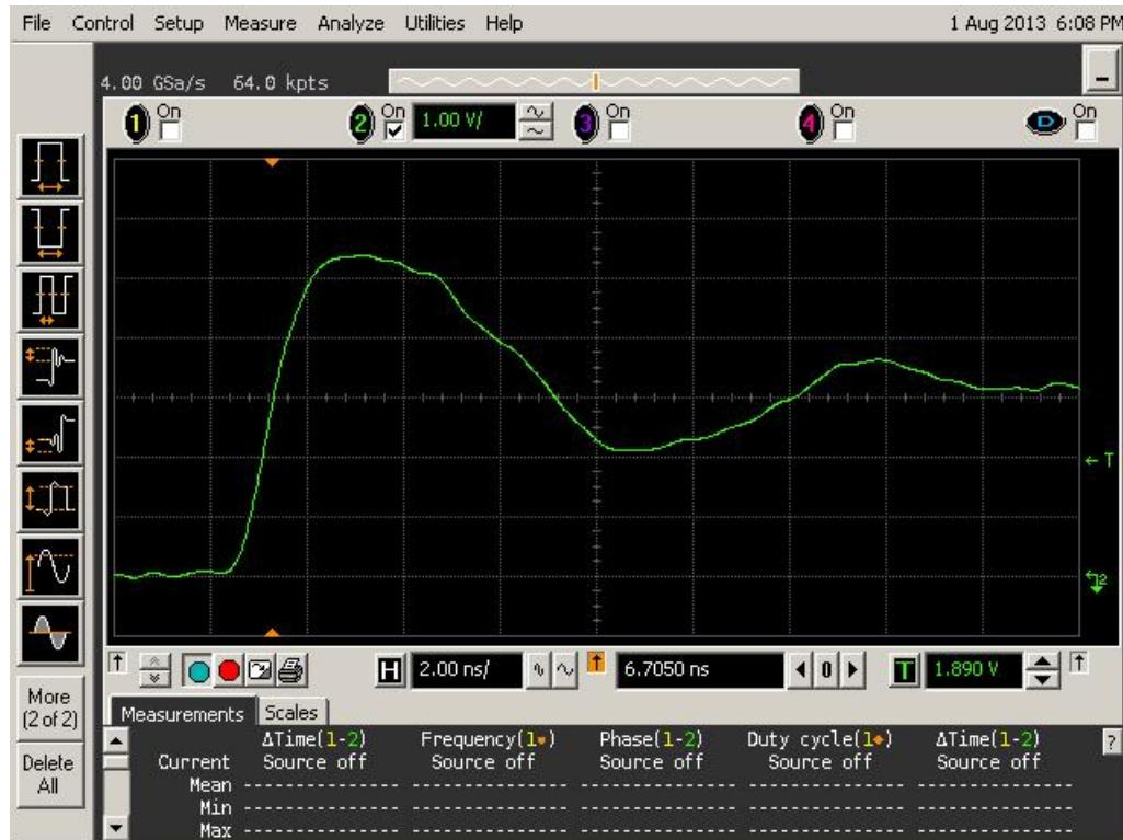
Figure 14a DUT 6120 Pre-Irradiation Rising Edge
