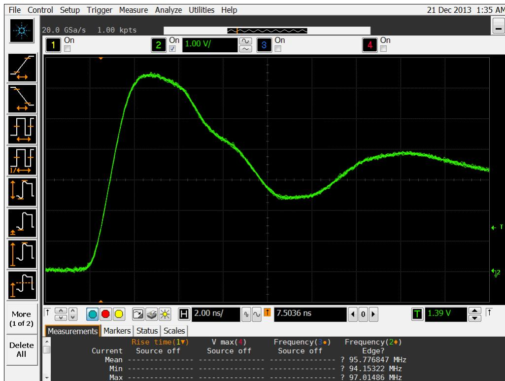
Figure 14b DUT 6120 Post-Annealing Rising Edge
