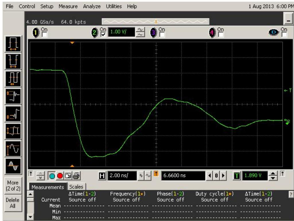
Figure 18a DUT 6107 Pre-Irradiation Falling Edge
