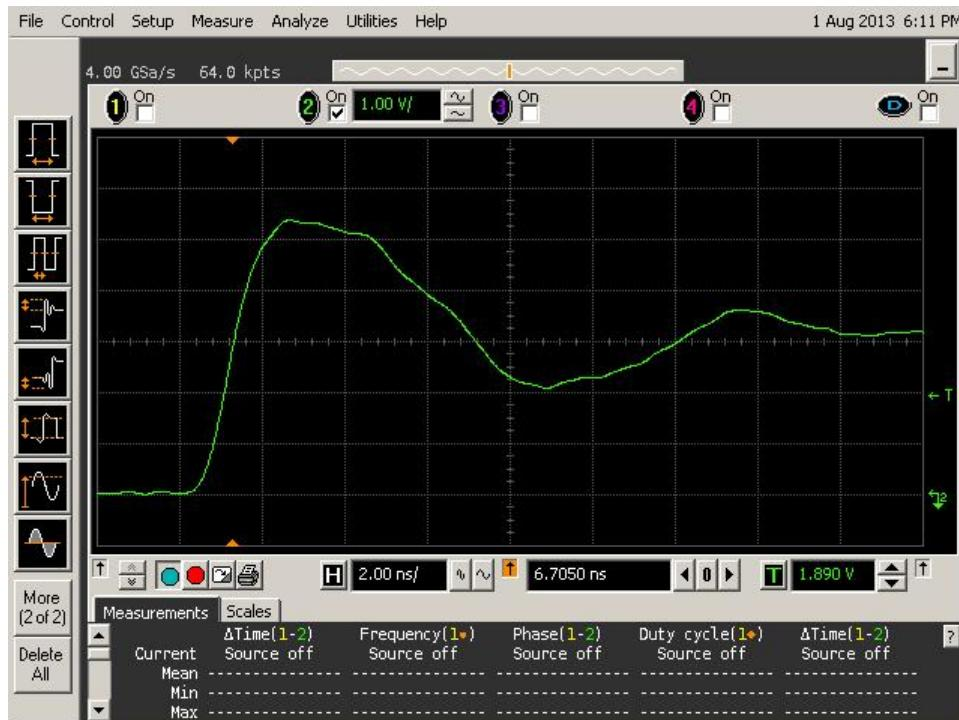
Figure 9a DUT 6121 Pre-Irradiation Rising Edge
