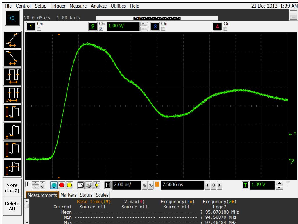
Figure 11b DUT 6152 Post-Annealing Rising edge
