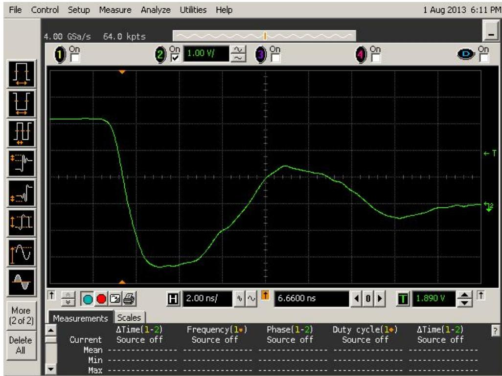
Figure 15a DUT 6121 Pre-Radiation Falling Edge
