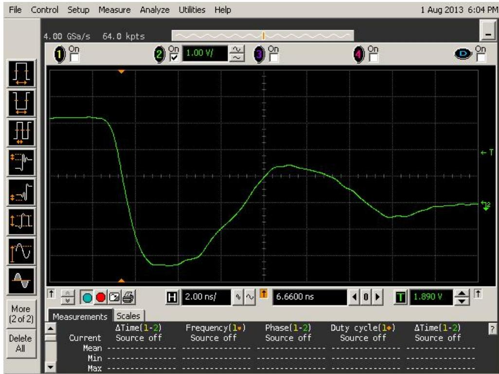
Figure 19a DUT 6119 Pre-Irradiation Falling Edge
