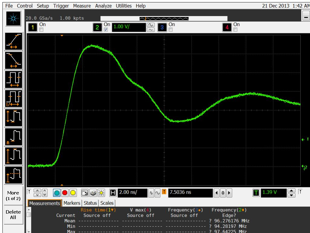
Figure 10b DUT 6122 Post-Annealing Rising Edge
