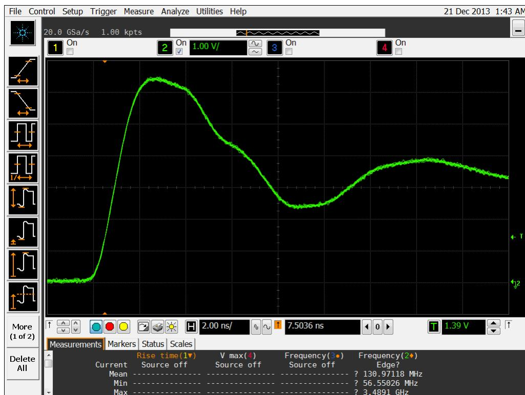
Figure 12b DUT 6107 Post-Annealing Rising Edge
