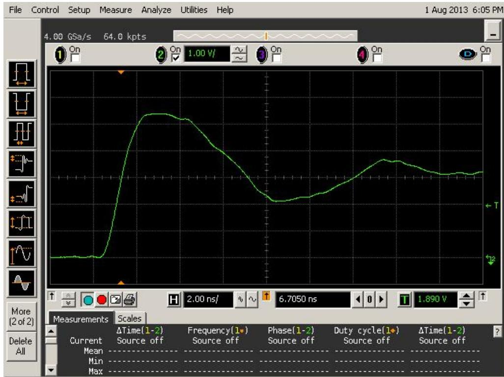
Figure 13a DUT 6119 Pre-Irradiation Rising Edge
