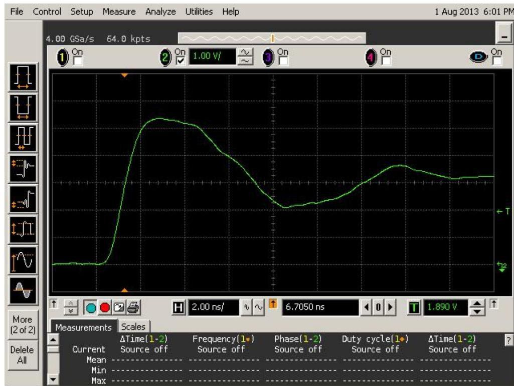
Figure 12a DUT 6107 Pre-Irradiation Rising Edge
