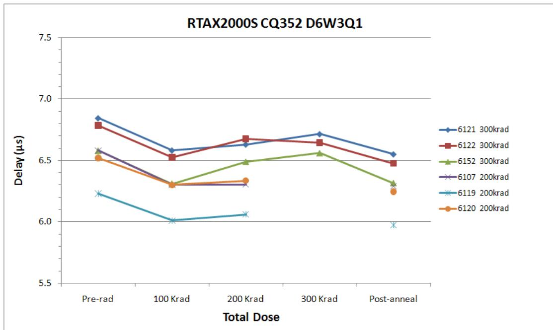
**Figure 8 In-Situ Propagation Delay versus Total Dose.**
