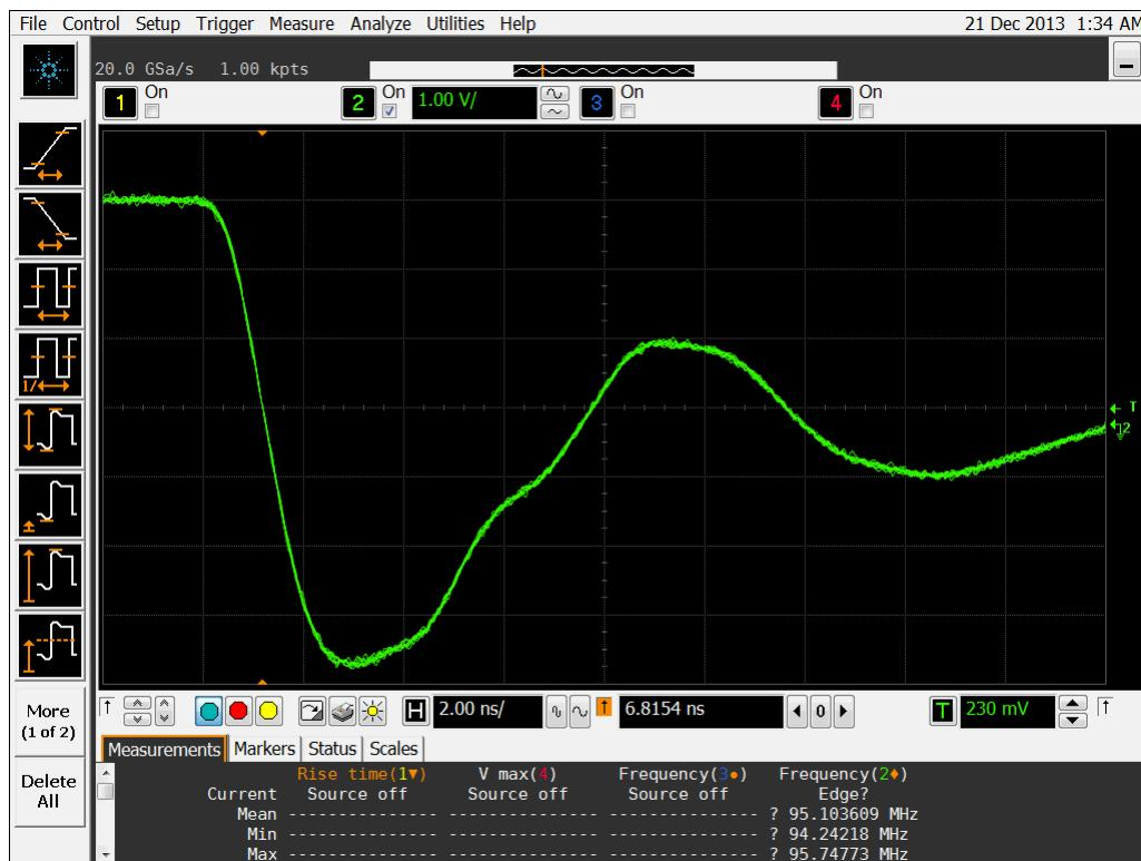
Figure 20b DUT 6120 Post-Annealing Falling Edge
