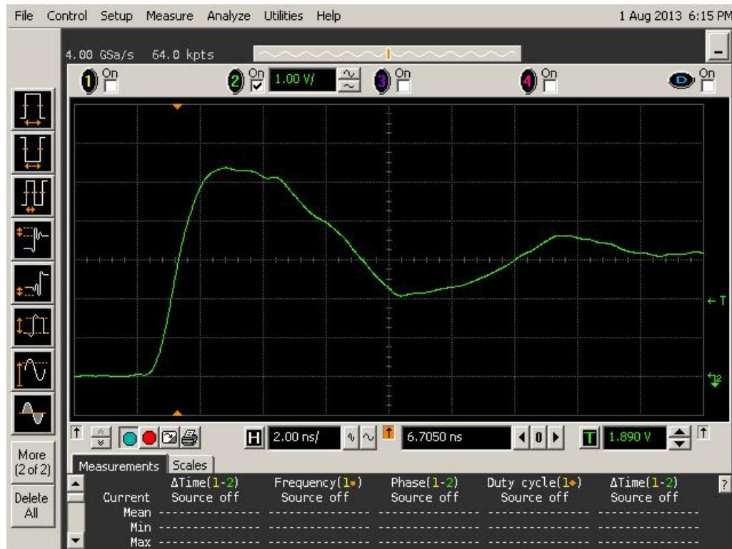
Figure 10a DUT 6122 Pre-Irradiation Rising Edge
