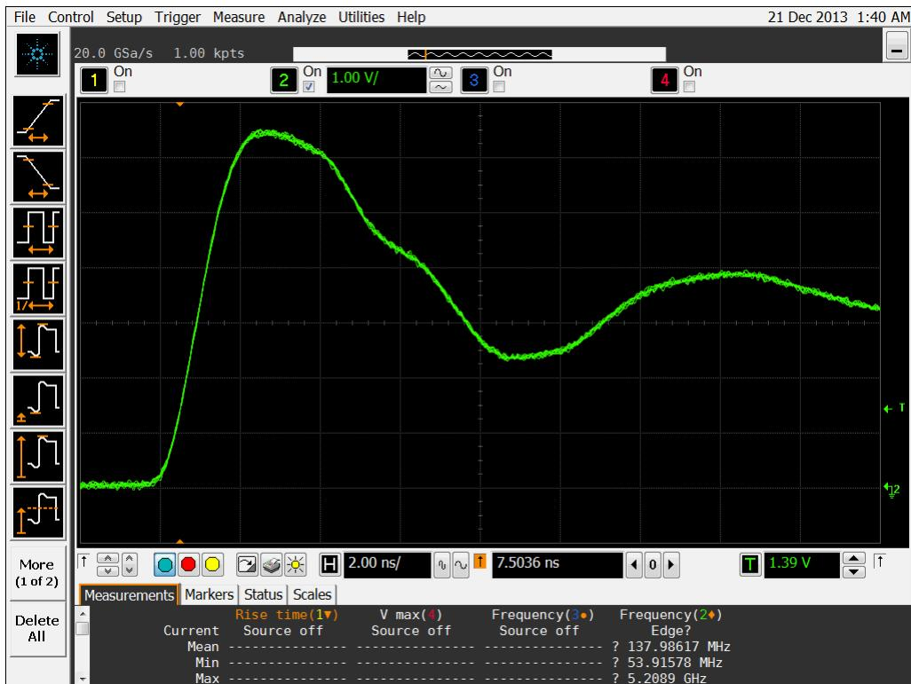
Figure 13b DUT 6119 Post-Annealing Rising Edge
