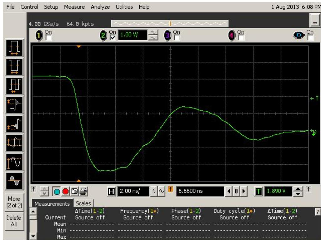
Figure 20a DUT 6120 Pre-Irradiation Falling Edge
