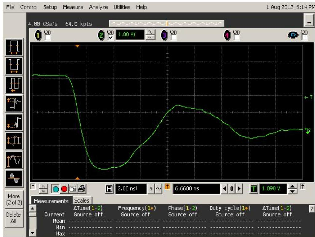
Figure 16a DUT 6122 Pre-Irradiation Falling Edge
