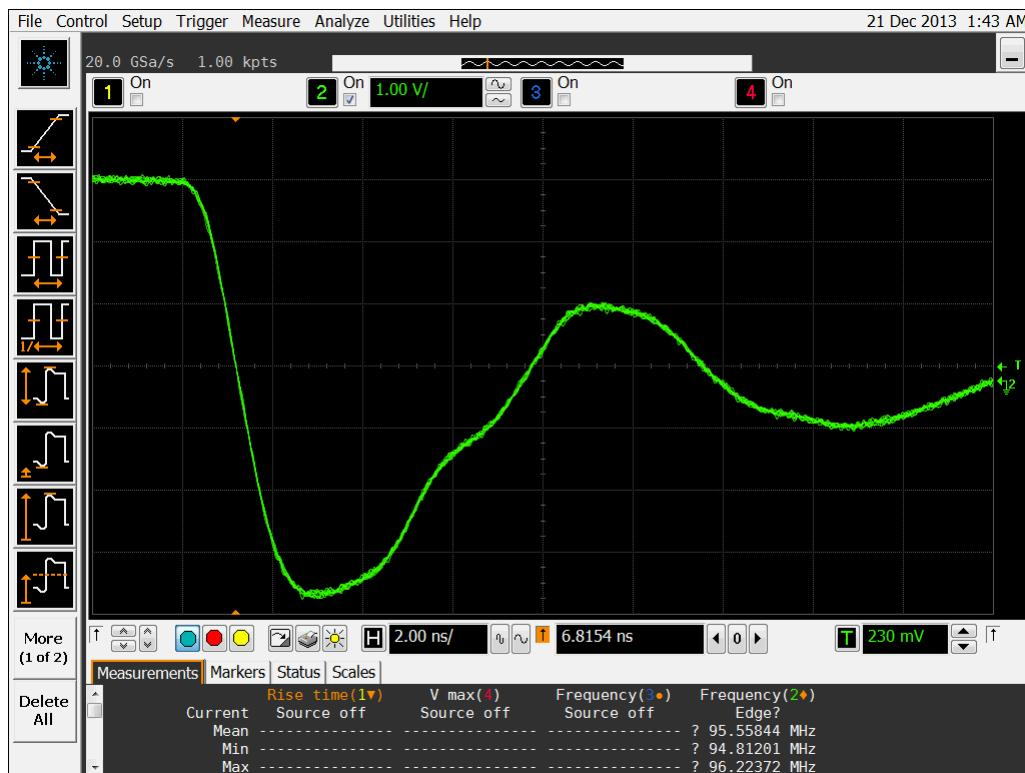
Figure 18b DUT 6107 Post-Annealing Falling Edge
