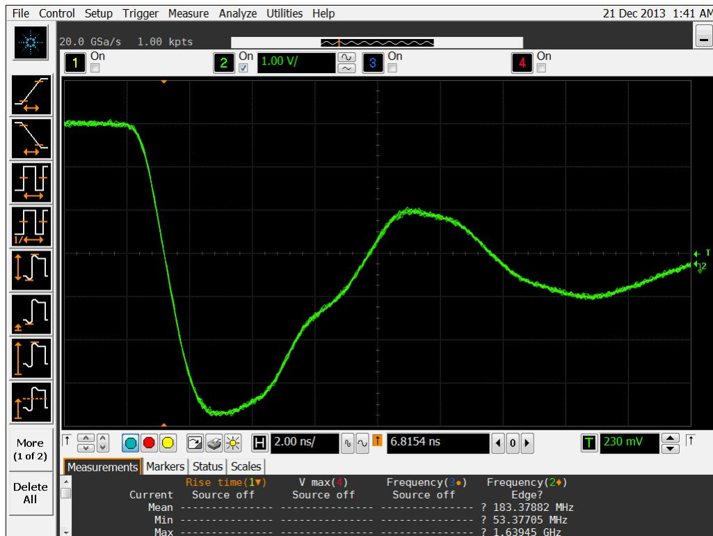
Figure 16b DUT 6122 Post-Annealing Falling Edge
