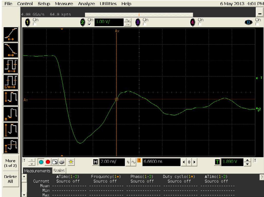
Figure 19a DUT 3429 Pre-Irradiation Falling Edge.
