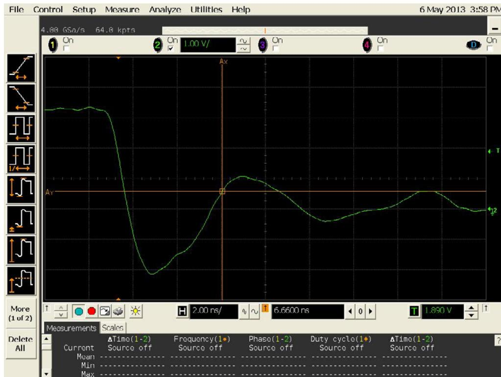
Figure 18a DUT 3421 Pre-Irradiation Falling Edge.
