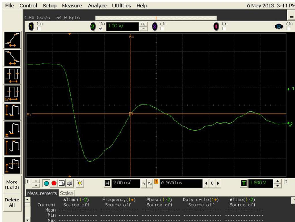
Figure 14a DUT 3401 Pre-Irradiation Falling Edge.
