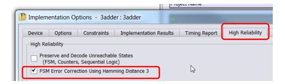
With Hamming-3 error correction, comparator circuits and parity flip-flops are automatically added during synthesis
