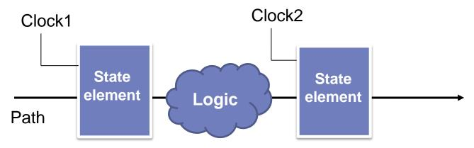
Clock1 and Clock2 are in different clock domains and are assumed synchronous by default unless you use the -asynchronous option
