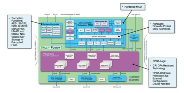
Figure 1: SmartFusion2 Architecture Block Diagram
