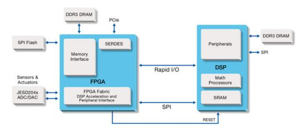
Figure 3: Industrial Sensor Controller Using an FPGA and a DSP
