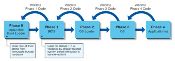
Figure 2: Multi-Stage Secure Boot Process Overview
