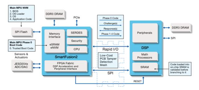
Figure 4: Secure Embedded Industrial Sensor Controller
