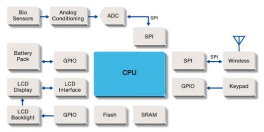
Figure 1: Example of Personal Health Monitor – Block Diagram
