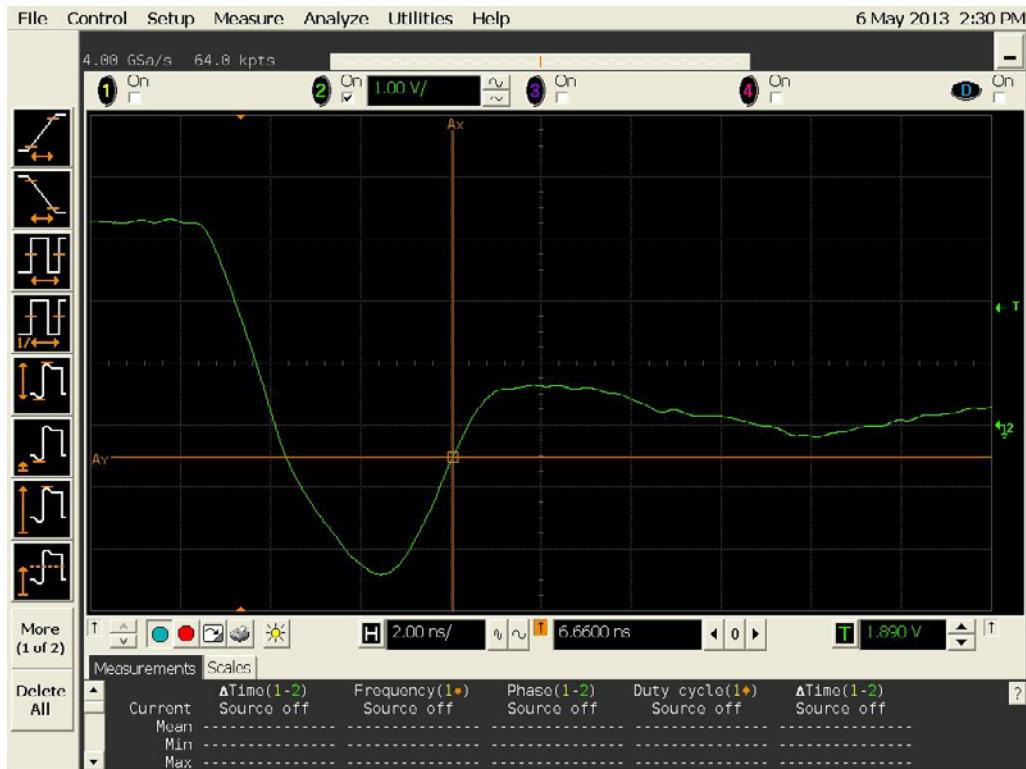
Figure 18a DUT 4391 Pre-Irradiation Falling Edge
