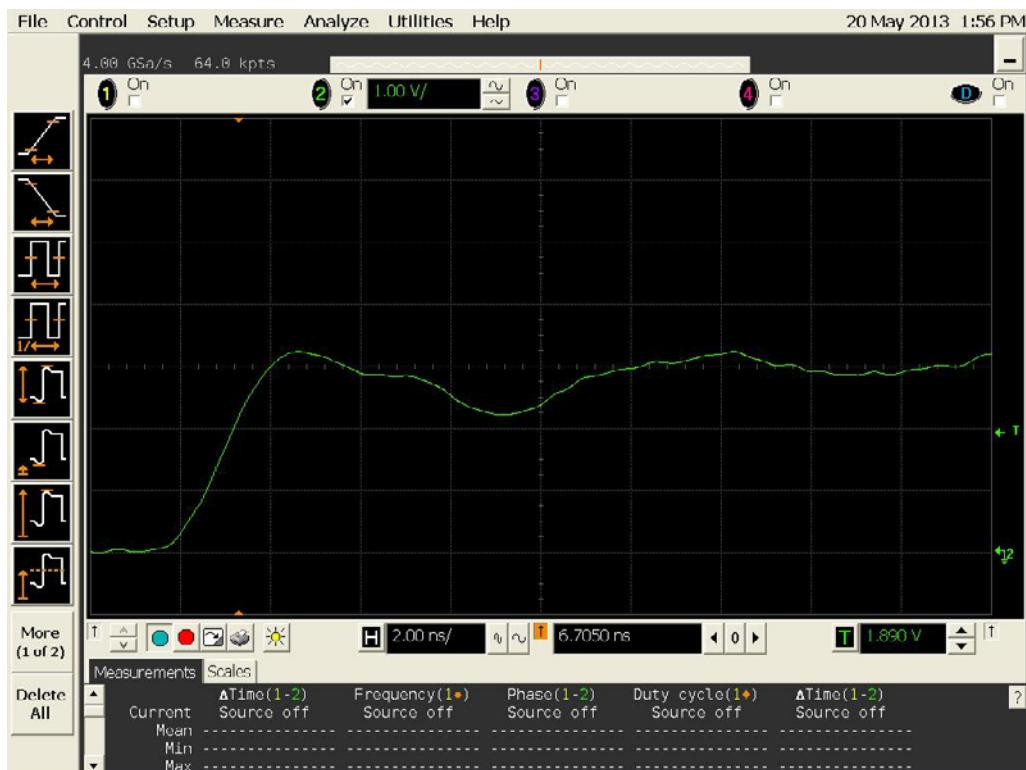
Figure 12b DUT 4391 Post-Annealing Rising Edge
