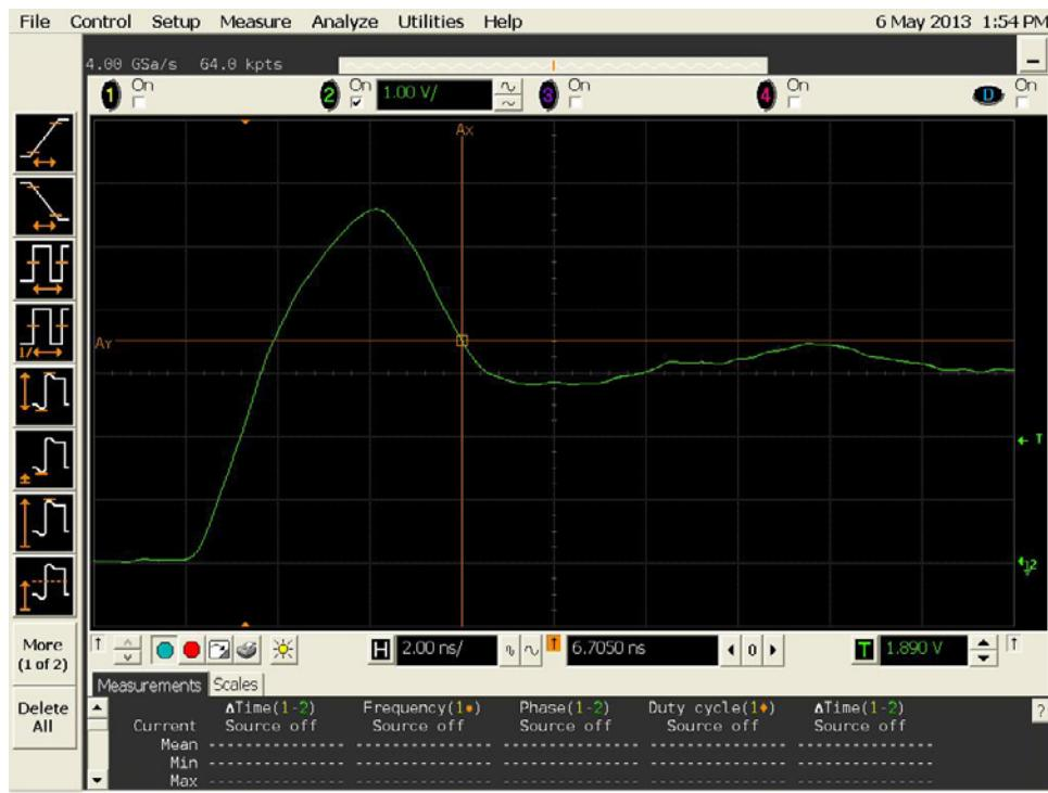
Figure 9a DUT 4360 Pre-Irradiation Rising Edge
