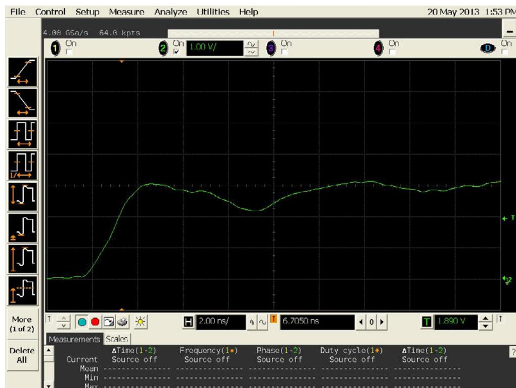
Figure 11b DUT 4390 Post-Annealing Rising edge
