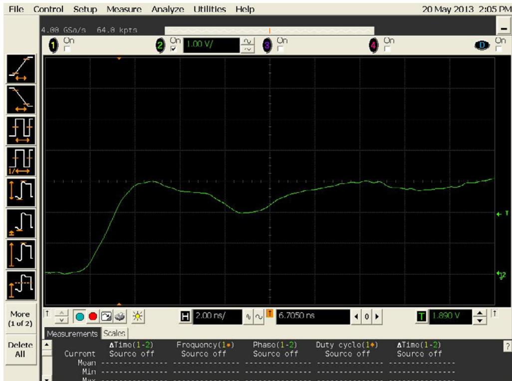
Figure 14b DUT 4412 Post-Annealing Rising Edge
