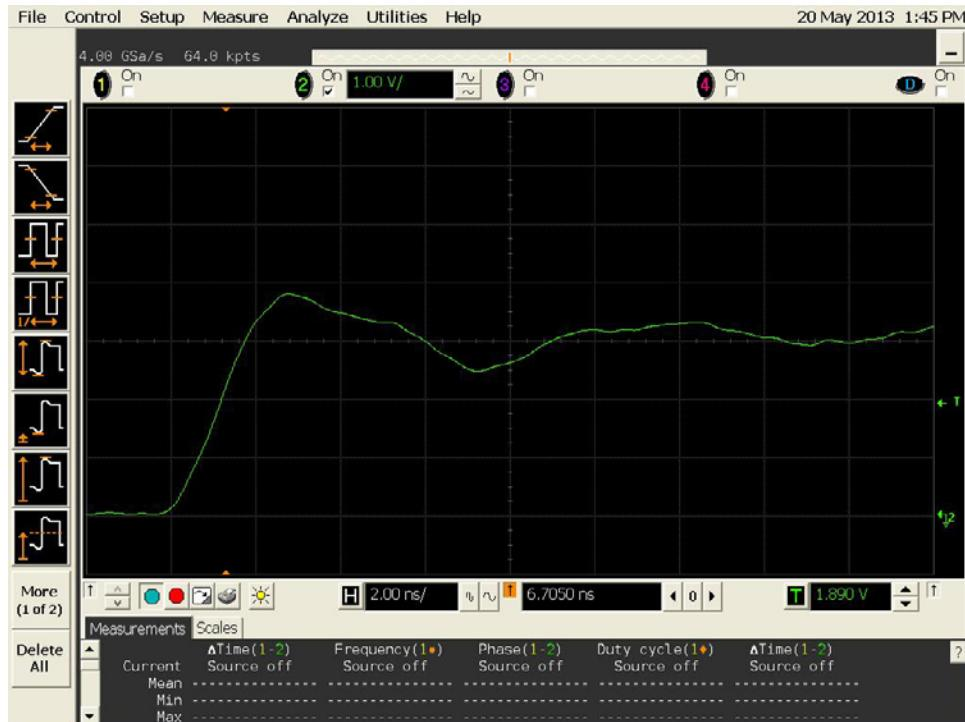
Figure 9b DUT 4360 Post-Annealing Rising Edge
