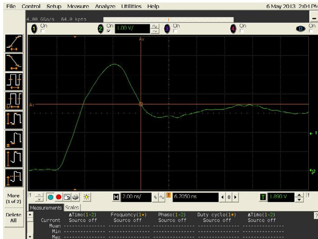
Figure 11a DUT 4390 Pre-Radiation Rising Edge
