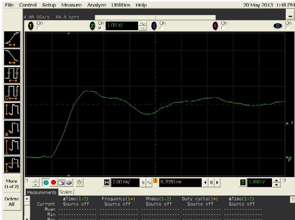
Figure 10b DUT 4381 Post-Annealing Rising Edge
