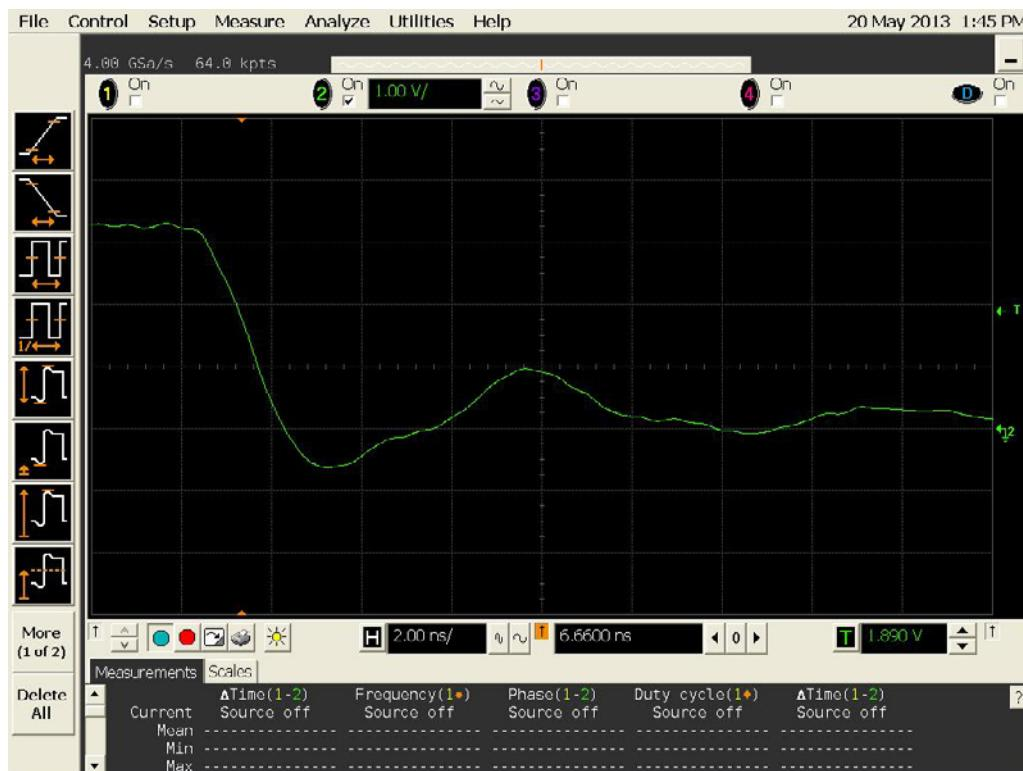
Figure 15b DUT 4360 Post-Annealing Falling Edge
