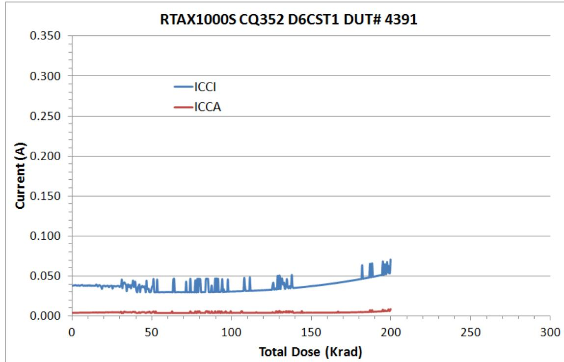
Figure 5 DUT 4391 Influx ICCA and ICCI (more measurement noises are seen on this run)
