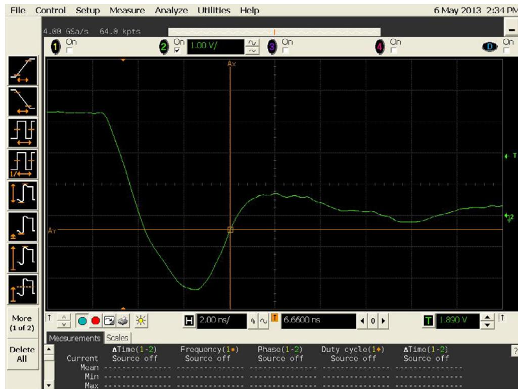
Figure 19a DUT 4395 Pre-Irradiation Falling Edge
