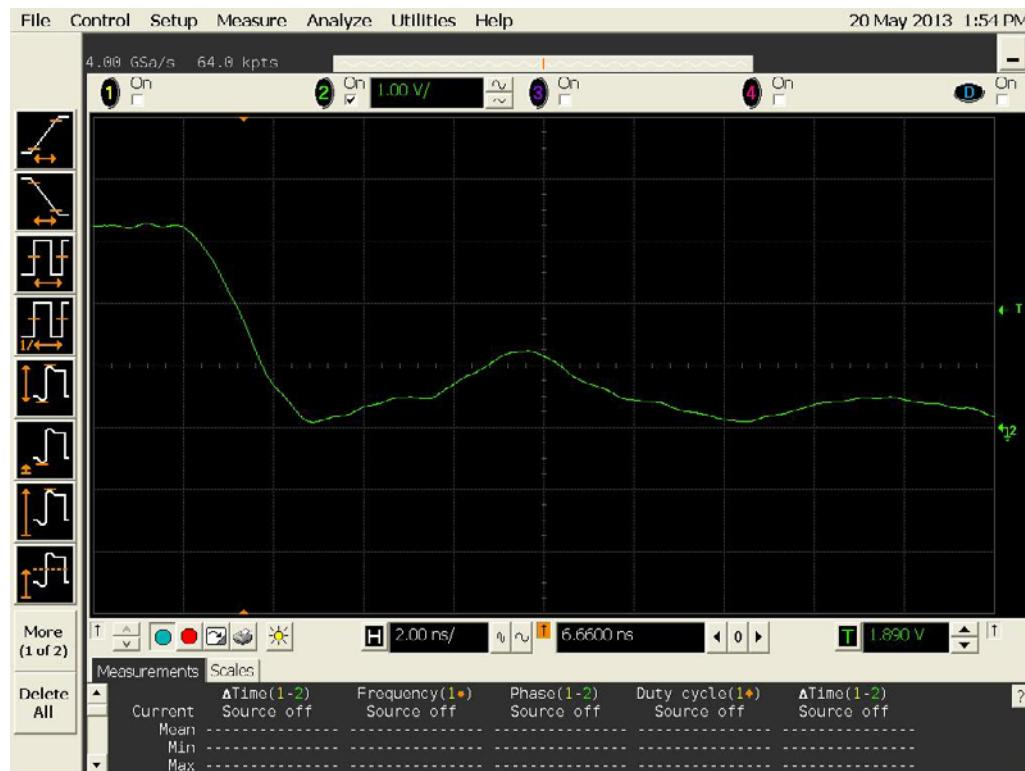
Figure 17b DUT 4390 Post-Annealing Falling Edge
