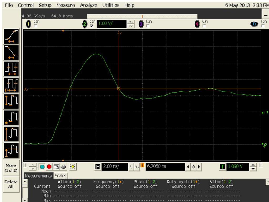
Figure 13a DUT 4395 Pre-Irradiation Rising Edge
