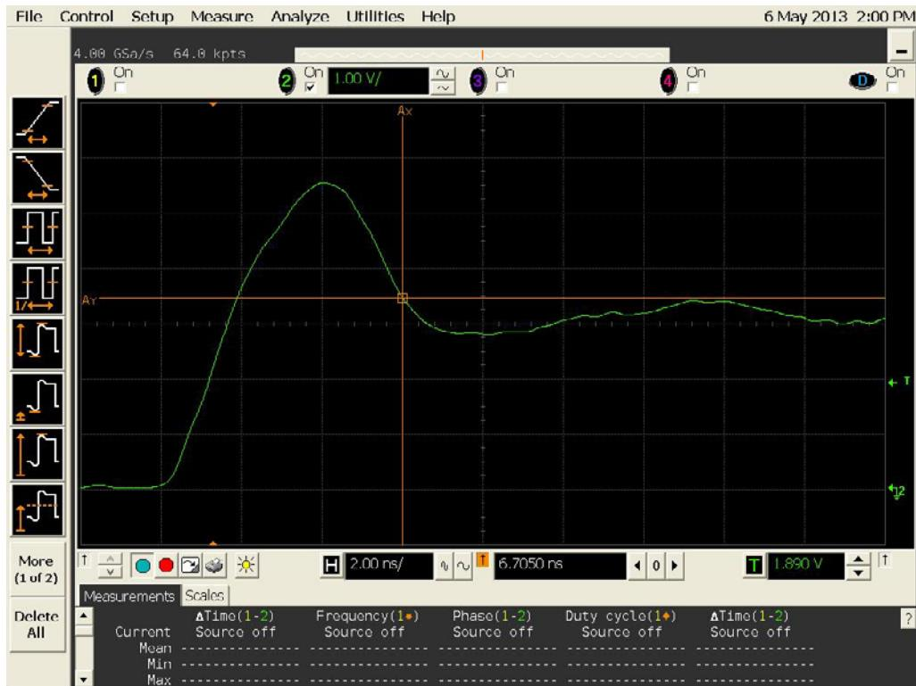
Figure 10a DUT 4381 Pre-Irradiation Rising Edge
