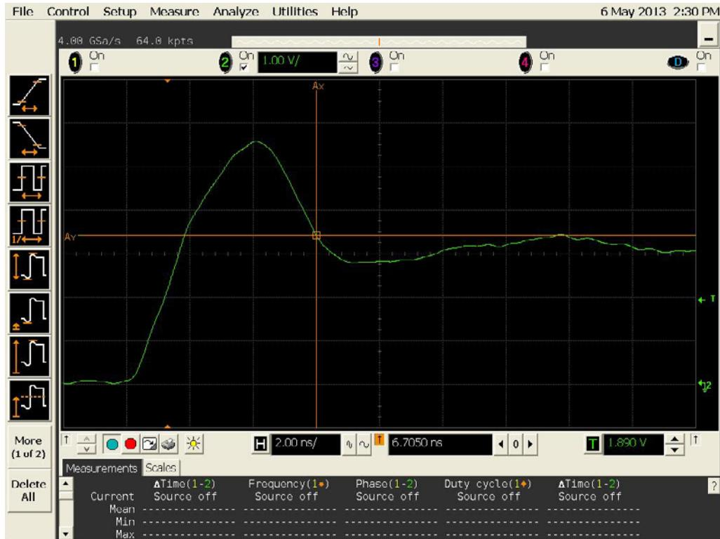
Figure 12a DUT 4391 Pre-Irradiation Rising Edge
