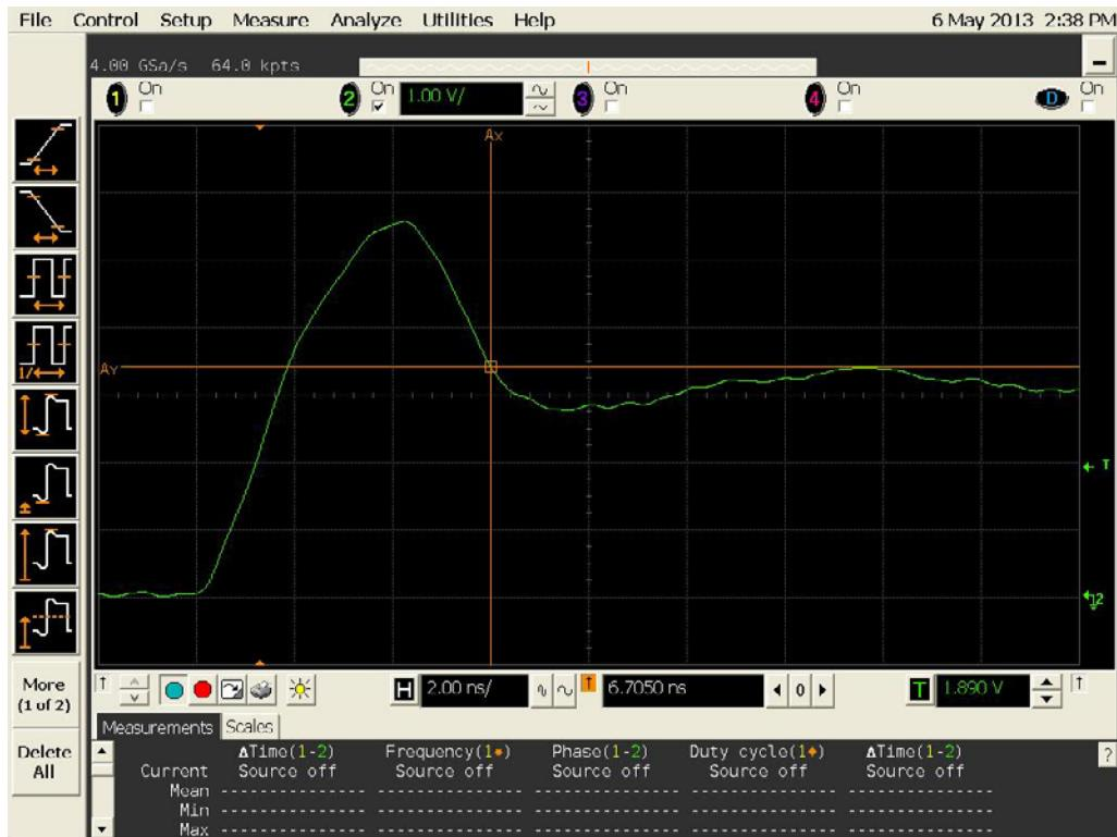
Figure 14a DUT 4412 Pre-Irradiation Rising Edge
