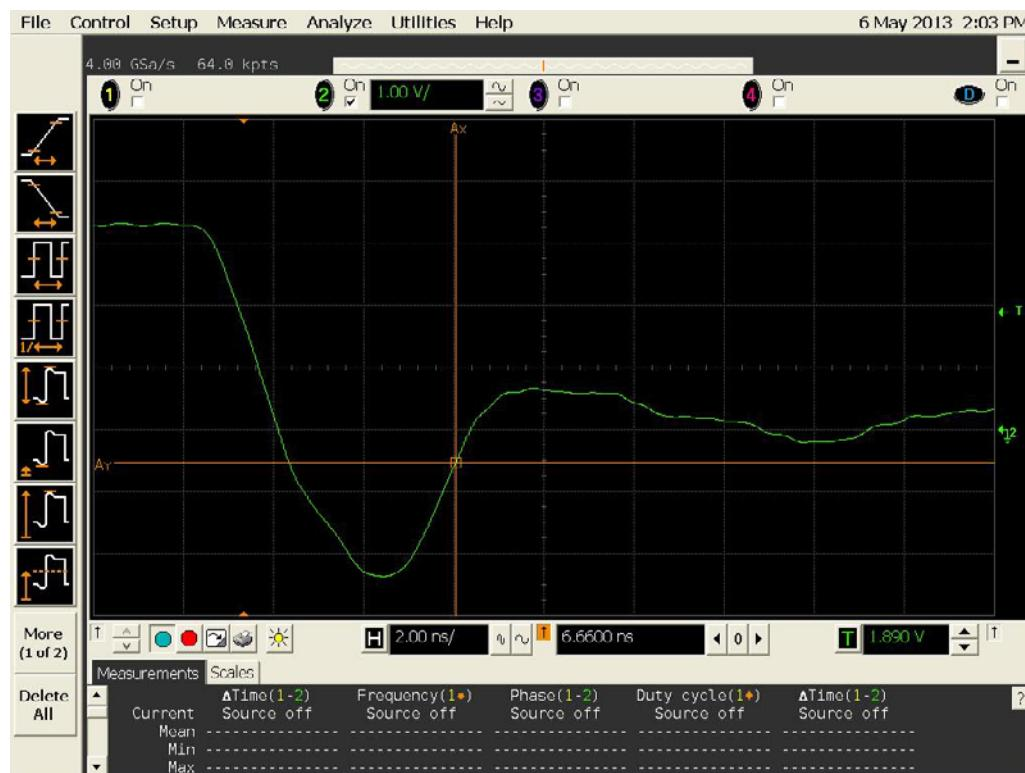
Figure 17a DUT 4390 Pre-Irradiation Falling Edge
