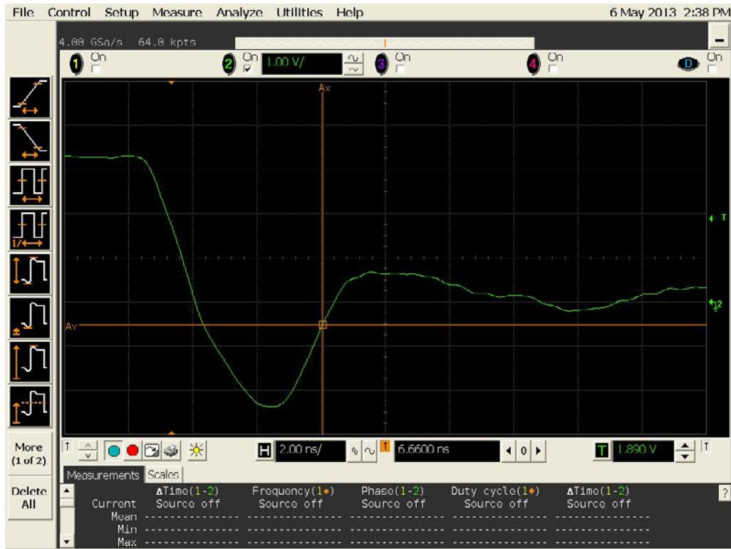
Figure 20a DUT 4412 Pre-Irradiation Falling Edge
